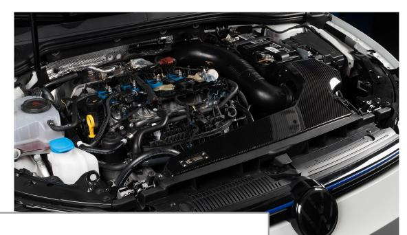
Lower your carbon lid into place and get it oriented properly where the fastener holes align.
