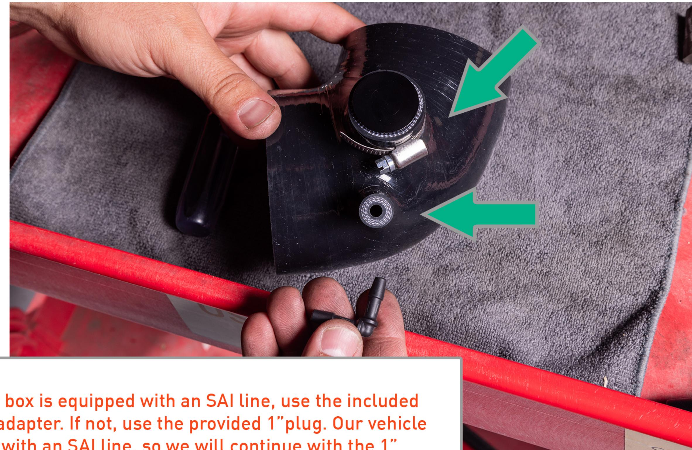
If your stock air box is equipped with an SAI line, use the included billet SAI filter adapter. If not, use the provided 1"plug. Our vehicle is not equipped with an SAI line, so we will continue with the 1" plug.
