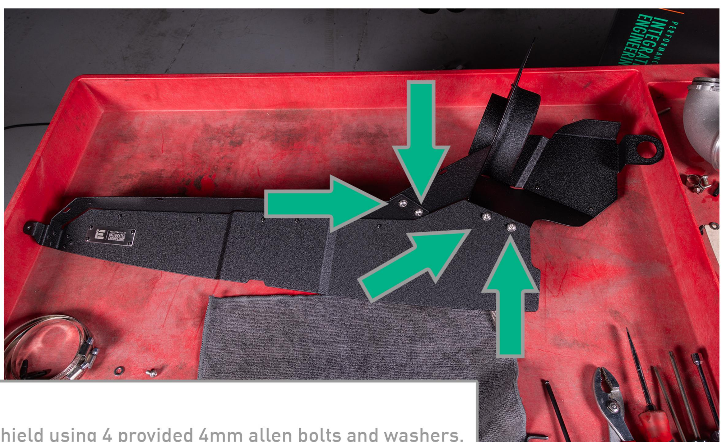
Assembly heat shield using 4 provided 4mm allen bolts and washers. Leave bolts finger tight until installing intake lid.
