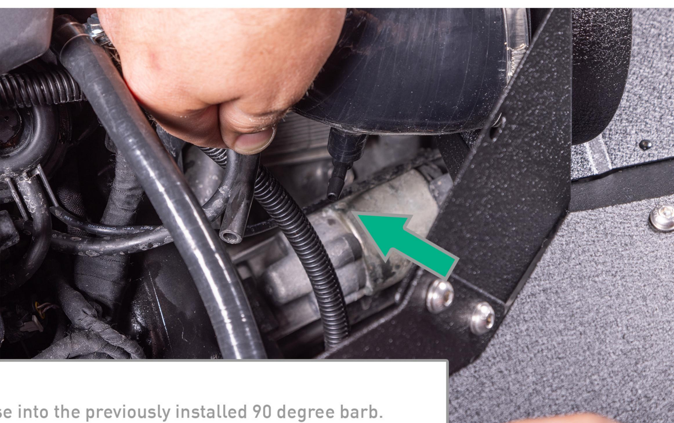
Plug vacuum hose into the previously installed 90 degree barb.
