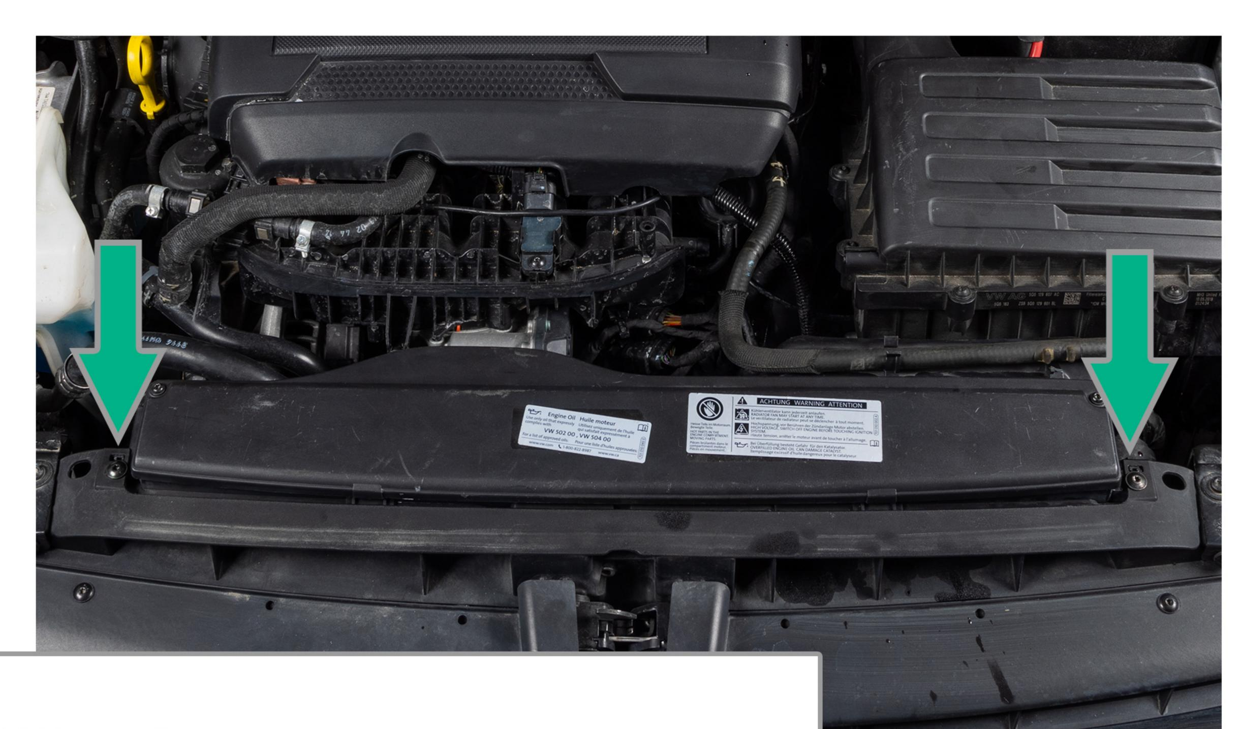
Remove two T20 Torx radiator mount screws.
