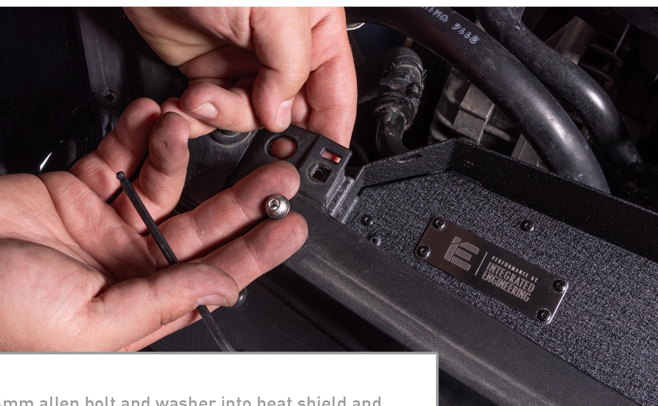
Install provided 4mm allen bolt and washer into heat shield and radiator support.
