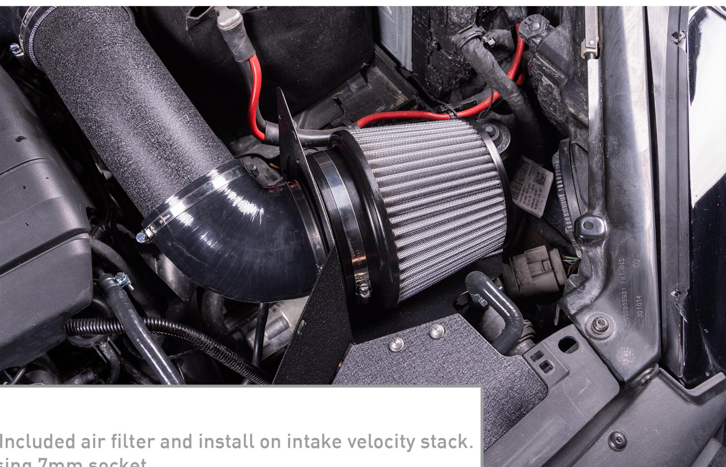
install clamp on Included air filter and install on intake velocity stack. Tighten clamp using 7mm socket.
