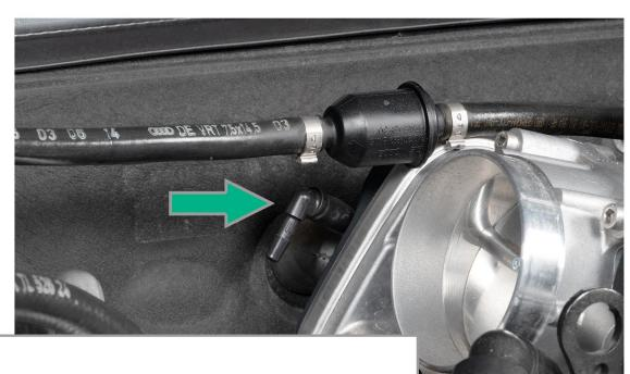
Install vacuum barb into vacuum hose located behind the throttle body.
