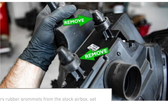
Remove the factory rubber grommets from the stock airbox, set them aside for reinstall. Note: If you do not see these grommets on the airbox, they may be in the frame rail.
