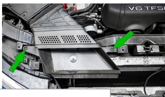
Remove the two bolts from the intake snorkel using a T25 torx driver.
