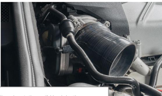
Loosely install silicone hose to the manifold and plug the vacuum barb into place.
