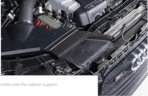
Reinstall OEM Snorkle onto the radiator support.
