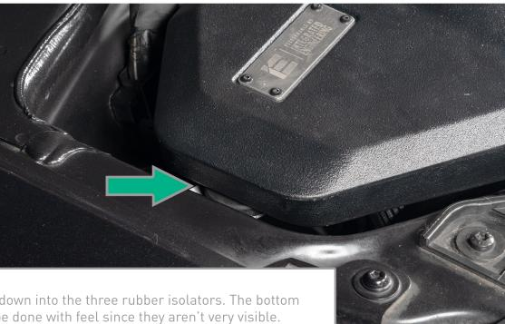
Press the intake down into the three rubber isolators. The bottom two will have to be done with feel since they aren't very visible.
