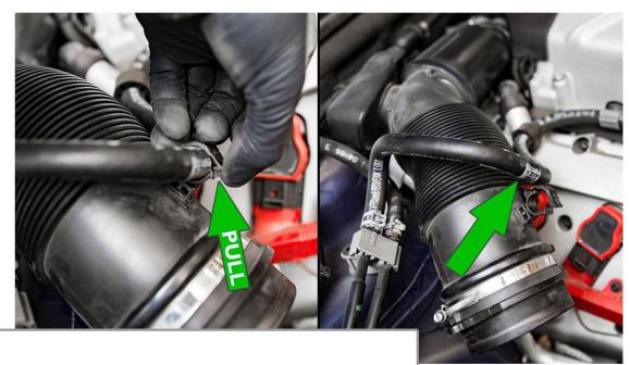
Pull up on the hose clip to release the fuel line from the intake pipe, safely set fuel line outside the clip.
