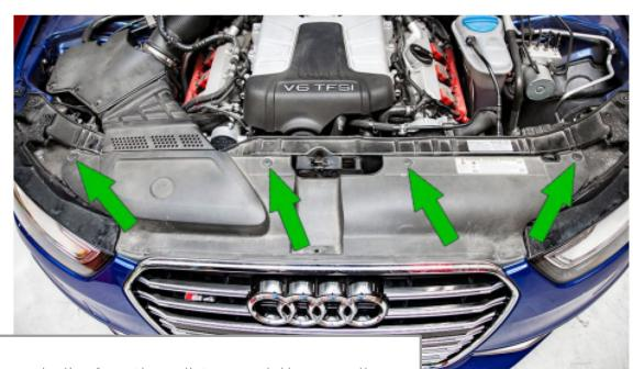
Remove the four push clips from the radiator cowel. Use a small flathead to depress the center pin of the clip, then pull to remove entire clip.
