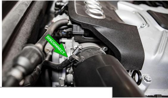
Disconnect the vacuum line from the intake pipe by carefully pulling it off the barb fitting.
