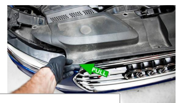
Carefully pull up on the edges of the cowel to release it, remove it from the vehicle and set aside.
