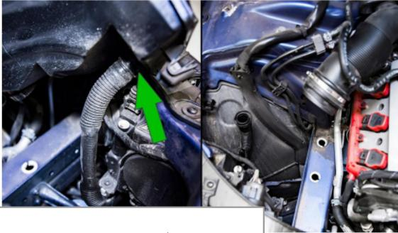
Carefully pull the airbox up and disconnect the SAI (secondary air injection) hose from the underside of the airbox. Remove the airbox completely.
