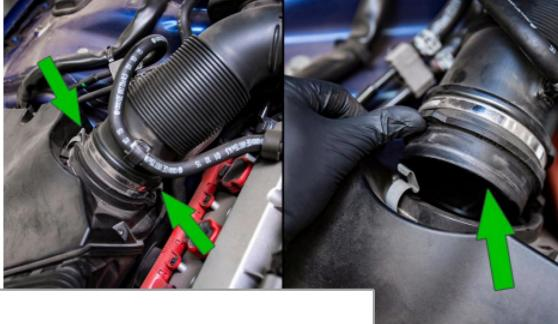
Disconnect the metal retaining clips and separate the inlet pipe from the airbox.
