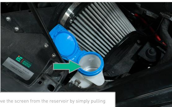
If equipped, remove the screen from the reservoir by simply pulling it straight up.
