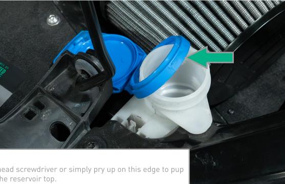
Use either a flat head screwdriver or simply pry up on this edge to pup the blue ring off the reservoir top.
