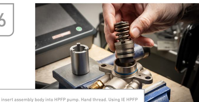
assembly tool, torque to 40 ft-lb.
