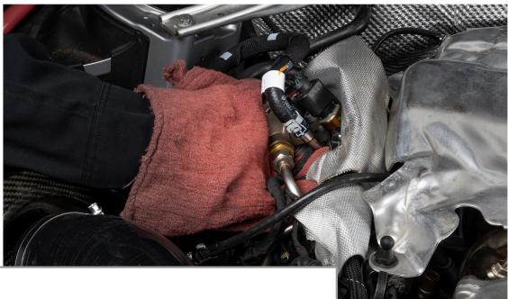
Place rag over fuel supply line and remove clamp using pliers.
