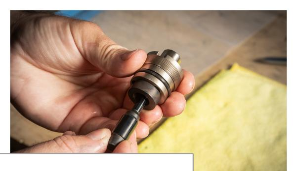
Coat pin in included assembly lube.
