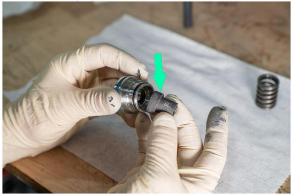
Slide pin into the new IE barrel and fuel pump nut.
