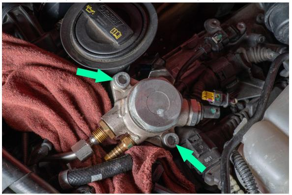
Install and tighten the 17mm fuel line nut.
