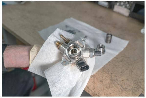
Carefully remove blue O-Ring with a pick located on the OE fuel pump nut.
