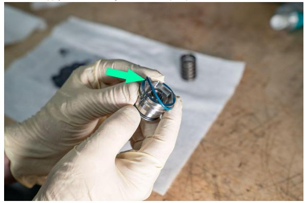
Apply supplied lubricant to the pin and spread over the whole pin.
