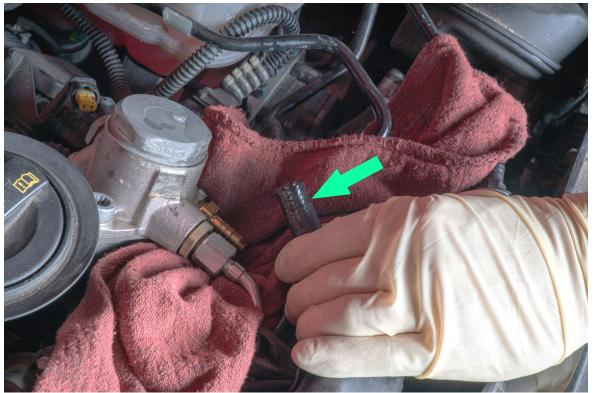
Remove fuel line nut with a 17mm open ended wrench.
