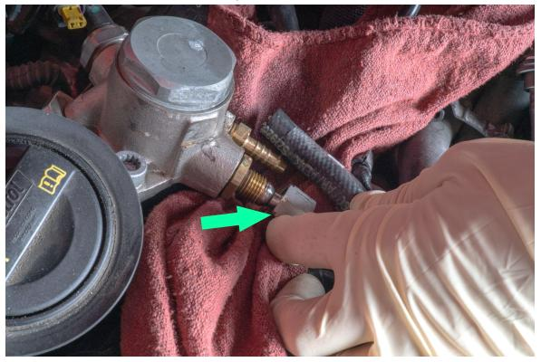
Use a #10 triple square to remove 2 bolts on the fuel pump.
