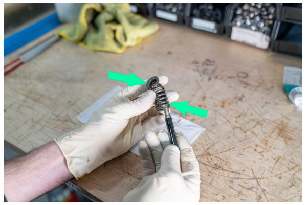
Remove the IE pump internals from the box, and place in a clean location.
