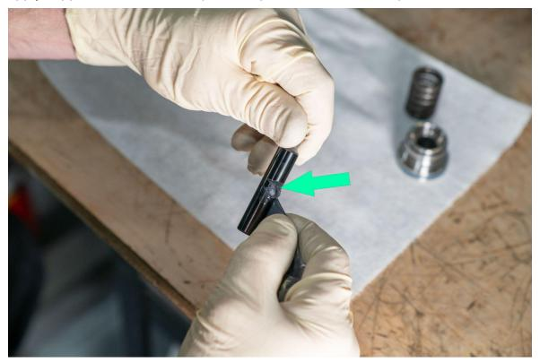
Install barrel into fuel pump nut.
