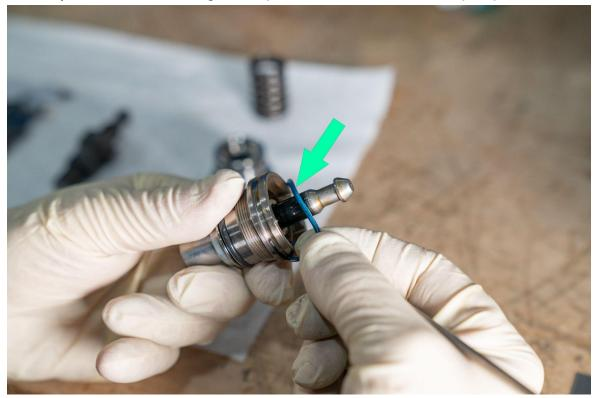
Clean and apply the OE O-Ring onto the new pump nut insert.
