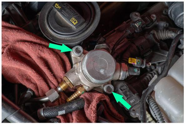
Remove the fuel pump from the engine bay by pulling up.
