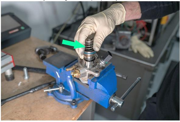
Install IE internals by threading in the fuel pump nut by hand
