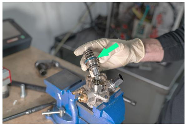
Push the pin up to release the retainer, then remove the pin from spring.
