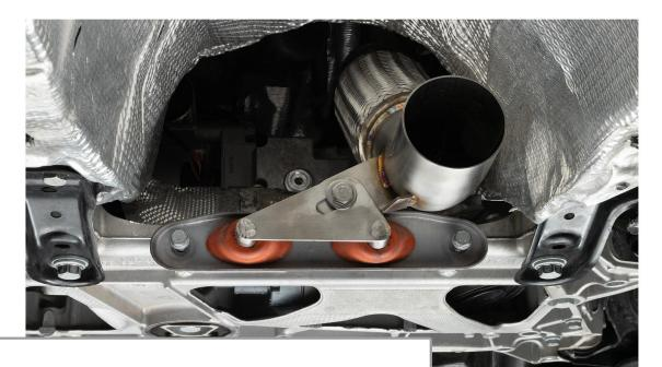
Press ie mount into stock mount then Install stock mount using 2 17mm bolts previously removed.
