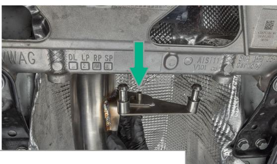
Install included dp mount onto ie dp using included nut washer and bolt using 15mm for nut 17mm for bolt
