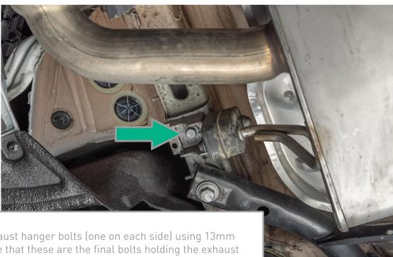
Remove two exhaust hanger bolts (one on each side) using 13mm socket. Take note that these are the final bolts holding the exhaust up, so be ready for it to drop. Ideally it's good to have another pair of hands ready to pull the exhaust.
