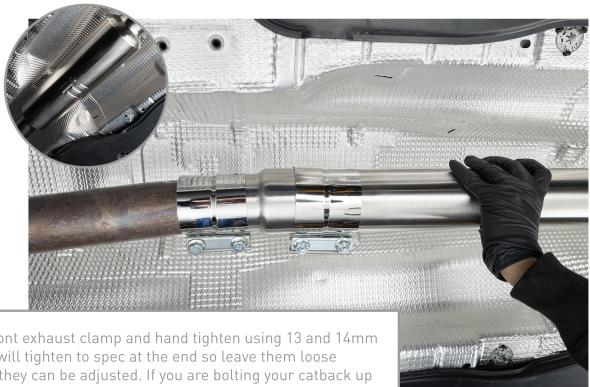
Install the front exhaust clamp and hand tighten using 13 and 14mm drivers. You will tighten to spec at the end so leave them loose enough that they can be adjusted. If you are bolting your catback up to an OE downpipe, you will use the reducer as seen above. If you have an aftermarket downpipe and have purchased the IEEXDB3-1 optional resonator, you will install it in place of this front section.
