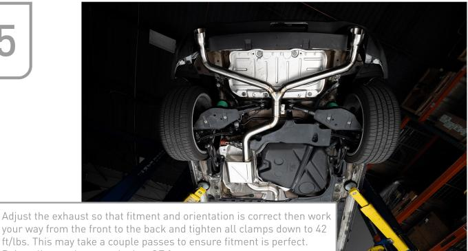
your way from the front to the back and tighten all clamps down to 42 ft/lbs. This may take a couple passes to ensure fitment is perfect. Reinstall cross beam and other OE fasteners.
