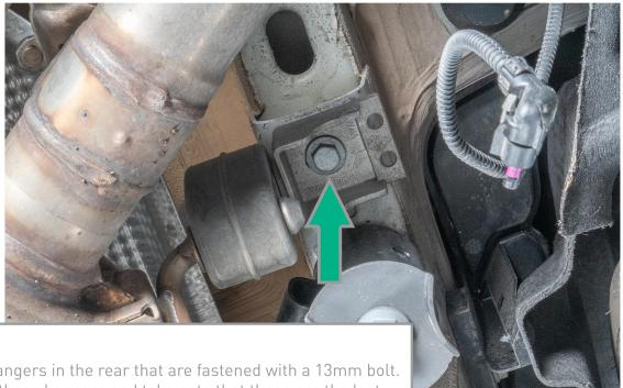
There are two hangers in the rear that are fastened with a 13mm bolt. Remove both of these hangers and take note that these are the last fasteners holding up the exhaust so before removing them, have a friend ready to help you lift the OE cat back down and away from the vehicle.
