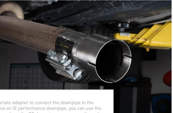
Install the appropriate adapter to connect the downpipe to the catback. If you have an iE performance downpipe, you can use the straight clamp, if you have the OE downpipe, you can use the reducer shown.
