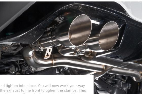
Install your tips and tighten into place. You will now work your way from the back of the exhaust to the front to tighen the clamps. This will ensure proper alignment. Once the fitment is to your liking, tighten down all the clamps to 40 ft/lbs
