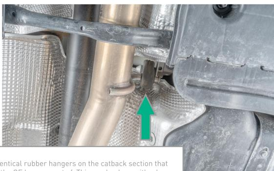
There are two identical rubber hangers on the catback section that you need to pull the OE hangers out of. This can be done with a long flathead or harnger removal tool. Remove the exhaust from the rubber hangers and allow the rubber to stay mounted to the top hanger.
