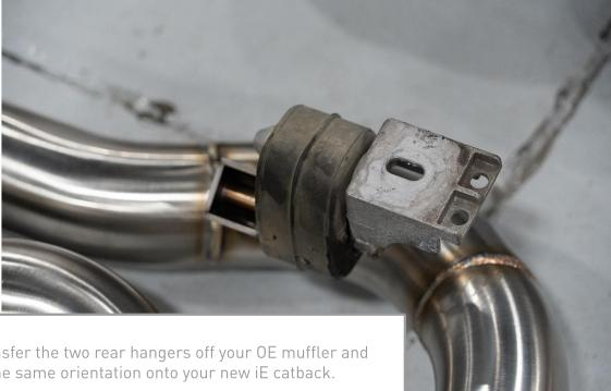
Remove and transfer the two rear hangers off your OE muffler and install them in the same orientation onto your new iE catback.
