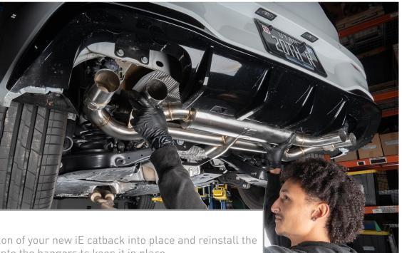
Lift the rear section of your new iE catback into place and reinstall the two 13mm bolts into the hangers to keep it in place.
