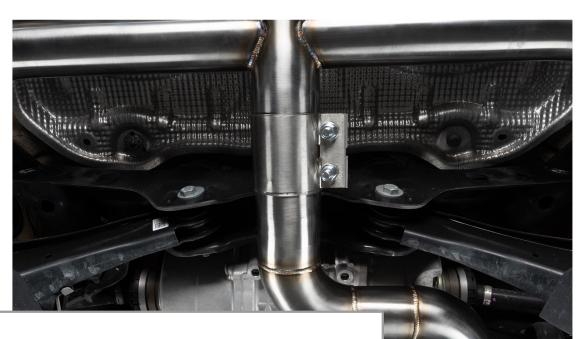
Install the clamp to connect the rear and front section of your iE catback and loosely tighten.
