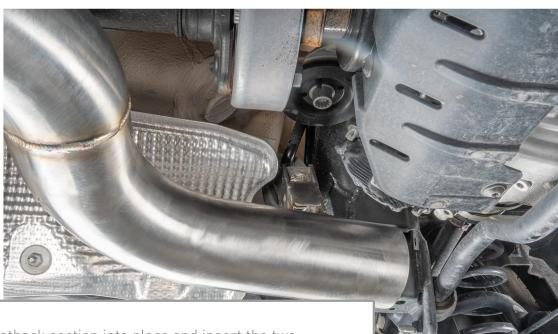
Raise the front catback section into place and insert the two hangers into the rubber hangers that are still attached to the chassis.
