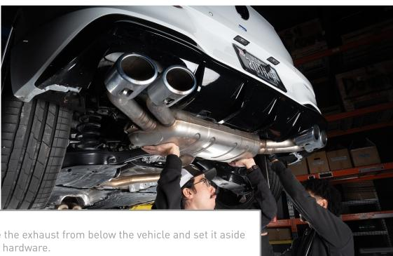
Carefully remove the exhaust from below the vehicle and set it aside to transfer some hardware.
