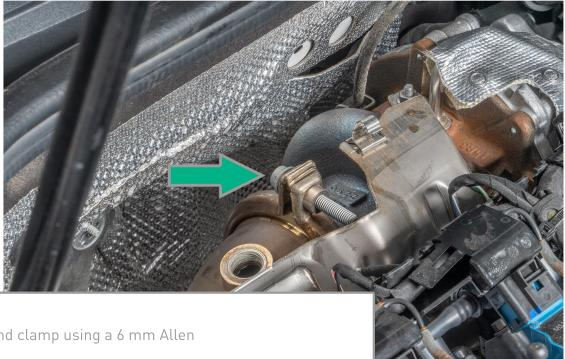
Loosen the V band clamp using a 6 mm Allen
