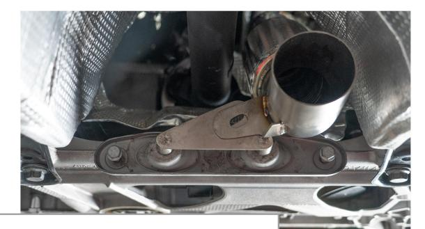
Install the mount in place on the subframe.
