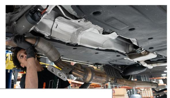
Remove the downpipe by pulling it out the bottom of the vehicle.
