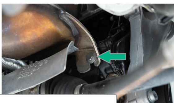
Remove 13mm downpipe mounting bolt
