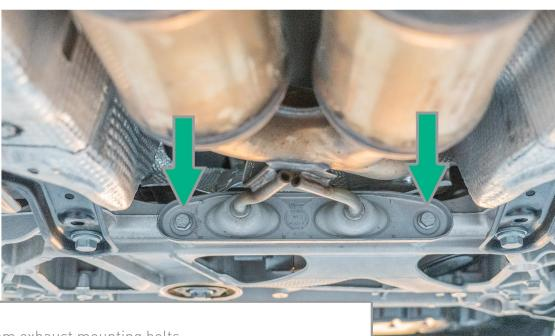
Remove two 13mm exhaust mounting bolts
