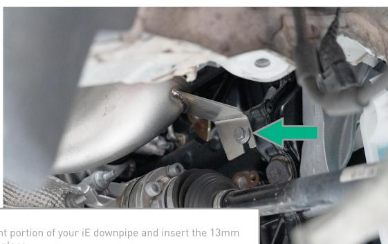
Raise up the front portion of your iE downpipe and insert the 13mm bolt to keep it in place.
