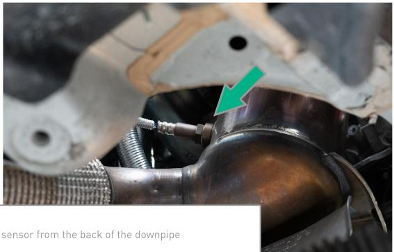
Remove rear 02 sensor from the back of the downpipe
