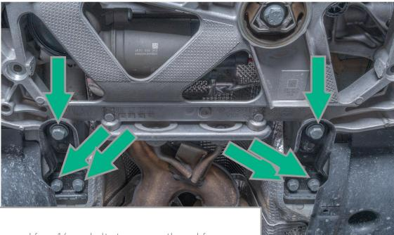
Remove two 18mm and four 16mm bolts to remove the subframe mounts
