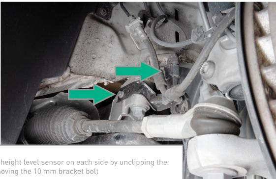
Remove the ride height level sensor on each side by unclipping the harness and removing the 10 mm bracket bolt
