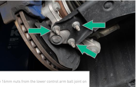
Remove the three 16mm nuts from the lower control arm ball joint on each side
