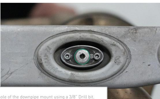
Drill out center hole of the downpipe mount using a 3/8" Drill bit. This will allow you to remove the OE Mount from the OE downpipe. Once it has been drilled, pry off the mount and reinstall the mount on your iE downpipe.
