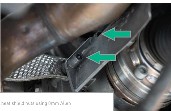
Remove two axle heat shield nuts using 8mm Allen
