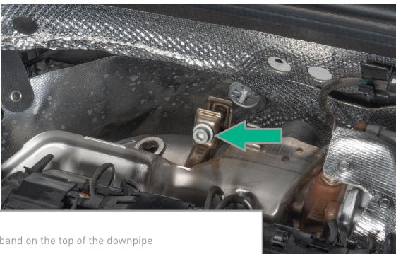
Loosely install v band on the top of the downpipe
