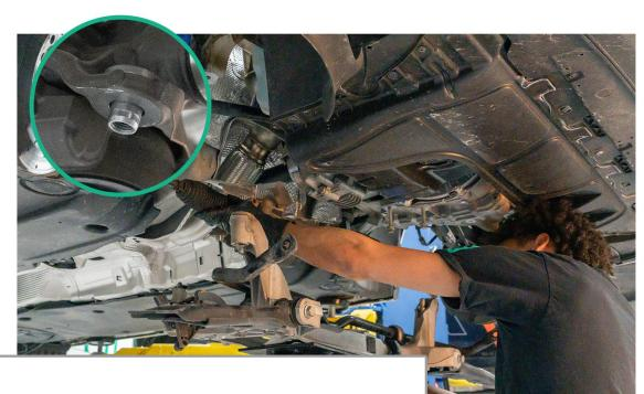
Reinstall subframe in reverse order. Take note when raising the subframe back into place, there are alignment pins on the steering rack that help alignment of the subframe. You can see these pins in the detailed view bubble in the top left of the photo.
