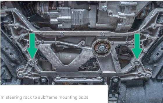
Remove two 18mm steering rack to subframe mounting bolts
