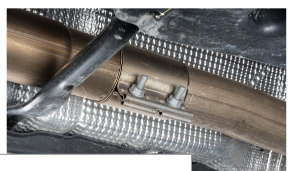
Remove the exhaust clamp that secures the downpipe to the catback portion of the exhaust using a 15mm socket.
