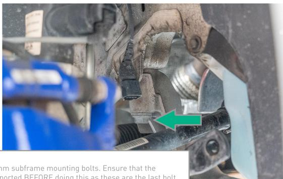
Remove two 18mm subframe mounting bolts. Ensure that the subframe is supported BEFORE doing this as these are the last bolt holding it up
