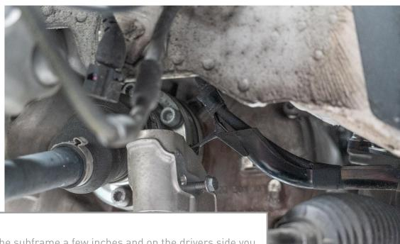
Begin to lower the subframe a few inches and on the drivers side you will see a black mount for the steering rack wire harness, unclip that.
