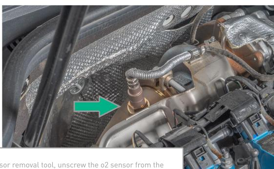
Using an o2 Sensor removal tool, unscrew the o2 sensor from the OE downpipe.
