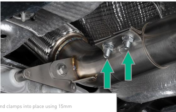
Install midpipe and clamps into place using 15mm
