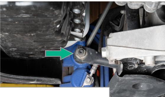
Remove the sway-bar end link nut from the sway bar using an 18 mm socket. You may need to use a 6mm triple square to counter hold the end link.
