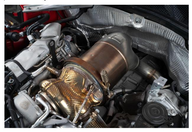
Insert supplied bolts into the downpipe. (6 will be required for most aftermarket mid pipes. 4 will be required if installing onto factory OEM midpipes due to factory studs)
