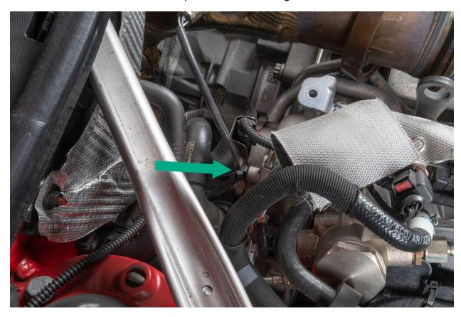
Use 22mm wrench to loosen and remove the o2 sensor from the downpipe.
