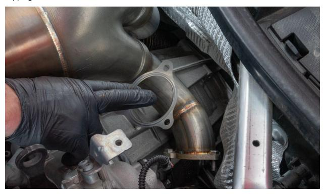
Orient the mid pipes onto the bolts and then install nuts and tighten. Again, you will need to get creative with your available sockets and wrenches to reach the back bolts/nuts. You may want to remove the v-band clamp as well during this process to help orient the downpipe for best access.
