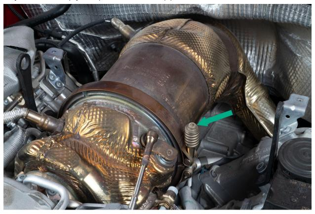
Remove six (Three on each side) 12mm nuts that connect the downpipe to the midpipes. The two nuts in the back can be very difficult to gain access to. A long extension applied from underneath the vehicle is easiest or you will need to be creative with extensions, wobble sockets, and wrenches.
