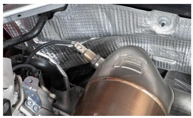
Once all bolts/nuts have been tightened, reinstall v-band clamp and tighten.
