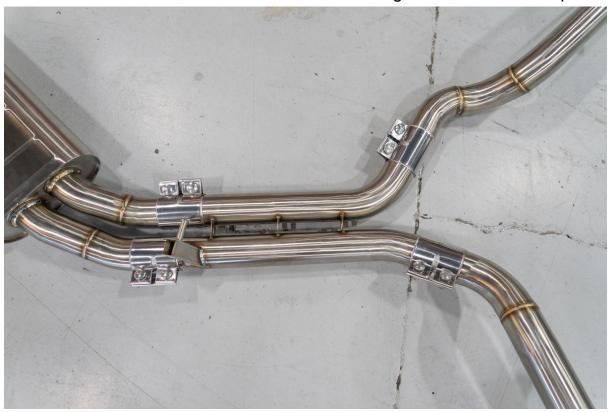
Use the provided zip tie to get the exhaust valve connector secured out of the way
