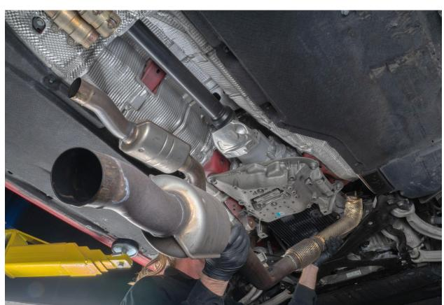
Remove the exhaust hangers from OEM Midpipe by using an exhaust hanger removal tool or pry off with pry bar
