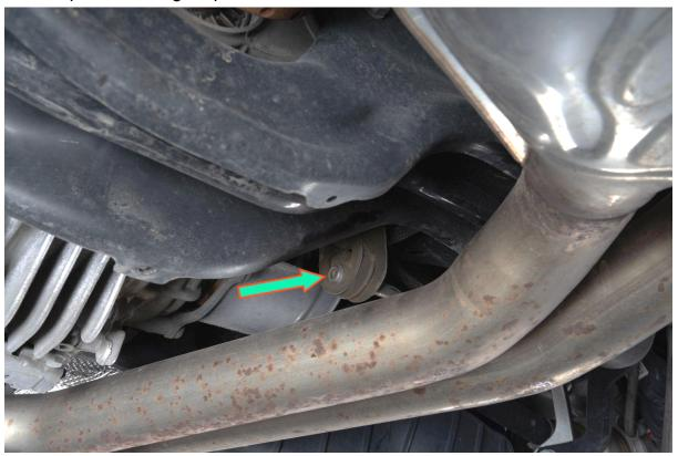
Assemble the catback rear and middle section using the four 63mm clamps
