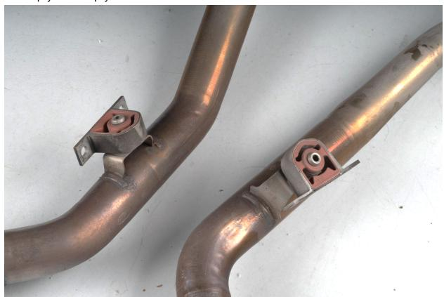
Reinstall exhaust hangers onto IE Midpipes. A small spray of lubrication can make this step easier
