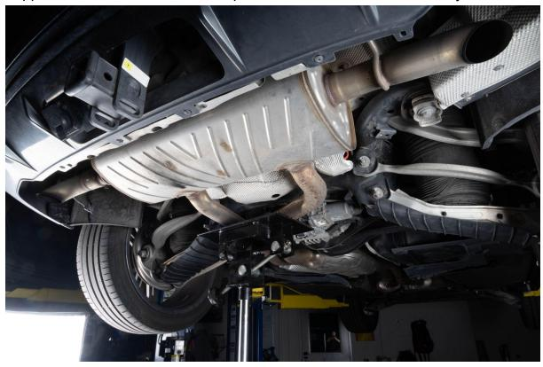
Remove two (one per side) 13mm bolts that secure the muffler to the body
