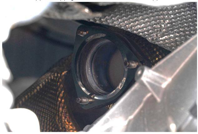
Raise front section of midpipe into engine bay then loosely fit exhaust hanger bolts and downpipe nuts.
