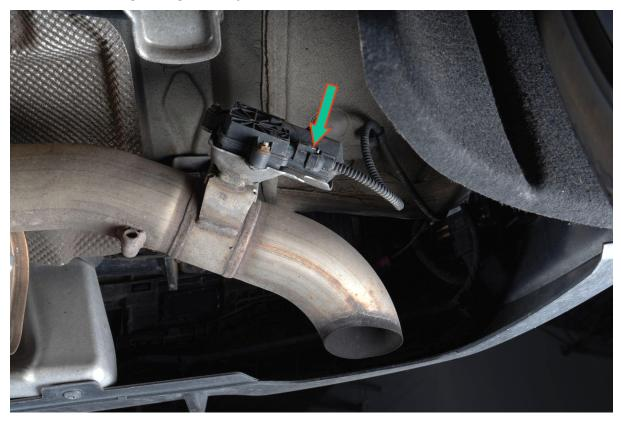
Support the muffler with either help from a friend of a transmission jack
