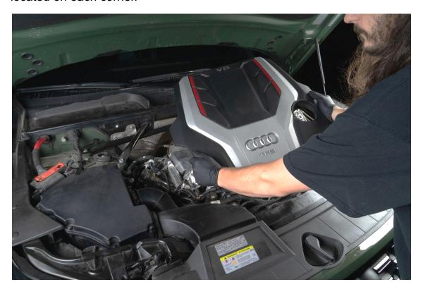
Remove four 13mm Engine Cover Mounts then remove Heat Shield from Engine Bay
