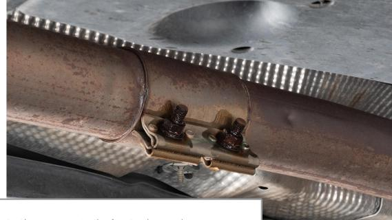
Apply some penetrating spray onto the front exhaust clamp nuts/bolts. You can give the spray some time to work and come back after a few minutes. Then loosen both 13mm Nuts and push the clamp back onto the rear portion of the exhaust.
