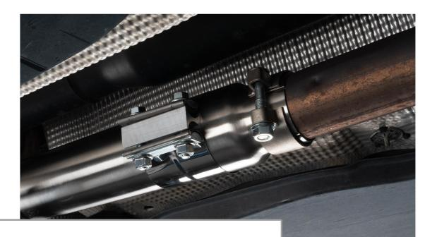
Assemble the reducer and install it on the front section of the IE Catback.
