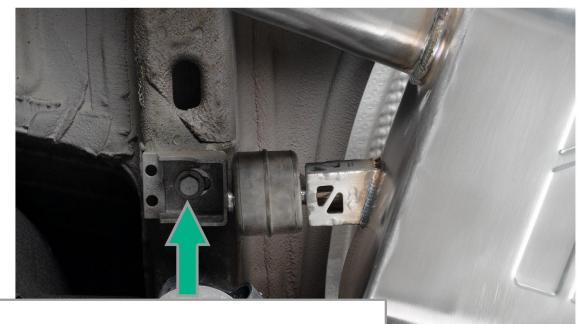
Raise the muffler section into place and reinstall the OEM Hanger bolt.
