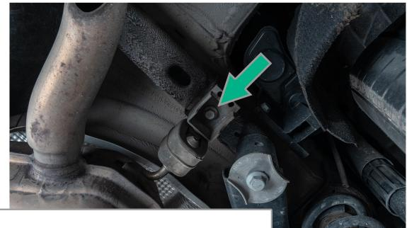
Remove both rear 13mm bolts that secure the two rear hanger. Be prepared because once these are removed, the exhuast will drop.
