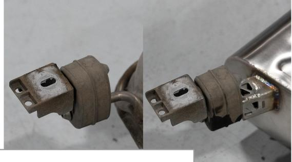
Remove the drivers side hanger from the OE exhaust to your new IE Performance Exhaust.
