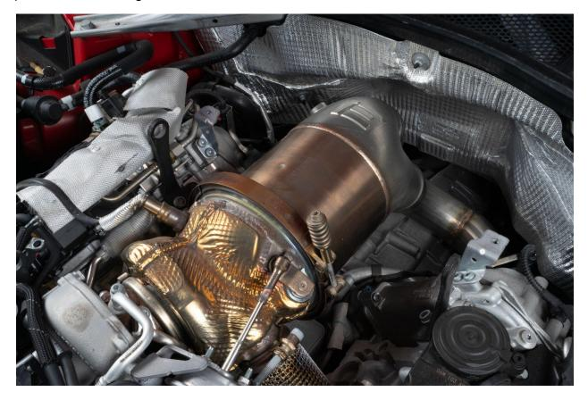
Insert Six supplied bolts into downpipe. Three on each side.
