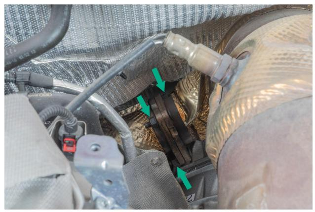
Use Trim removal tool to remove zip tie fastener holding o2 sensor wire.
