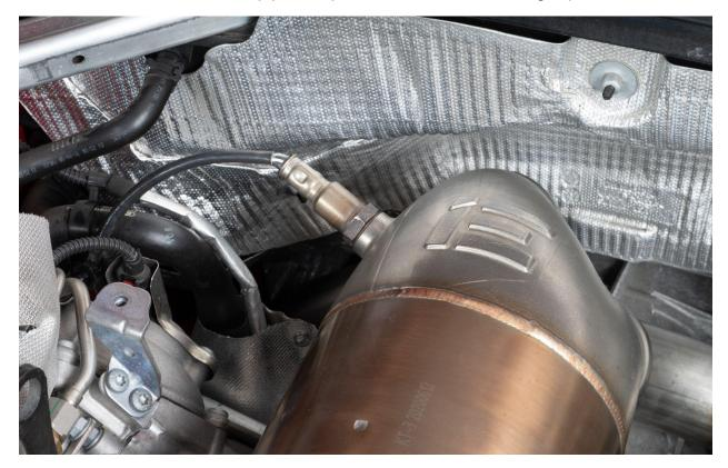
Once all six bolts/nuts have been tightened, reinstall vband clamp and tighten.
