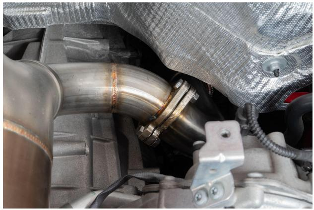
Reinstall o2 Sensor onto downpipe and press back in wire retaining clip
