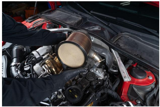
Loosely install v band clamp to fasten IE downpipe to turbo. This will help hold it in place while inserting rear bolts.
