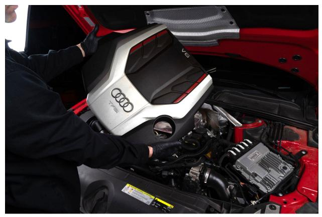
Remove four 13mm Engine Cover Mounts then remove Heat Shield from Engine Bay
