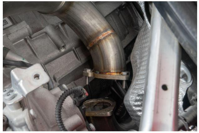
Install gasket onto the bolts. Press the gasket flush with the downpipe to prevent it from slipping off.
