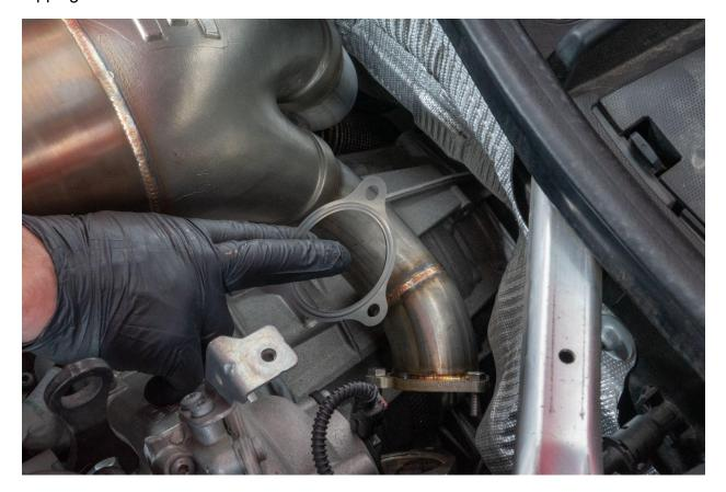
Orient the midpipes onto the bolts and then install six nuts and tighten. Again, you will need to get creative with your available sockets and wrenches to reach the back bolts/nuts. You may want to remove the vband clamp as well during this process to help orient the downpipe for best access.
