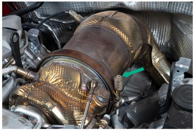
Remove six 12mm bolts that connect the downpipe to the midpipes. The two bolts in the back can be very difficult to gain access to, and remove. You will need to be creative with extensions, wobble sockets, and wrenches. Pushing the downpipe back towards firewall can also help with clearance.
