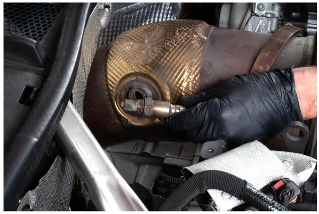
Lift stock downpipe out of the engine bay.
