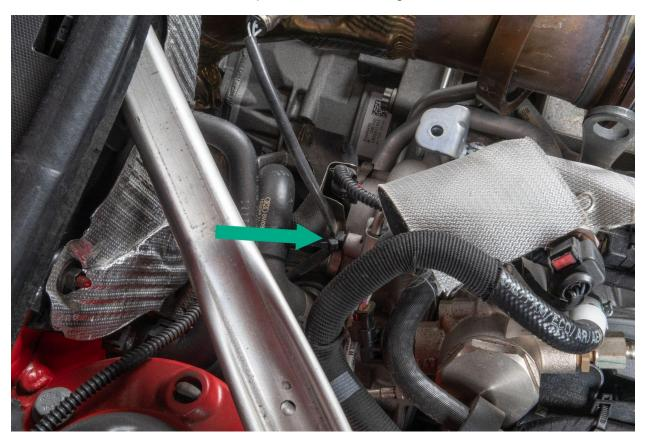
Use 22mm wrench to loosen and remove the o2 sensor from the downpipe.
