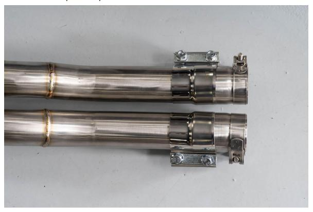
Install center portion of IE exhaust on the vehicle
