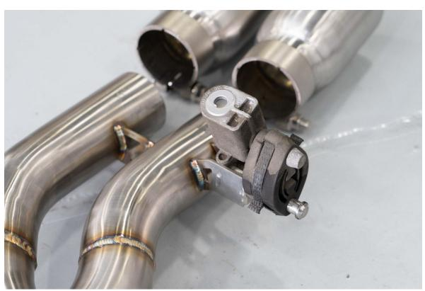
Loosely install tail pipe sections of IE exhaust and fasten to vehicle with the 13mm bolts
