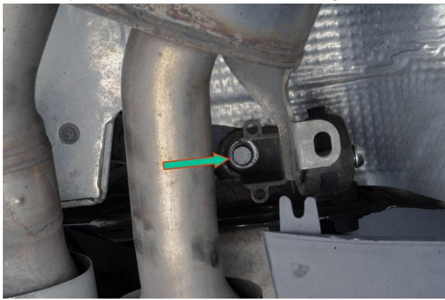
Push out the last exhaust hanger located near the resonator. Be prepared for exhaust to drop from the car. An extra set of hands is helpful here. Then remove the entire rear muffler section from vehicle
