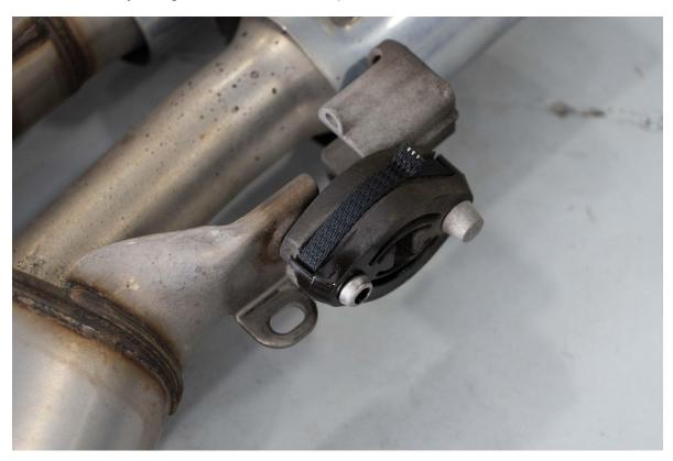
Reinstall hangers onto IE Exhaust.
