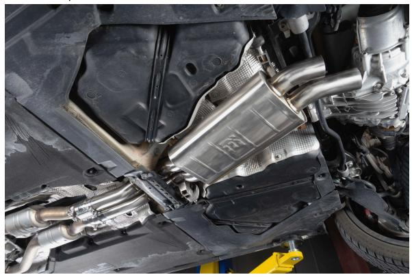
Loosely install middle section of the IE exhaust between muffler and rear sections
