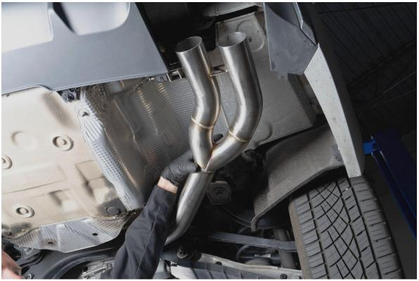
Remove center exhaust hanger in front of resonator
