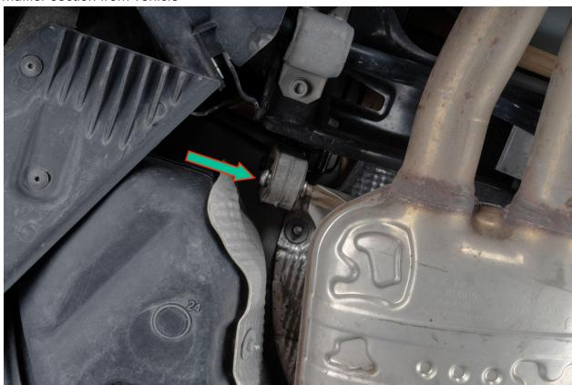
Remove factory hangers from the muffler portion.
