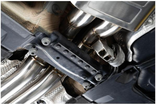
Tighten exhaust clamps starting from the front to the back, take care to align the pipes as you go
