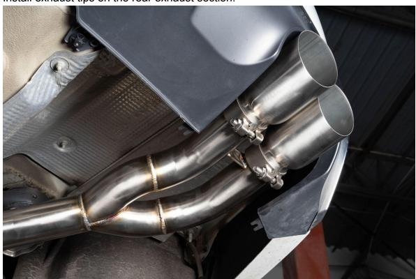
Tighten rear exhaust hangers while taking care to try and level the tail pipes. Ensure that the tips are not making contact with the rear valence. If they are, loosen the exhaust clamps, reorient, and retighten. This may take a couple of tries to get perfect
