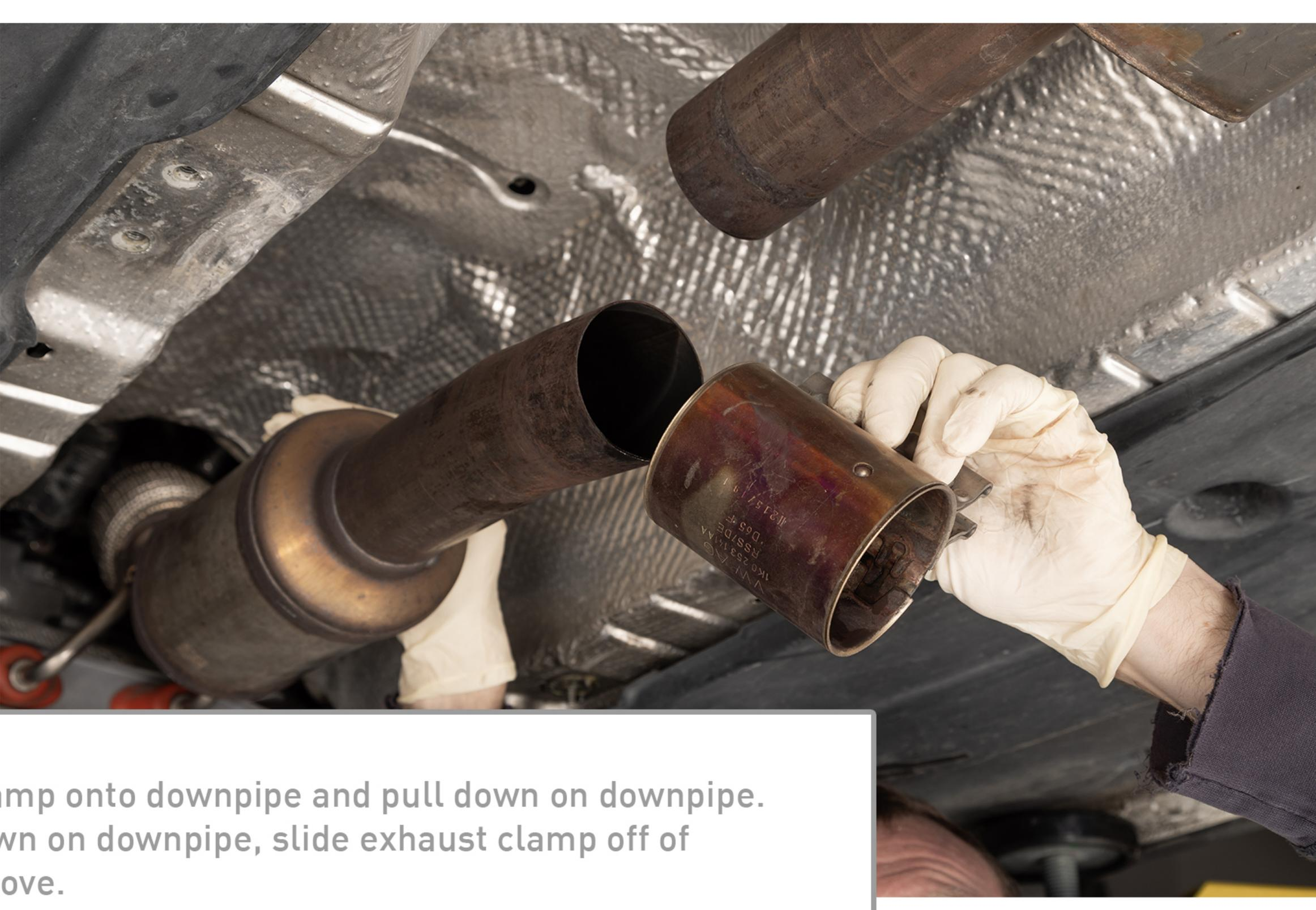
Slide exhaust clamp onto downpipe and pull down on downpipe. While pulling down on downpipe, slide exhaust clamp off of downpipe to remove.
