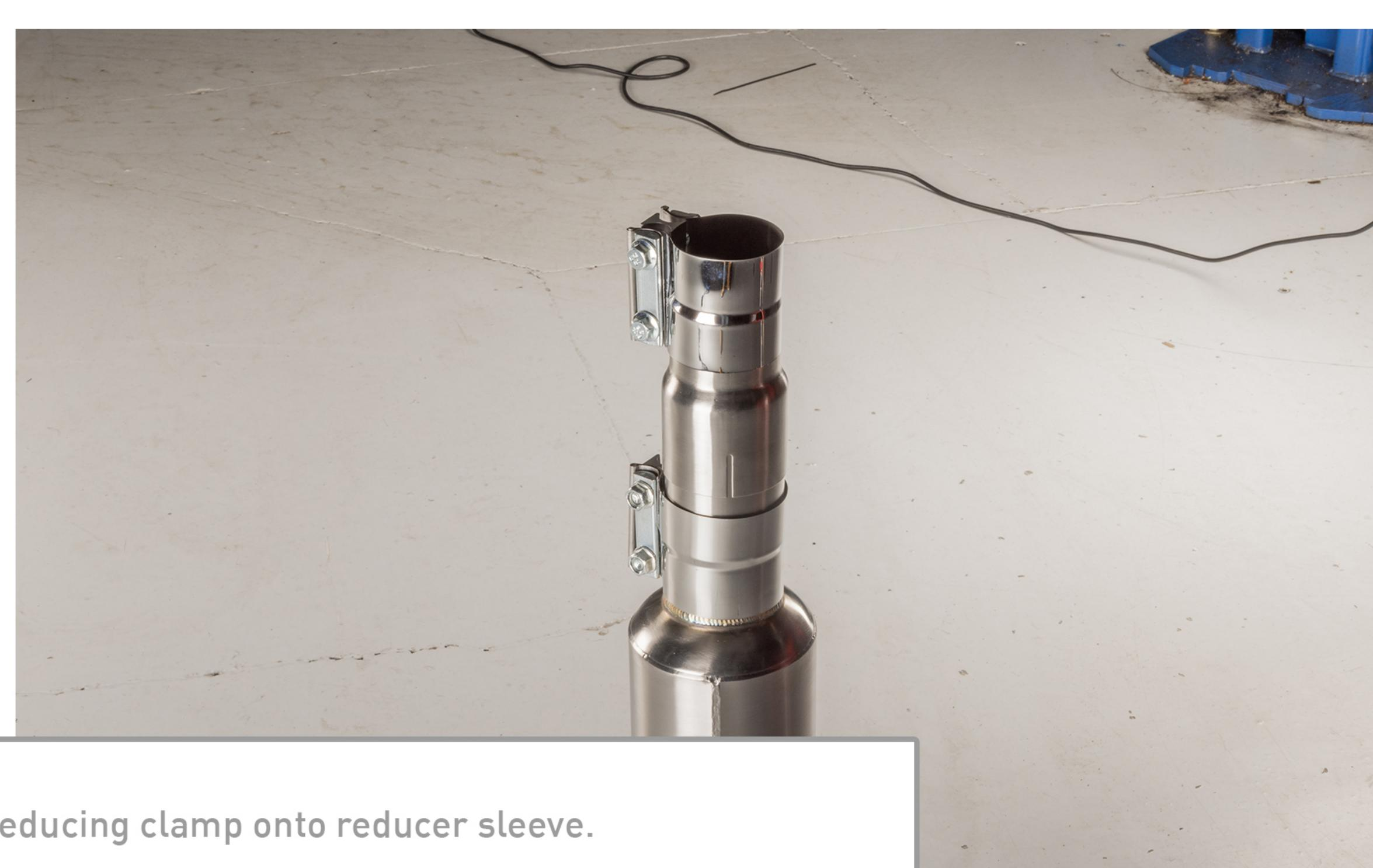
Slide provided reducing clamp onto reducer sleeve.
