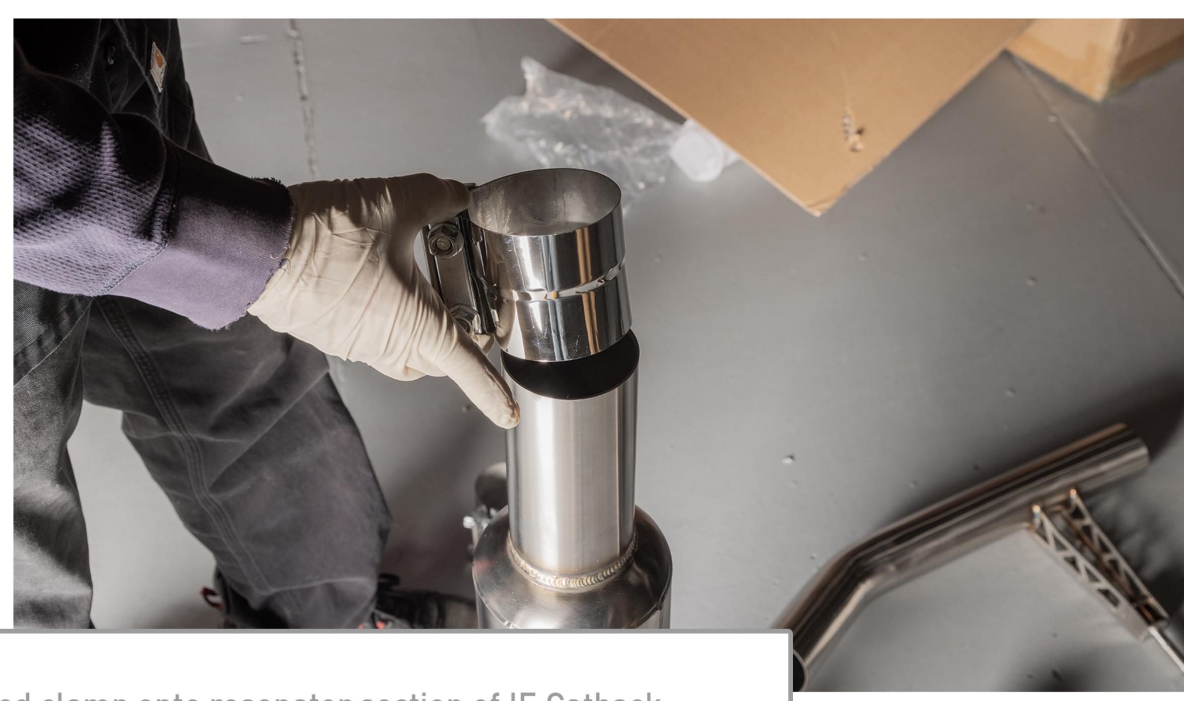
Slide the provided clamp onto resonator section of IE Catback.
