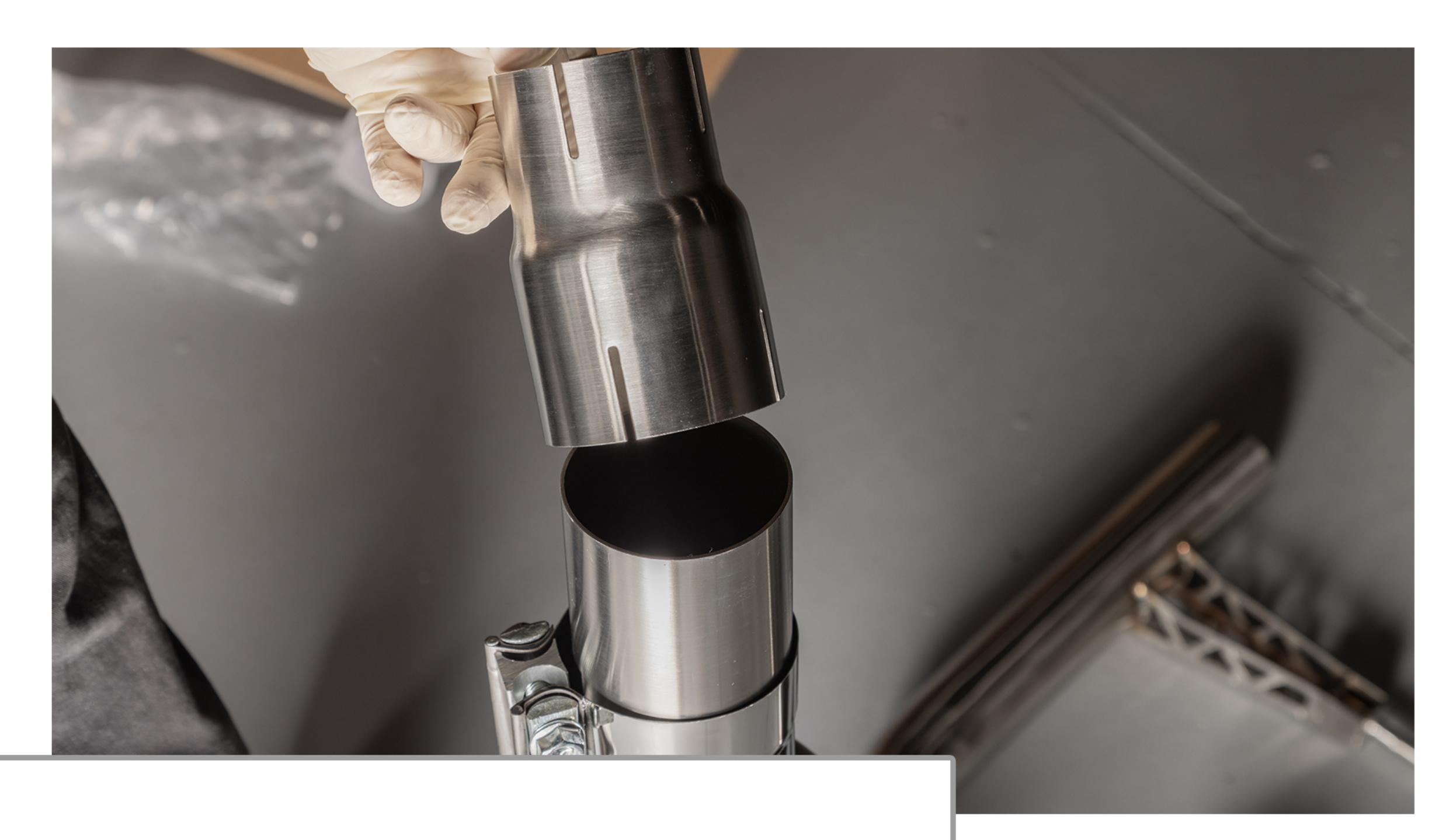
Slide provided reducer sleeve onto IE resonator. (Reducer sleeve not needed when installing with an IE Downpipe.)
