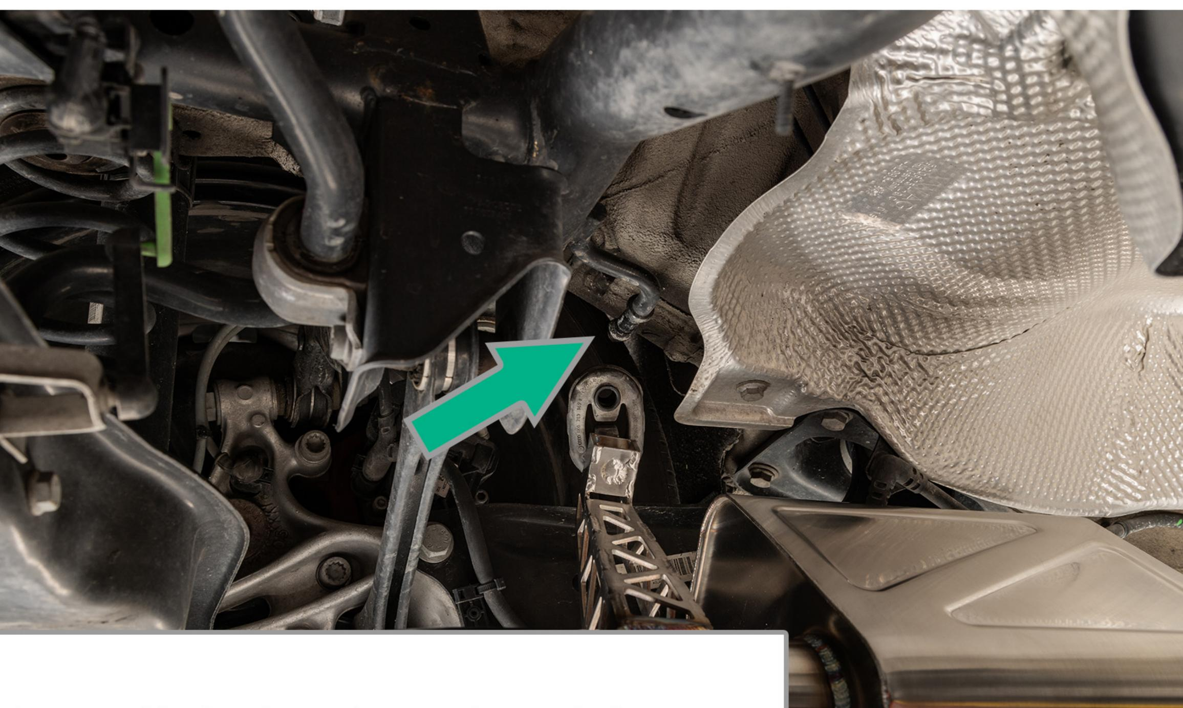
Hang muffler section onto black exhaust hanger forward of rear driver side wheel.
