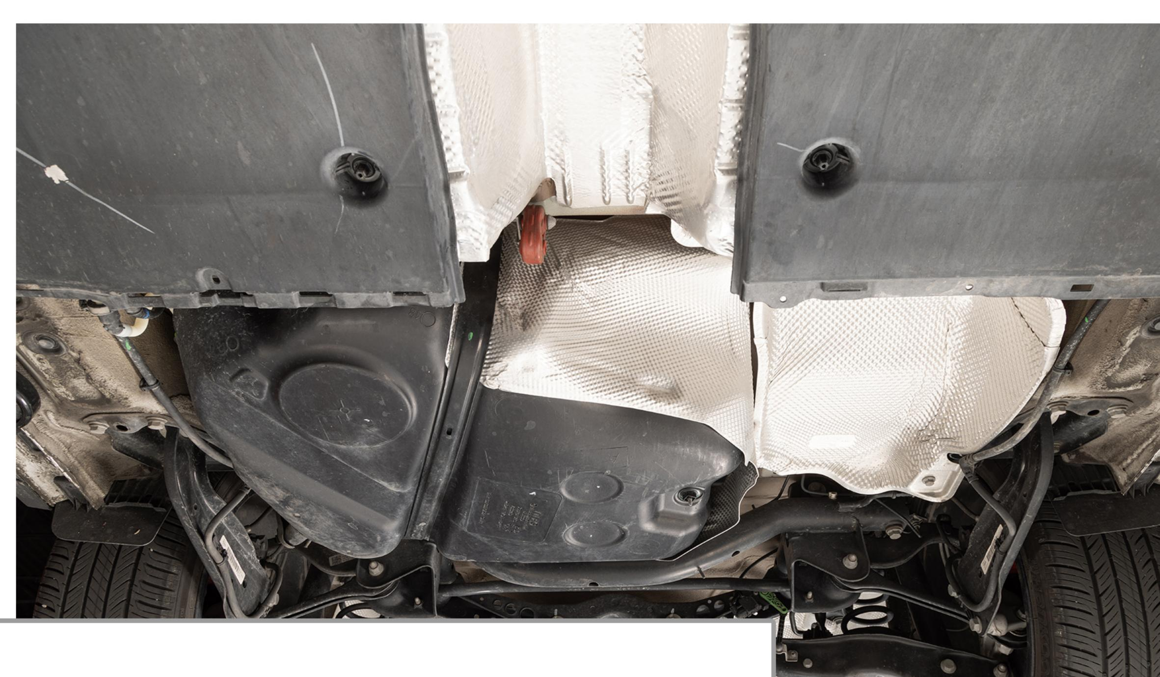
Using a second set of hands, lower and remove stock exhaust system from vehicle.
