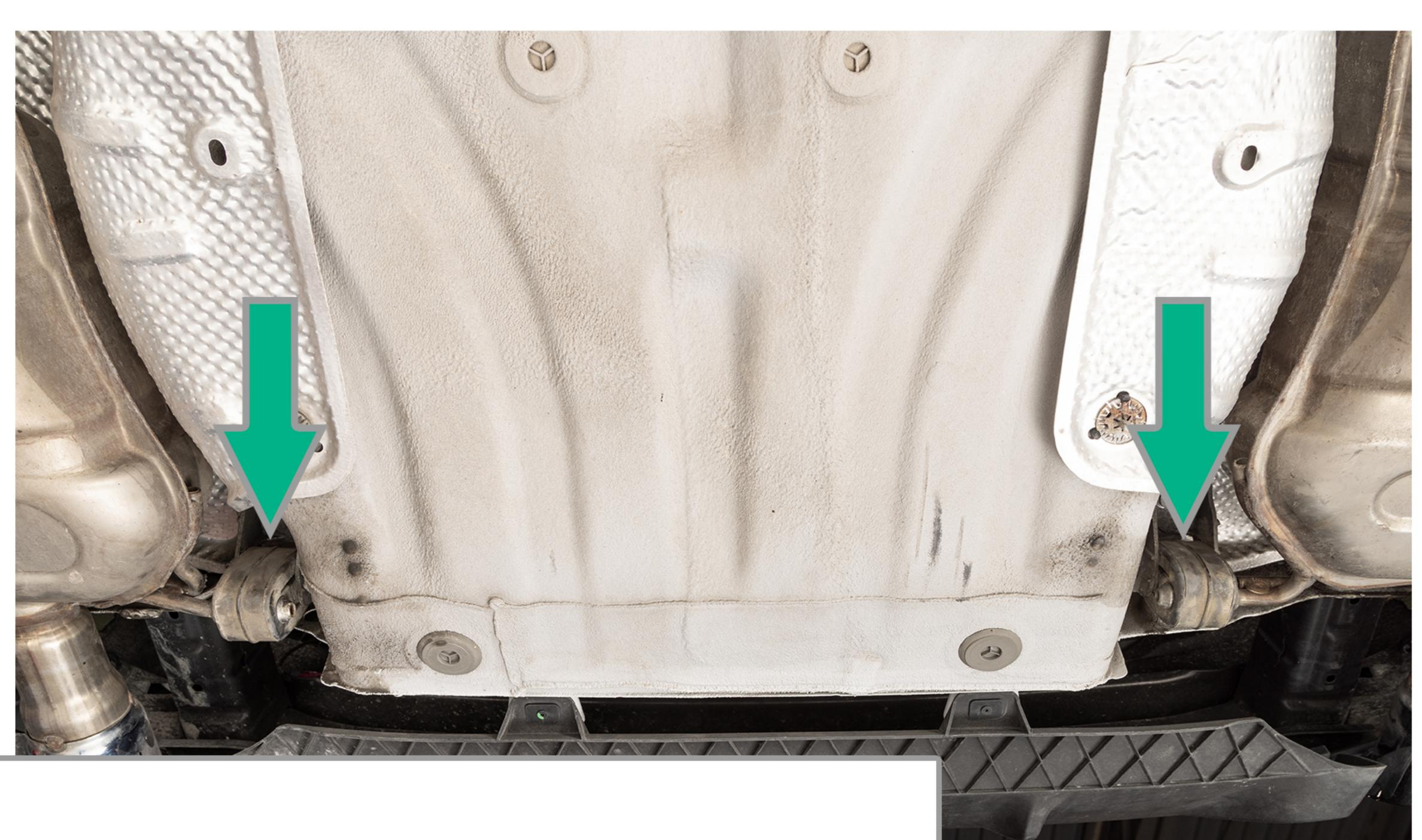
Remove 2 13mm bolts from rear most muffler exhaust hangers. Use a second set of hands to support stock exhaust and prevent it from falling.
