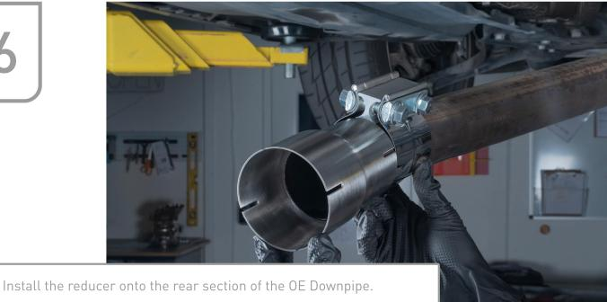
From here forward, when installing, all the clamps will be very loosly installed to allow adjustment at the end. So don't clamp them down until instructed.
