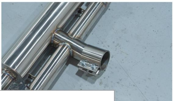
Slide the supplied clamp onto the front of your IE Muffler section.
