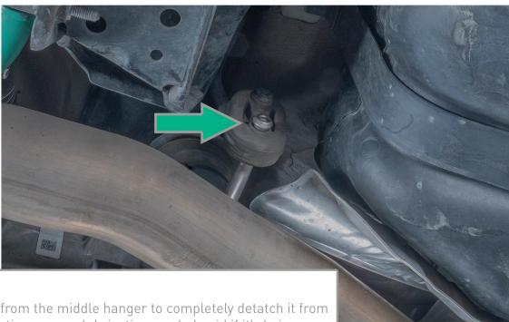
Pull the exhuast from the middle hanger to completely detatch it from the vehicle. Sometimes some lubrication can help aid if it's being stubborn.
