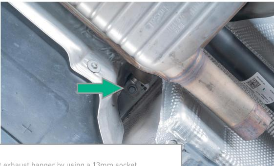
Remove the front exhaust hanger by using a 13mm socket.
