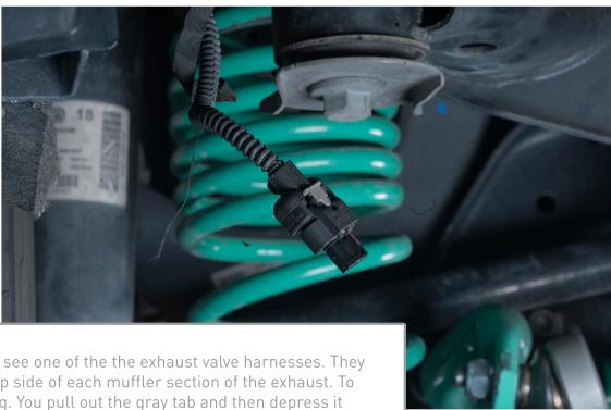
Pictured you will see one of the the exhaust valve harnesses. They are located on top side of each muffler section of the exhaust. To remove each plug. You pull out the gray tab and then depress it while pulling the harness away from the plug.
