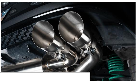
Install your IE Catback Tips and adjust the distance in which they stick out to your liking. Once they're in place, tighten the 14mm clamps. If you'd like, you can also install the clamps on the top side as well.
