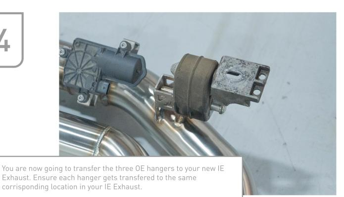
Lubrication and/or an exhaust hager removal tool can greatly aid removal/reinstallation of the hangers.
