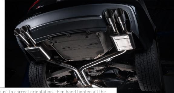
Adjust the exhaust to correct orientation, then hand tighten all the clamps from the front moving backwards while ensuring everything stays in place. Once everything looks right correct, tighten all the clamps to 42 ft/lbs.
