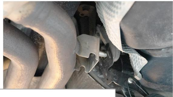
Using an hanger removal tool, or a pry bar, remove the hanger from the rubber isolator on the other side.
