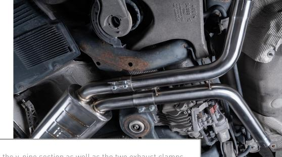
Loosly install the y-pipe section as well as the two exhaust clamps. Do not fully tighten clamps yet as there will be adjustments made before they are fully tightened down.
