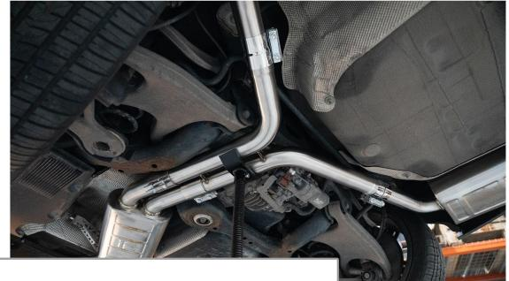
Ideally support the center of the exhaust to help make adjustments easier.
