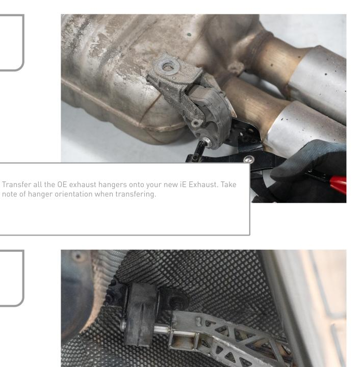
Lift the resonated section of your iE Exhaust into place and simultaneously insert the hanger into the isolator as well as reinstall the opposing hanger back into place with the 13mm nuts.
