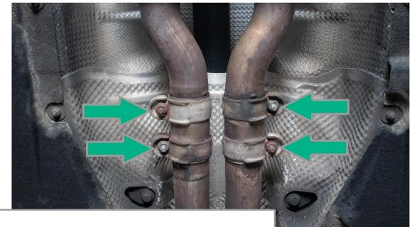
Use a 13mm driver to loosen OE exhaust clamps that connect the catback to the catted section of the exhaust.
