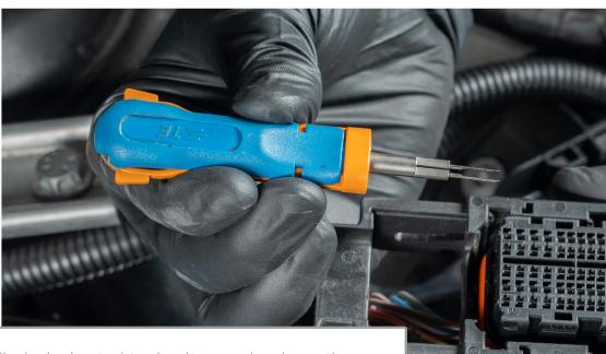
We use the specific depinning tool to simultaneously release the clip on the pin and push it out from the harness at the same time. You can now do so on Pin 71.
