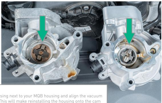
Lay the OEM housing next to your MQB housing and align the vacuum pump drive key. This will make reinstalling the housing onto the cam smoother. Those teeth align and insert into a groove on the camshaft.
