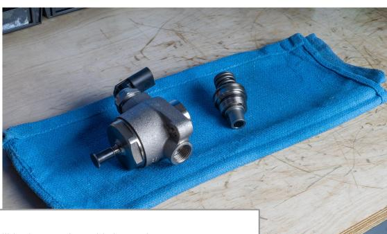
Prepare an incredibly clean surface, this is very important as any contamination can cause issues with seals or wear on the pin/cylinder and lead to premature failure.
