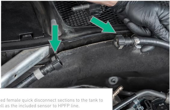
Install two provided female quick disconnect sections to the tank to sensor line as well as the included sensor to HPFP line.
