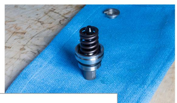
Install factory spring over the pin seated on the assembly body.
