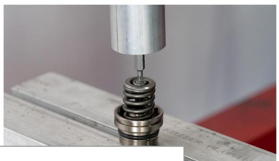
Using a hydraulic press, line up a similar-sized bit to the stock HPFP pin and press it out of the retainer to release the spring. Remove the stock spring and set aside for re-assembly with IE parts.
