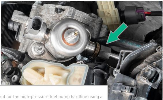
Loosen the flair nut for the high-pressure fuel pump hardline using a 17 mm wrench.
