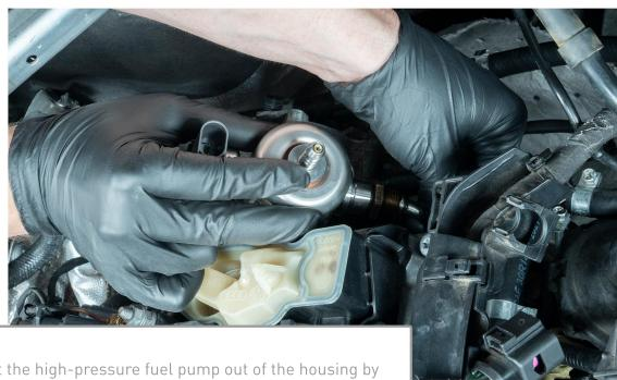
Next, you will lift the high-pressure fuel pump out of the housing by simultaneously applying upward pressure on the pump as well as downward-outward pressure on the hardline so you do not overstress or bend the hardline.
