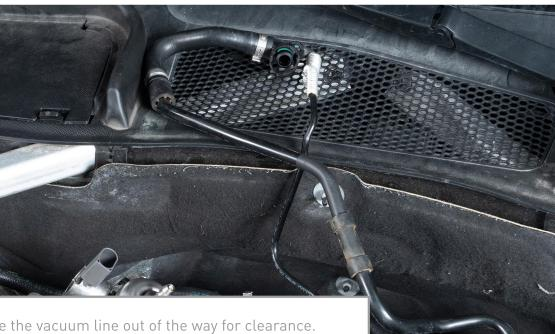
You can then move the vacuum line out of the way for clearance.
