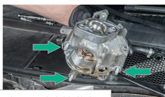
You will now remove the vacuum pump housing by loosining the Three 10mm bolts located on the backside of the housing. Pictured above you can see bolt location. Also note that there is a gasket between the cyinder head and the housing. We recommend replacing the gasket, but it can be reused.
