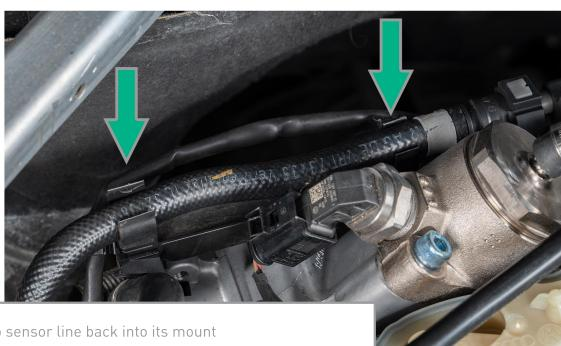
Press the tank to sensor line back into its mount
