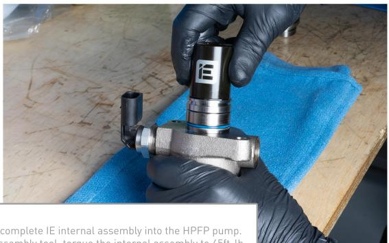
Hand thread the complete IE internal assembly into the HPFP pump. Using IE HPFP assembly tool, torque the internal assembly to 45ft-lb.
