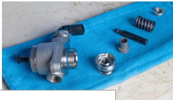
Lay out all the new IE components, pump body, and the stock spring in your clean environment. Inspect and clean all parts of any contaminants (dust, dirt, lint, etc.)
