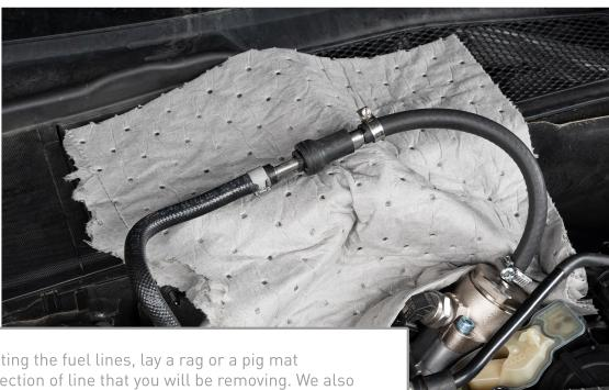
Before disconnecting the fuel lines, lay a rag or a pig mat underneath the section of line that you will be removing. We also recommend if the line has any pressure you lay a rag or pig mat on top of the section. You're about to remove to catch any pressurized fuel spray.
