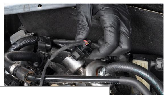
Remove the factory solenoid connector by lifting the tab and pulling straight away.
