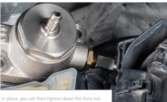
Once the pump is in place, you can then tighten down the flare nut
