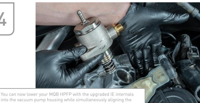
into the vacuum pump housing while simultaneously aligning the hardline on the side of the HPFP. We recommend hand starting and threading the flare nut on the hardline before bolting down the high pressure fuel pump housing so you can maneuver the hardline to seat correctly.
