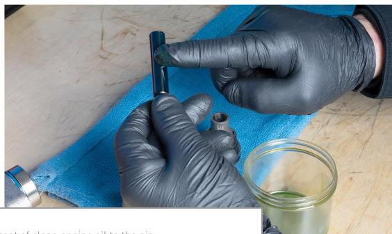
Apply generous coat of clean engine oil to the pin.
