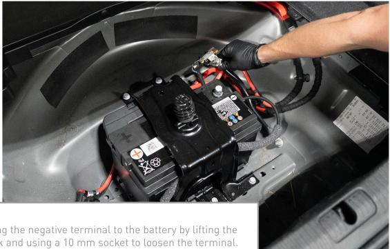
Begin by removing the negative terminal to the battery by lifting the cover in the trunk and using a 10 mm socket to loosen the terminal.
