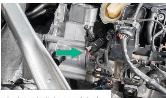
Once the teeth are aligned, ensure that the housing sits flush with the cylinder head before tightening any of the bolts failure to do so means that the cam teeth are not aligned. You can now tighten the three 10 mm bolts that secure the vacuum pump housing to the cylinder head.
