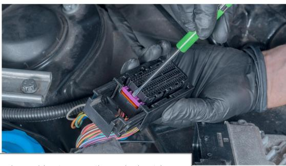
Use a small flathead screwdriver to remove the purple pin retainer clip from the harness. You can remove it completely from the harness and set it aside.
