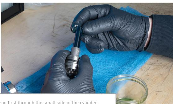
Insert pin small end first through the small side of the cylinder. Push until the tip of the pin has clearance to insert the retainer. NEVER install the opposite direction or seal damage will occur.
