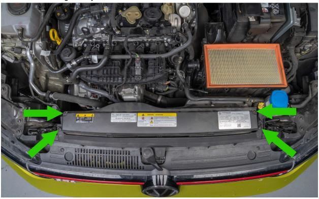
Push down on both mount tabs to release the air filter inlet from the radiator support.
