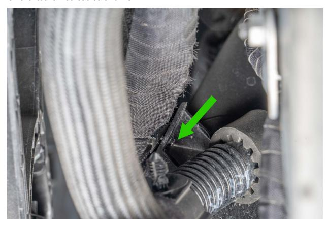
Use a flathead screwdriver to release the band clamp from the coolant hose.
