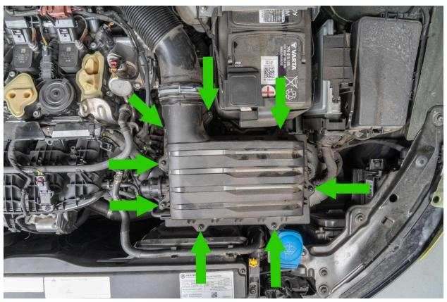
Remove the secondary air hose from the intake box by pinching both sides of the connector. Simply pull to remove the vacuum line from the air box.
