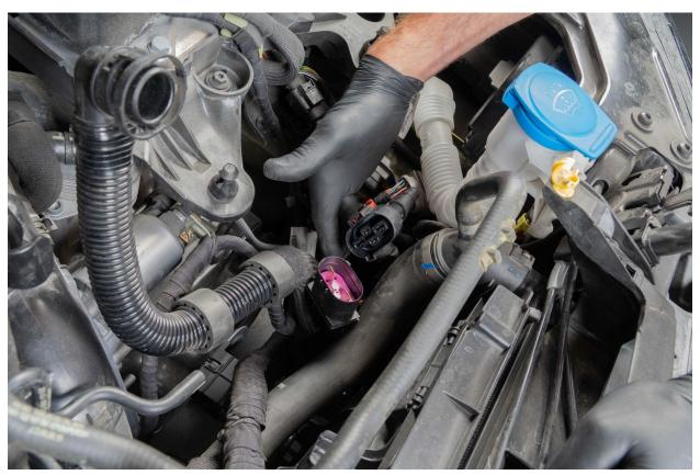
Disconnect the final wiring loom clip from the turbo outlet pipe with a flathead screwdriver. Remove the upper outlet pipe mount bolt with a T30 torx driver.
