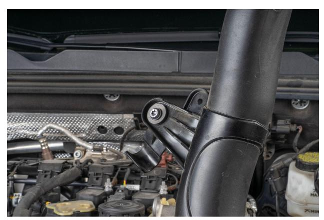
Pictured below are the rubber grommets and bolts in place on your IE Turbo Outlet Pipe
