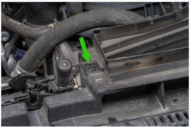
Remove the lower portion of the intake inlet.
