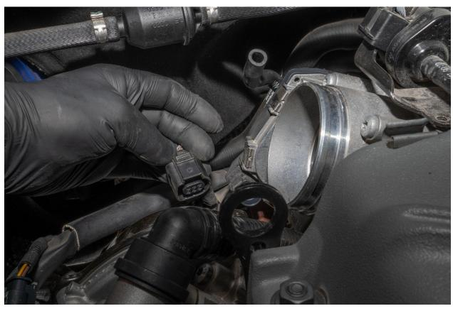
Release connector lock and remove it from the purge valve
