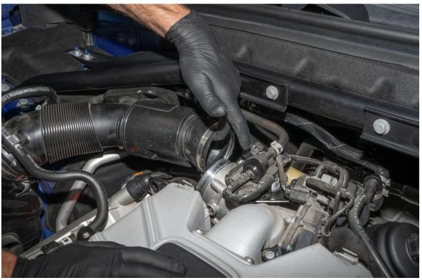
Remove vacuum line on the back side of the throttle body
