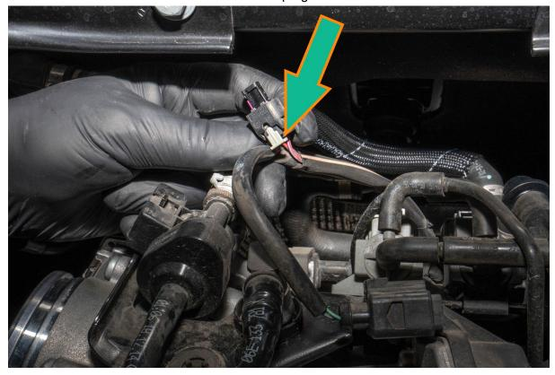
Remove purge valve to supercharger hose by pressing and releasing tabs on the side
