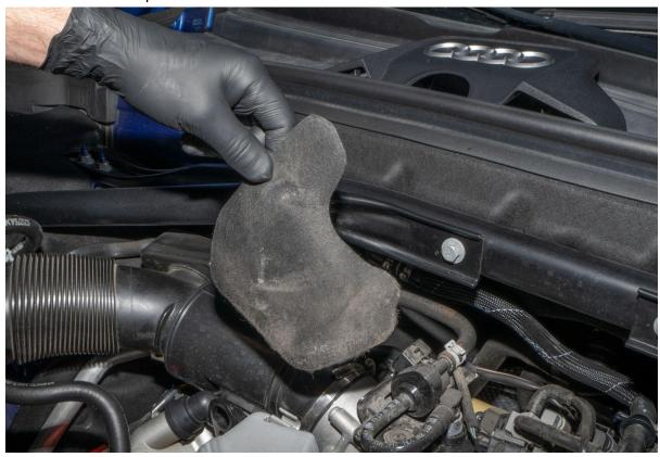
Remove throttle body pipe hose clamp with a flathead
