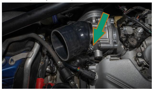
Reconnect evap purge valve and install connector
