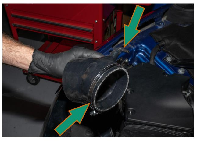
Install silicone coupler and tighten hose clamp
