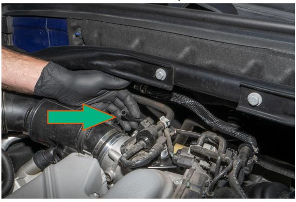
Remove throttle body pipe from throttle body and air box
