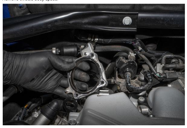
Place gasket onto throttle body spacer and install for 5mm Allen bolts in throttle body adapter
