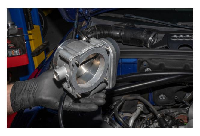
Install throttle body and tighten four 5mm Allen bolts
