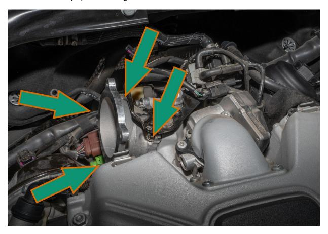
Place throttle body gasket on throttle body, and install four 5mm Allen bolts
