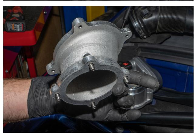
Install throttle body spacer and tighten the four 5mm Allen bolts
