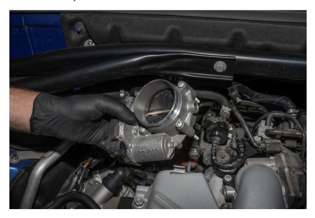
Remove throttle body spacer
