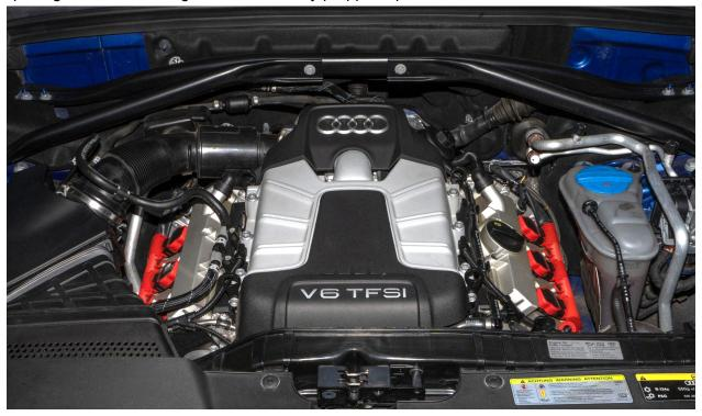
Remove upper engine cover by pulling straight up
