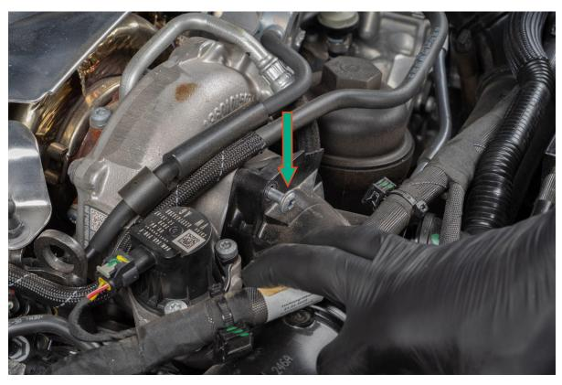
Remove bottom T27 inlet screw by using a stubby socket and an extension, then remove the lower EVAP hose by pinching on both sides and pulling down.
