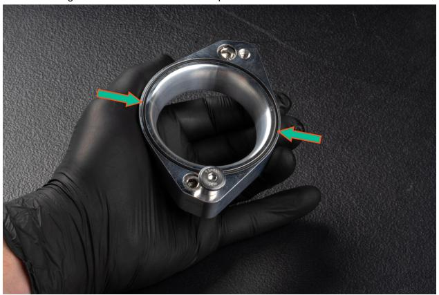
Install the inlet adapter to the turbo. Take care not to drop or pinch the o-ring between the turbo and inlet adapter, then slide the IE inlet onto the aluminum retainer post as shown. (*shown-off vehicle for clarity*)
