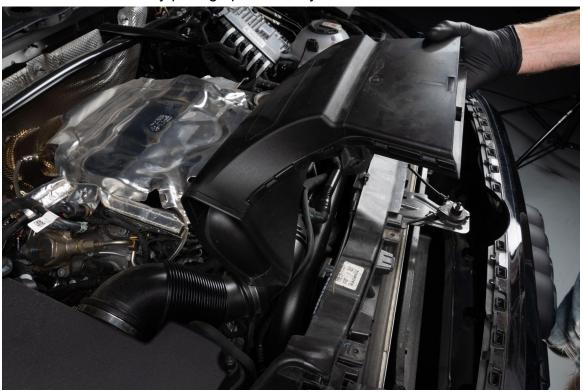
Loosen air box hose clamps using flat head screwdriver
