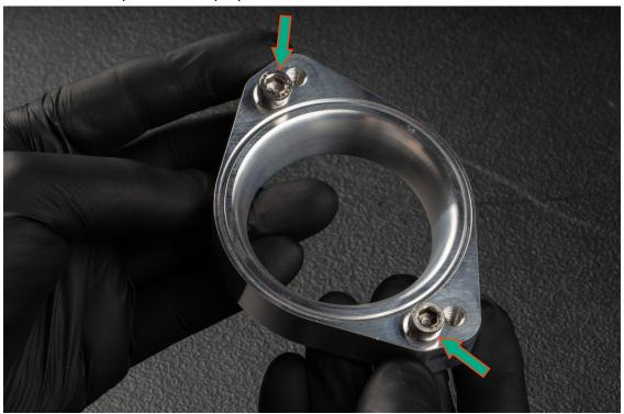
Install the retainer post by using the 25mm flat head 4mm screw
