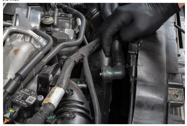
Back out the top T27 screw from inlet using T27 Socket.
