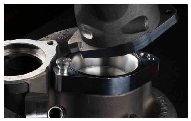
Use the button head screw to attach the inlet to the adapter.
