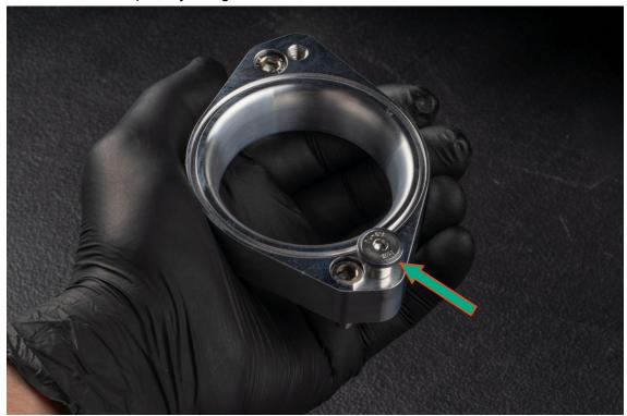
Install the o-ring on the front side of the inlet adapter.
