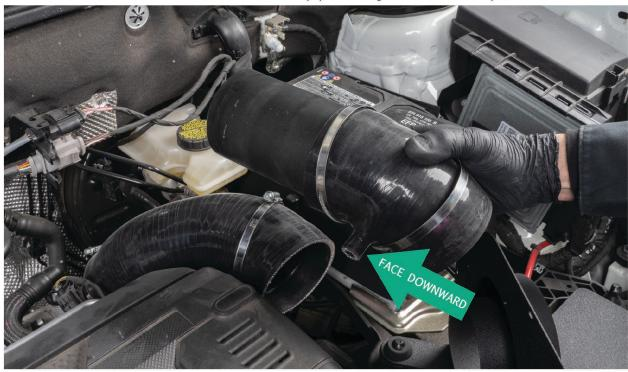
Install hard pipe and silicone elbow assembly to inlet silicone and heat shield. Point the vacuum hose hole downward.
