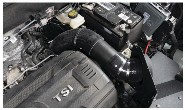
Insert vacuum hose elbow into vacuum hose, then insert into bottom of intake silicone elbow.
