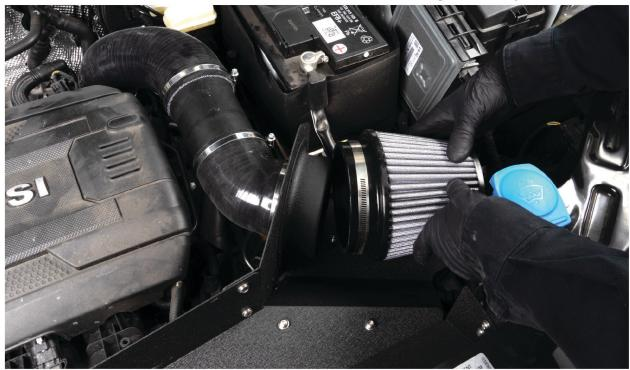
Ensure the heat shield is not binding on any plastic pieces by aligning properly, then tighten all Allen bolts to secure in place.
