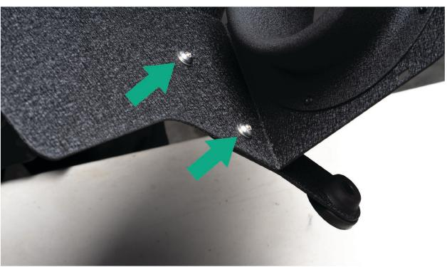
Using Four 4mm Allen bolts and Four Washers, attach two L shaped mounting brackets loosely on the outside of the scoop portion of the heat shield. One Bracket has a longer top length. That bracket will be on the driver's side of the vehicle.
