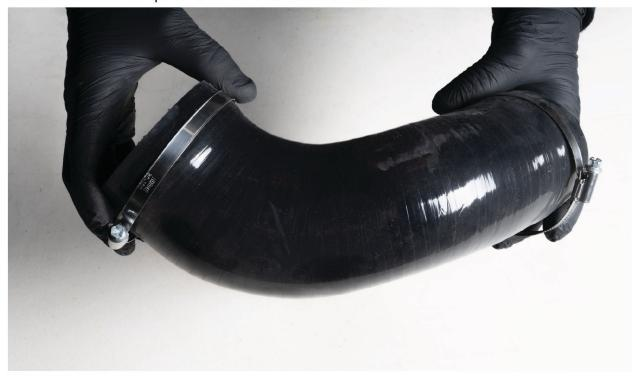
Install inlet silicone hose to turbo inlet.
