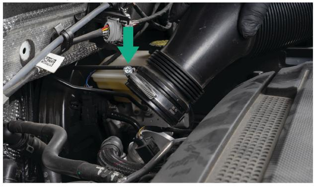
Remove the top portion of the Airbox and inlet pipe.
