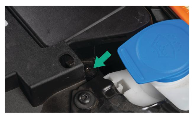
Pull Lower Air-box up to release from mounting pin, and remove air-box and scoop from vehicle.
