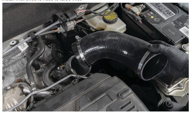
Install heat shield silicone elbow onto hard pipe, using two hose clamps.
