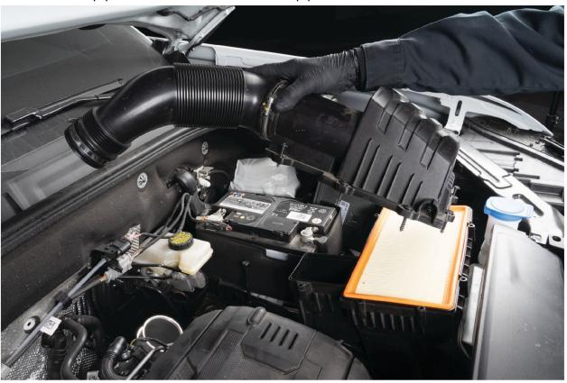
Remove Two T25 screws from each side of the Air-box Inlet Scoop.
