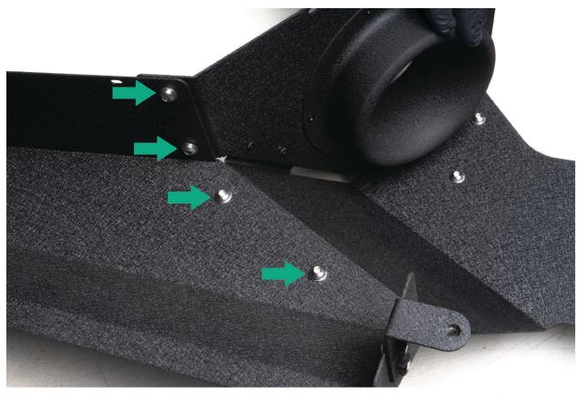
Install assembled heat shield into the engine bay. Align the two bolt holes with the two holes in the factory intake scoop.
