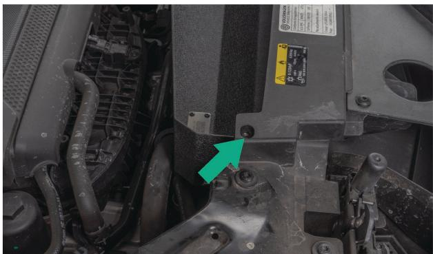
Then press mounting grommets located on the bottom of the heat shield onto alignment posts.
