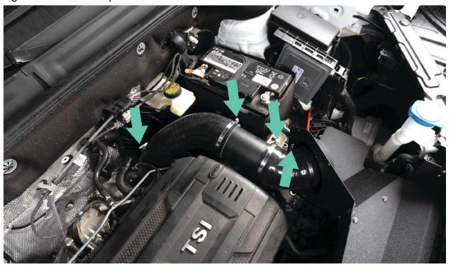
Install Air Filter onto intake bellmouth inside heat shield and tighten clamp.
