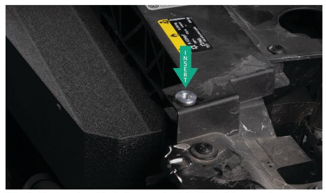
Using the Two long 4mm Allen bolts, secure heat shield to radiator support.
