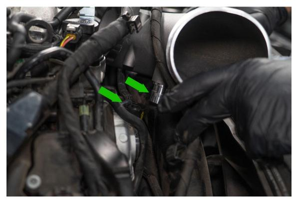
Reinstall upper breather hose onto the machined barb.
