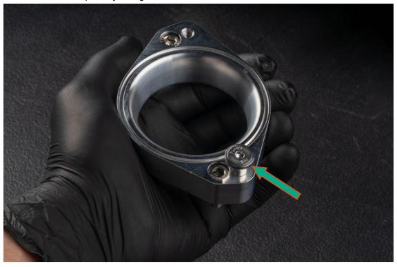
Install the o-ring on both sides of the inlet adapter.
