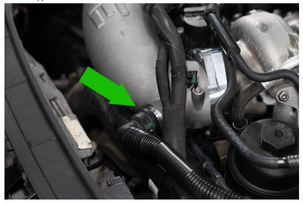
Reinstall Carbon intake. Space is tighter with the upgraded inlet. We recommend putting painter's tape on the inlet to help minimize the chance of scratching the airbox. To fit the carbon box without scratching it. First, turn the intake roughly 90 degrees towards you, then insert the pointed end of the intake into place.
