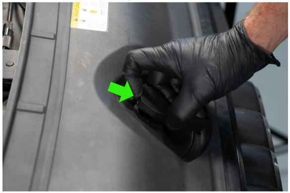
Remove the plastic radiator cover by pulling up on the front edge, then pulling straight towards the front of the vehicle.
