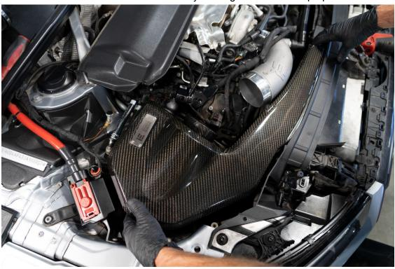
With the turbo inlet and the intake in place, reinstall the radiator Allen bolts, silicone elbow, hose clamps, radiator cover, hood latch, and engine cover. Enjoy your new IE Turbo Inlet Pipe!
