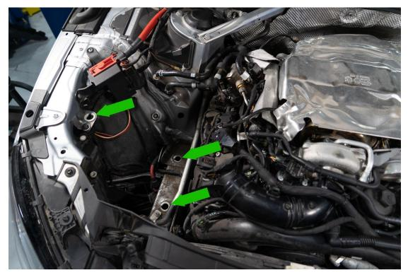
Remove the wire loom clips by pulling them up.
