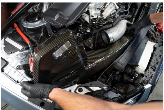
Then lower the air box while simultaneously twisting it back into the proper orientation.
