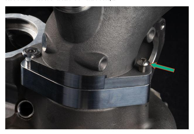
Install lower breather hose on the machined lower barb. Press until fully seated. It will click when properly in place.
