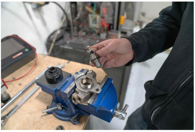
Assemble your IE Pump Internals by first putting the barrel into the HPFP seal housing. Push the pin up (do not install the pin downward) through the seal housing.
