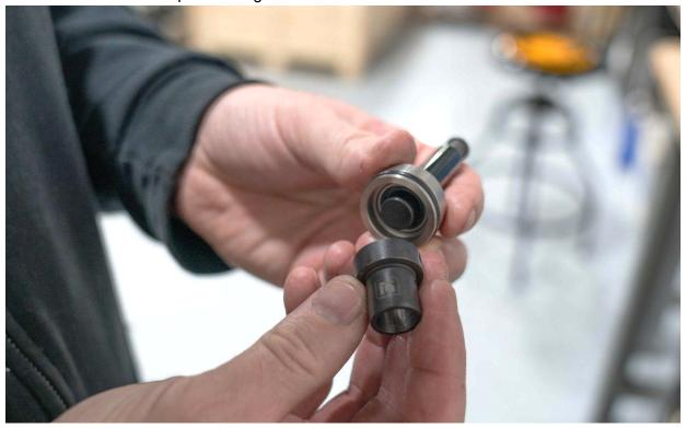
Place the pump internals inside pump housing.
