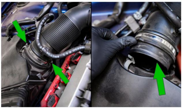
Pull back on the airbox to disconnect it from the fender bracket, then pull up to disconnect the box from the lower grommets. *Do not completely remove the airbox in this step.*
