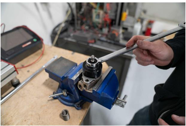
Remove the retaining nut from the housing.
