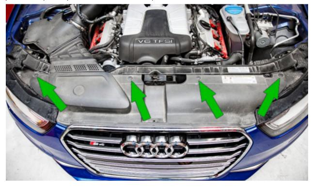
Carefully pull up on the edges of the cowl to release it, remove it from the vehicle and set aside.
