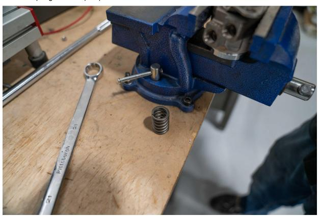
Place IE HPFP disassembly tool on the retainer nut.
