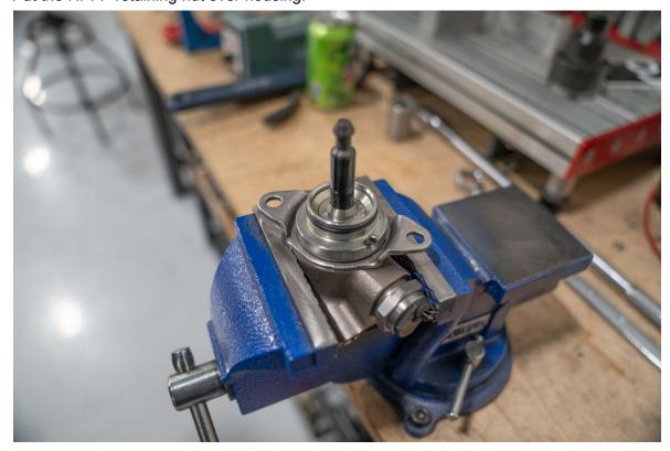
Use a Torque wrench and a 21mm deep socket with the assembly tool to tighten the retaining nut to 40 ft/lbs.
