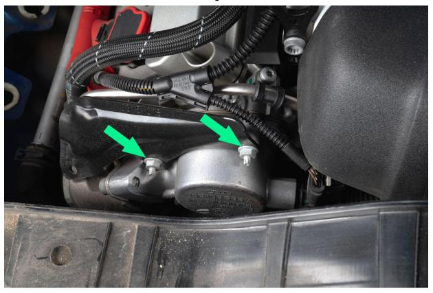
Remove shield from above the HPFP housing.
