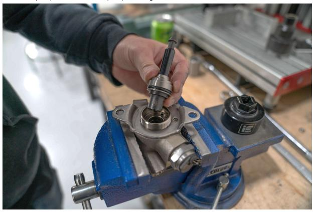
NOTE: If the pin comes all the way out of the seal housing, disassemble the entire housing and reassemble. If not disassembled, there is a potential to cause damage to the seal which voids warranty and will allow gas to pass through to your oil
