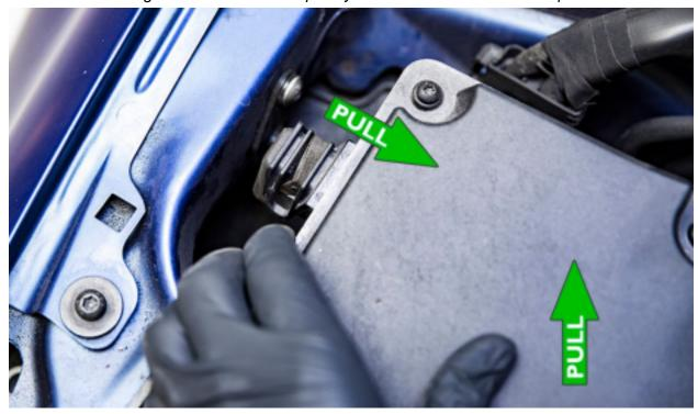
Carefully pull the airbox up and disconnect the SAI (secondary air injection) hose from the underside of the airbox. Remove the airbox completely.
