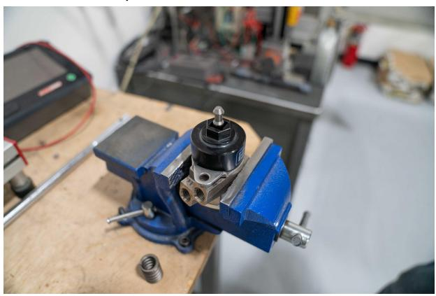
Use a 21mm wrench to loosen the HPFP retaining nut.
