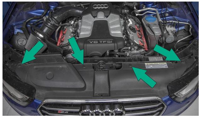
Remove the cowl carefully by pulling upwards.
