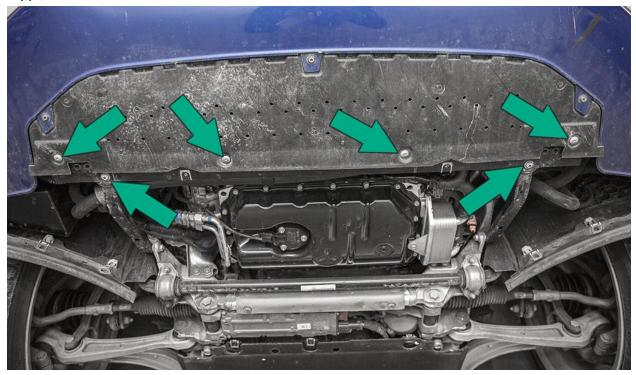
Remove the two 10mm nuts from the axel guard and let it sit disconnected. *Repeat this step on both sides of the car.*
