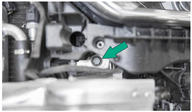
Remove the lower crash beam to radiator support bolts with a 16mm socket, two located on each side. *Note: We highly recommend installing a 10mmX1.5 threaded bolt at least 60mm in a lower hole on each side to support the weight.*
