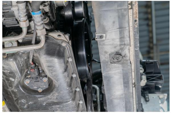
Tighten and torque all bolts using a 6mm allen bit to 20nm + 90 degree turn.
