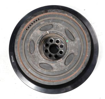
Once the offset holes are aligned, mark the IE pulley with a paint pen in the same location as your paint mark on the factory pulley, so you know which side of the pulley needs to be facing directly up.
