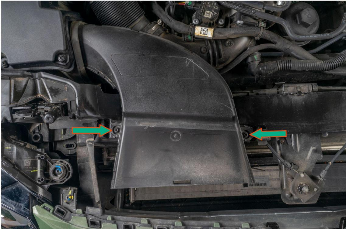
Remove Intake Scoop from Air Box by pulling straight away from Air Box
