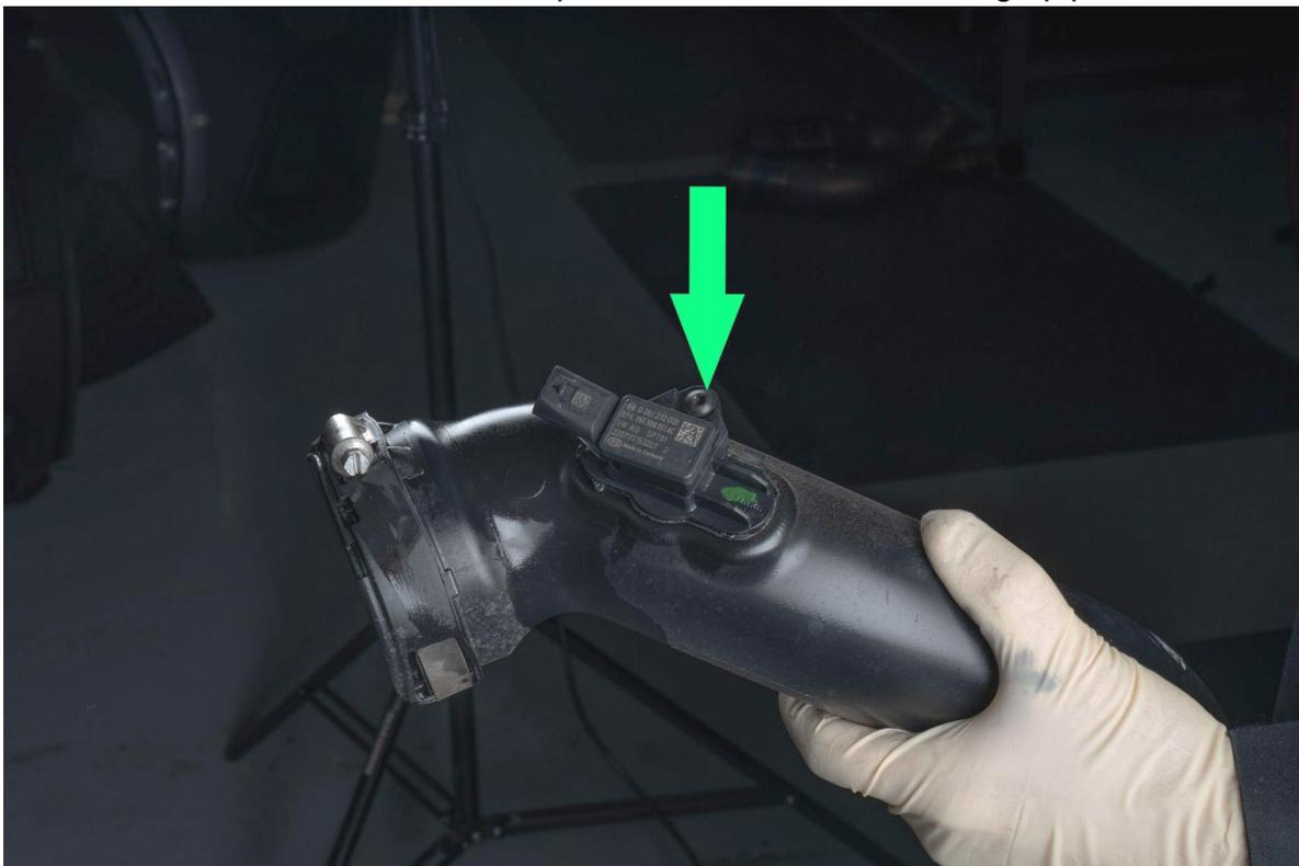
Install map sensor into new IE charge pipe using a 4mm button head screw
