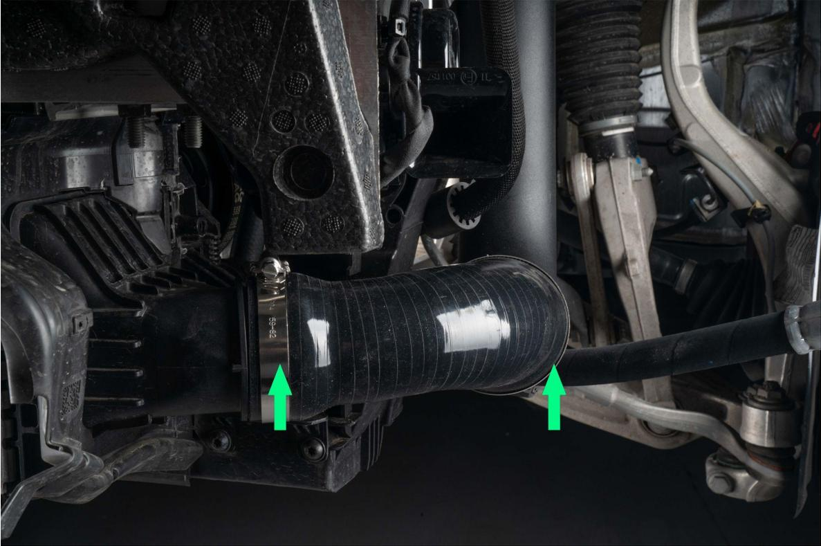
Remove three T30 screws connecting the charge pipe to the intake manifold
