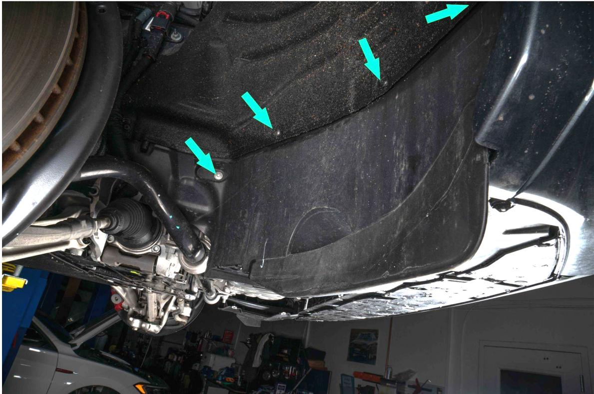
Remove headlight vent from fender liner, and remove fender liner
