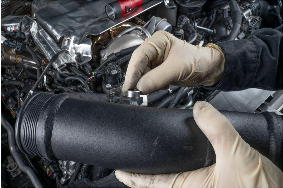
Connect the silicone to passenger side charge pipe
