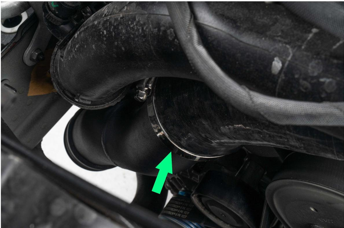
Loosely install hose clamps onto the silicone
