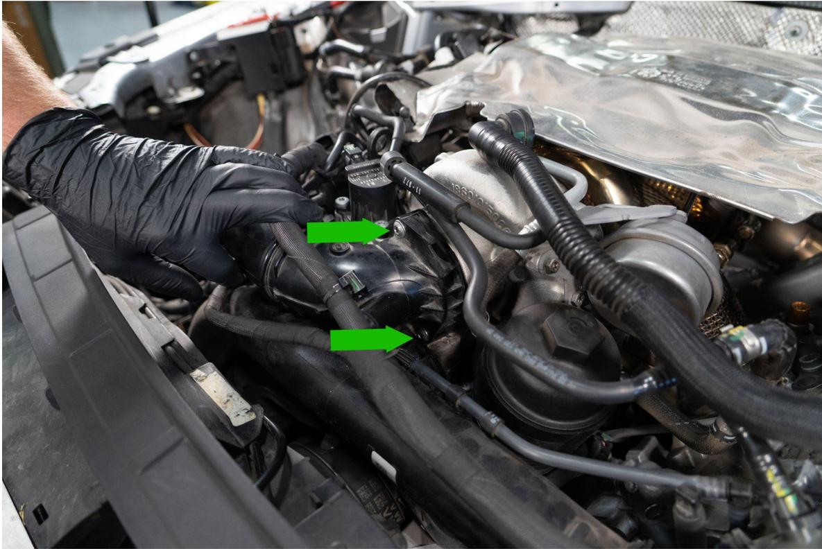
Remove the lower breather hose by pushing both sides of the release tab and pulling down and away from the turbo inlet. You can now remove the factory turbo inlet from the vehicle.
