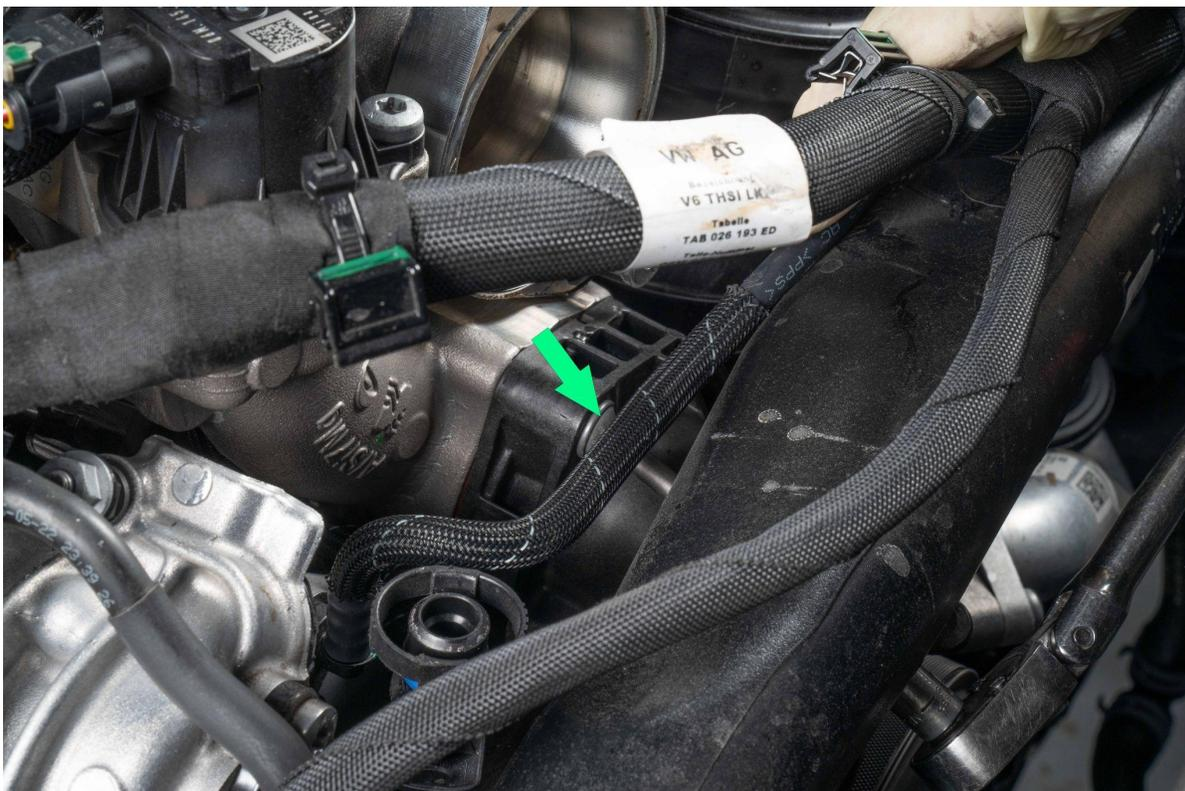
Remove three T30 screws from the driver side of the intake manifold
