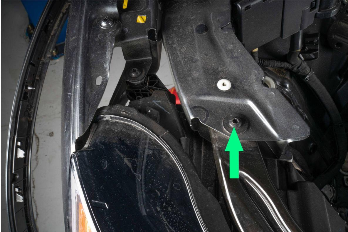
Remove the wiring harness fastener by pressing up with a flathead away from the connecting point.
