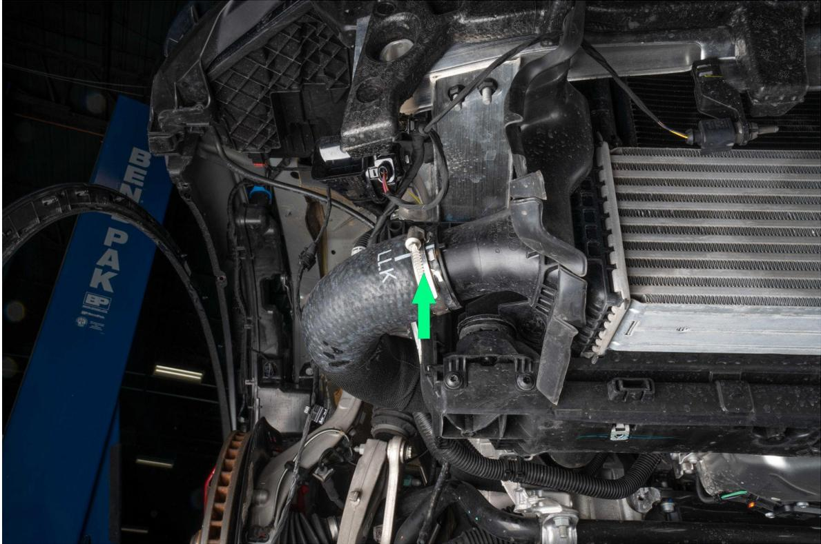
Remove charge pipes from intercooler
