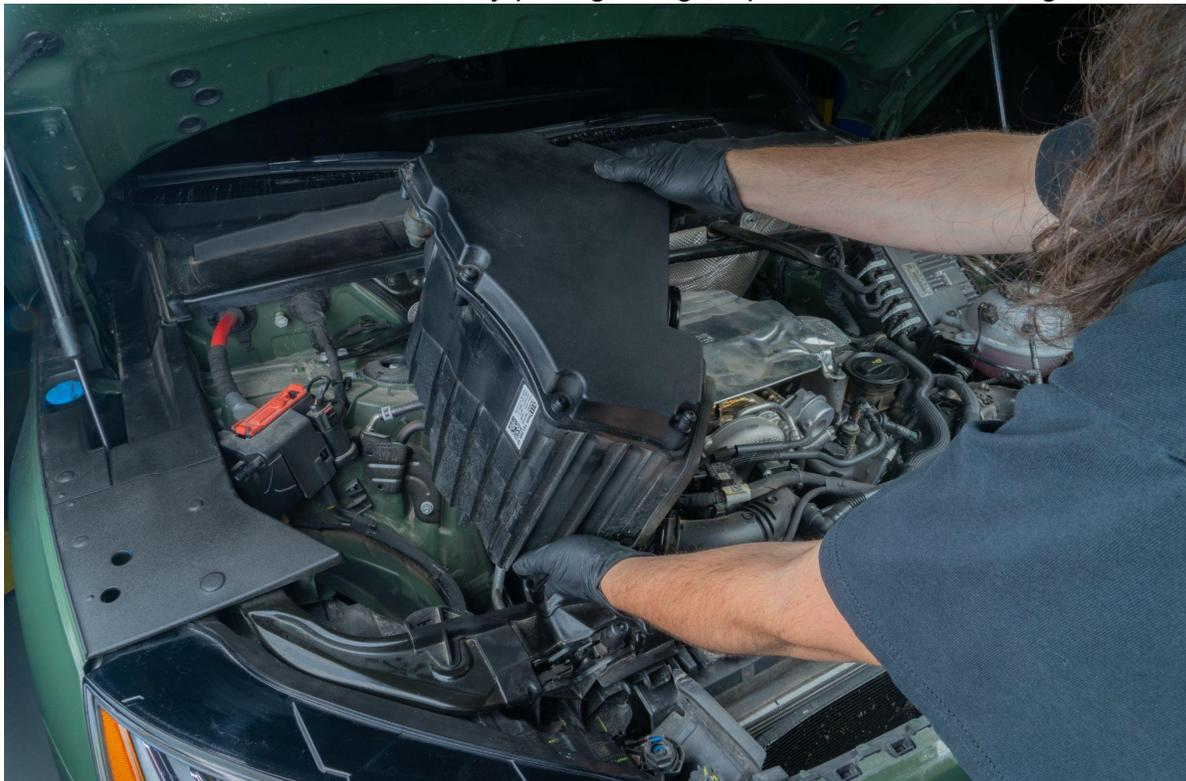
To remove the factory turbo inlet, start by removing the wire loom clips by pulling them up off the turbo inlet.
