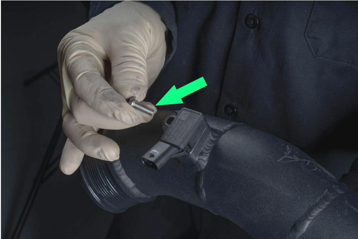
Install silicone connector hose at the end of the charge pipe and tighten hose clamp
