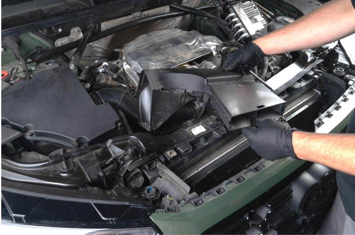
Loosen the two band clamps around the intake tube with flathead screwdriver
