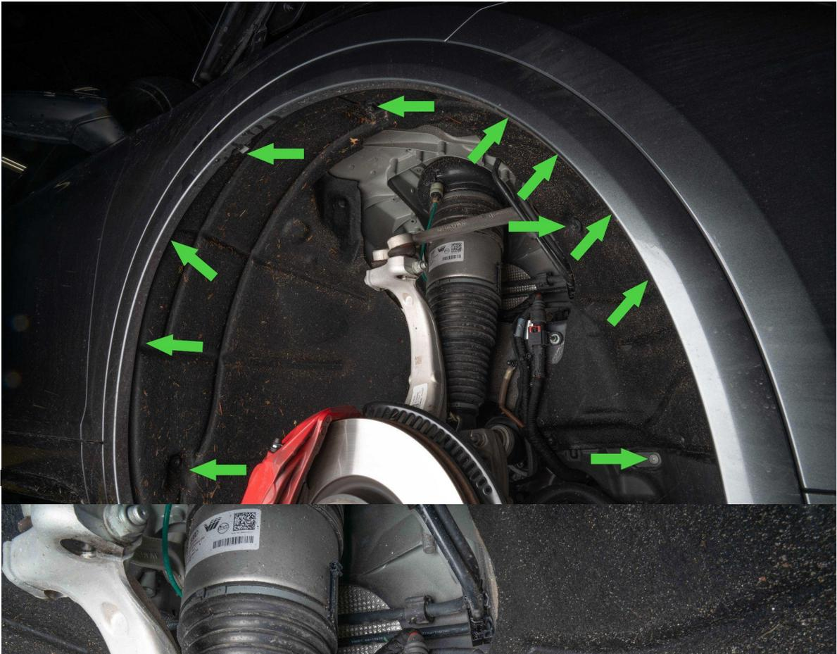
Remove 5 press in retainers from the fender and front bumper starting at the bottom of the wheel well and going up.
