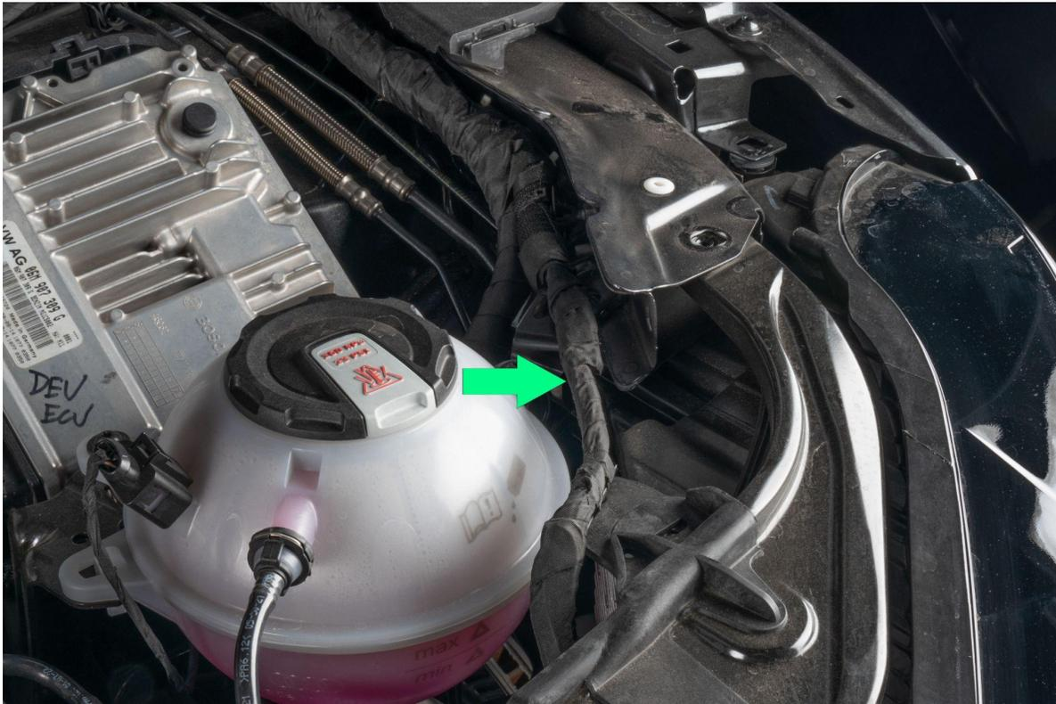
Remove #10 triple square and T30 from lower radiator support bracket
