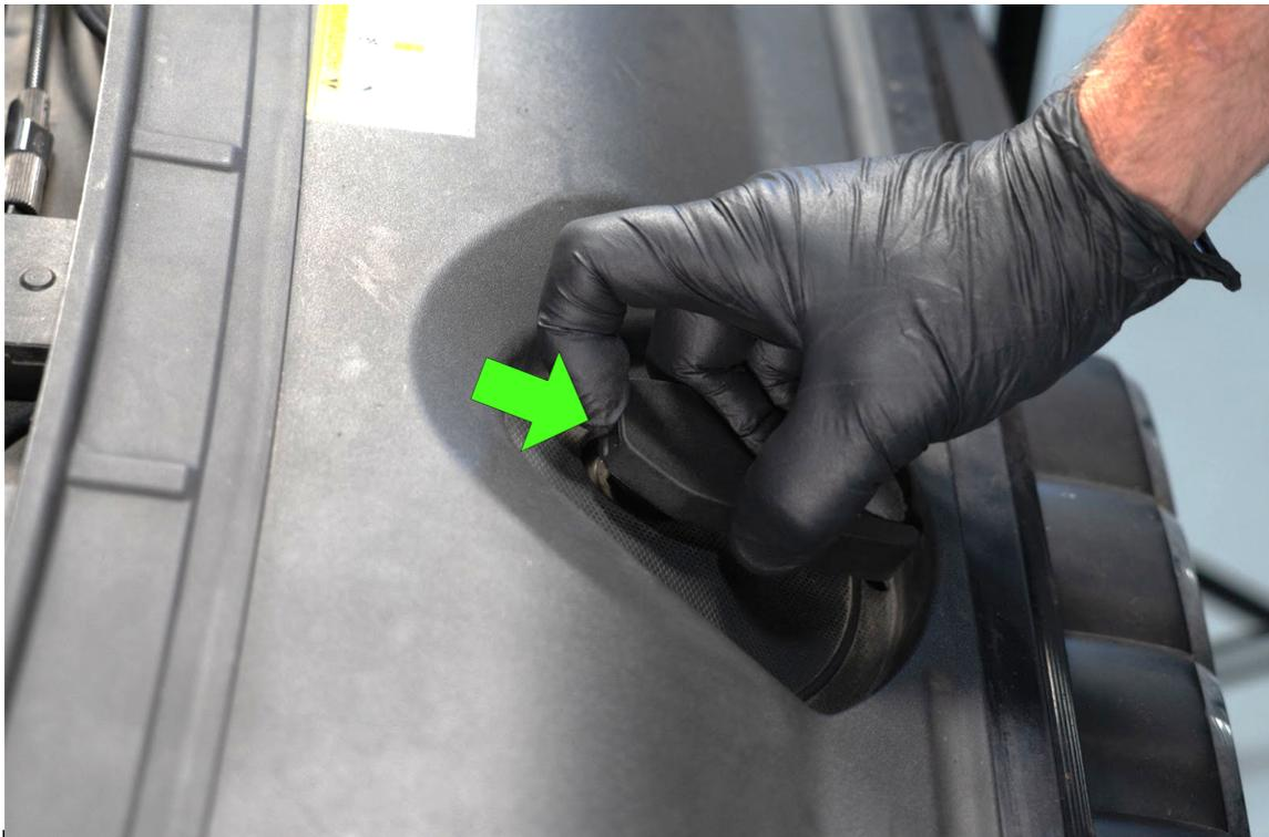
Remove plastic radiator cover by pulling straight up on the front edge. Once all front clips have been released, pull straight towards the front of the vehicle to remove.
