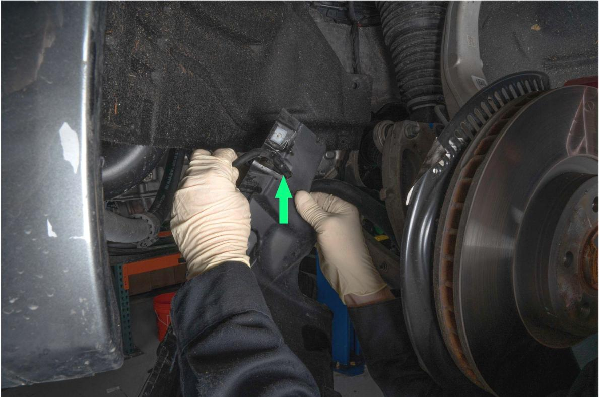
Remove 3 T25 screws, 6 10mm plastic nuts and 2 push in retainers and remove fender liner
