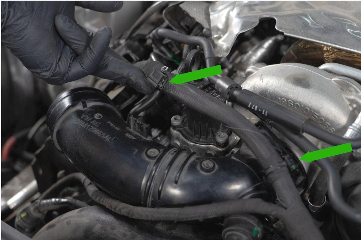
Remove the front breather hose by firmly pulling straight towards the front of the car.
