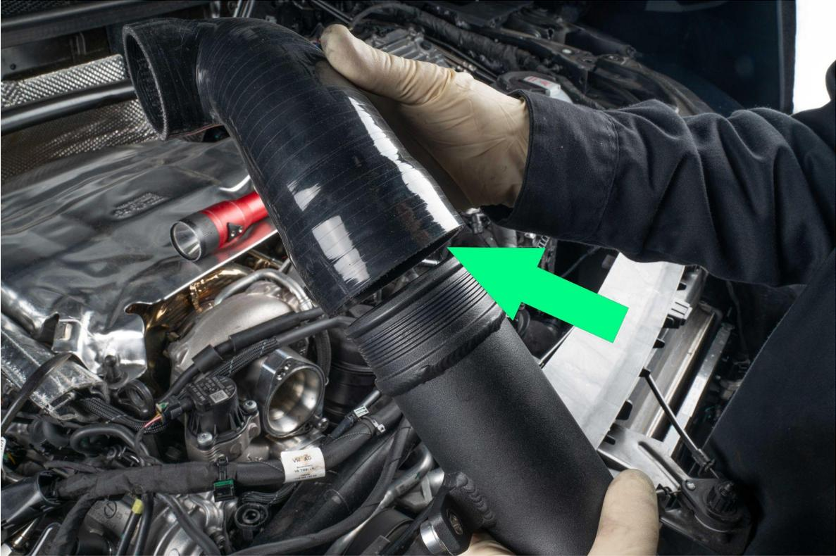
Loosely install the band clamps onto the silicone ends and connect to the charge pipe
