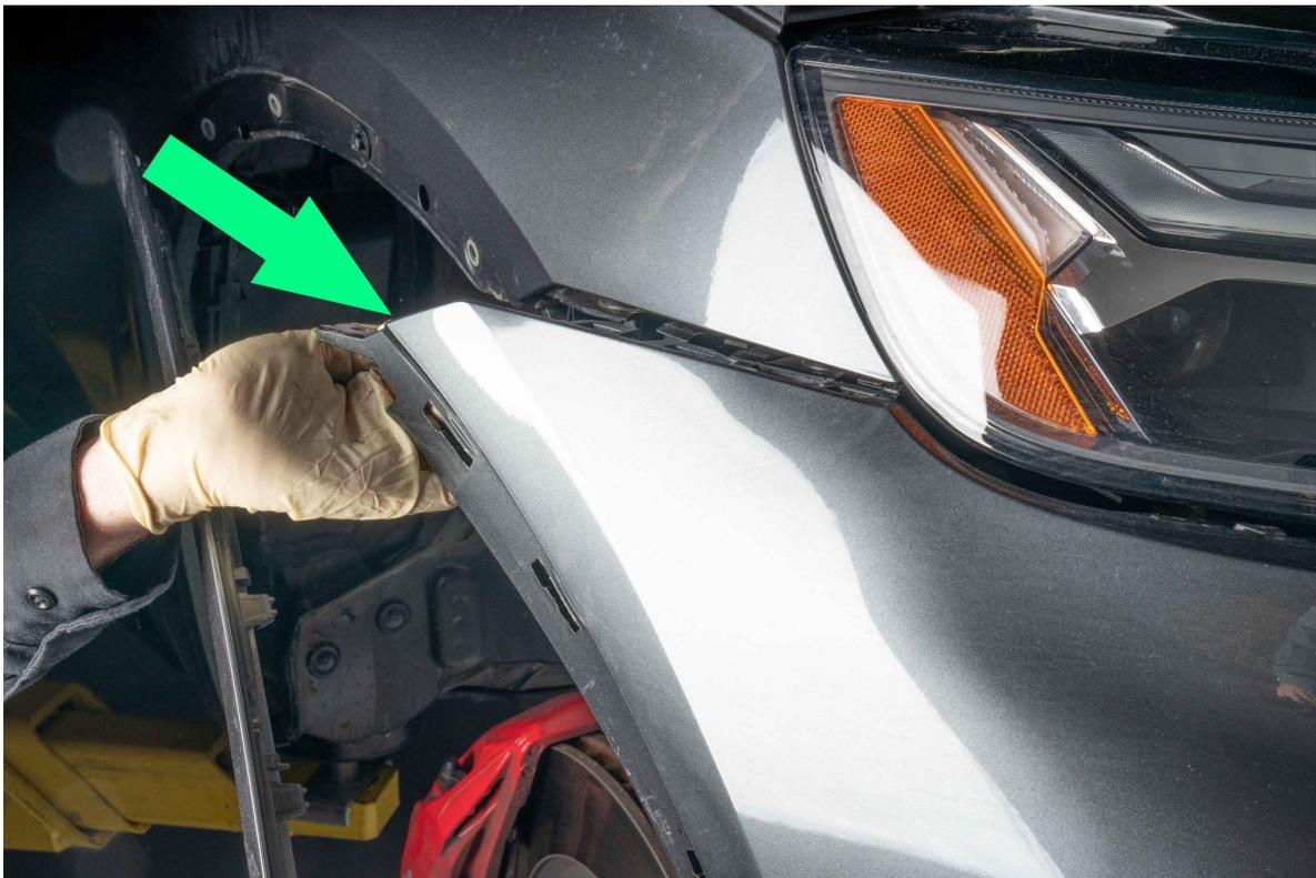
Remove 4 torx screws on the lower edge of the bumper
