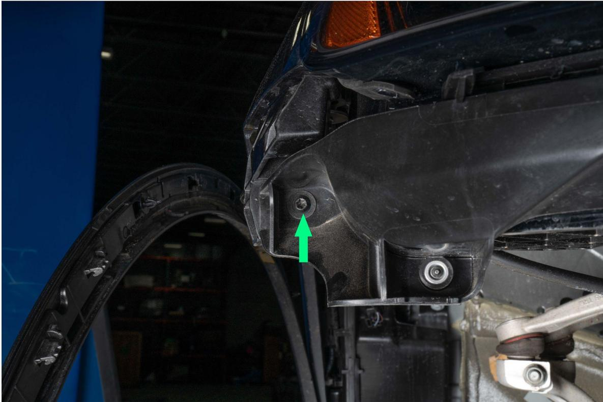
Remove plastic cover from both sides by pulling up from the corner.
