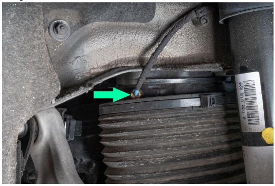
Once all of the air has been released from the bags, loosely tighten the 10mm nut and reinstall back wheels
