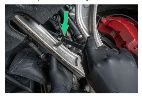
Open your supplied grease packet and apply some grease to the inside of both sides of the IE Link, then install new IE links to ride control by pressing firmly onto the OE mounting point.
