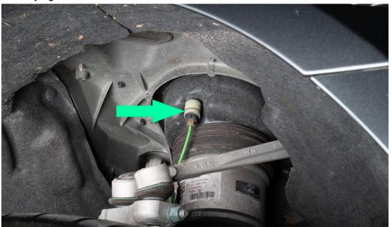
Once you have released the air from the front of the car, remove both rear wheels to gain access to the air bags
