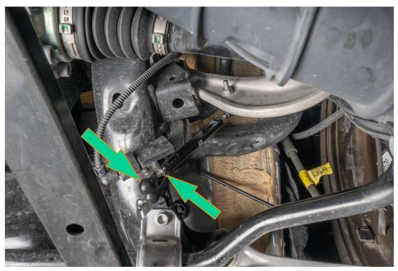
**Some vehicles may require an adaptation of the new links**. If either the rear or the front doesn't sit correctly after installation, Inside the front wheel wells in the upper shock you will see an airline that connects to a brass fitting. Using a 10mm wrench, loosen fitting until you hear air being released. After all the air is released, the air will stop. Loosely tighten the bolt after all the air is released.
