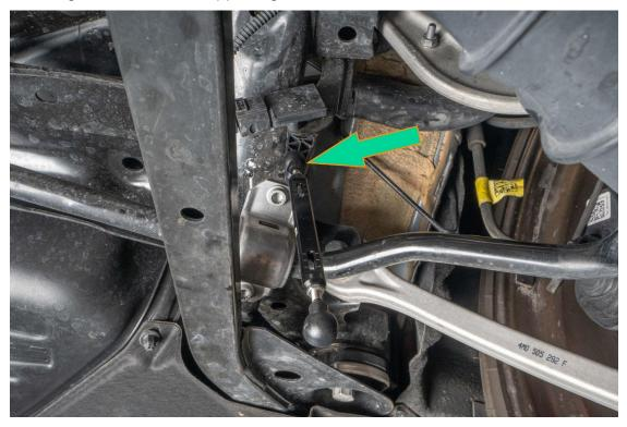
Attach the other side of the IE Link to the upper mounting point, then set desired ride height by twisting the body of the IE Lowering Link. Then tighten the locking nut using a 5/16mm wrench. As before, ensure that the measurement settings match from side to side.
