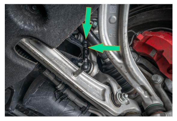
As before, lubricating the OE Link mounting points may help with removal.
