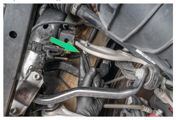
Apply grease to the inside of both sides of the IE link, then carefully attach new link to ride height sensor while supporting the sensor arm.
