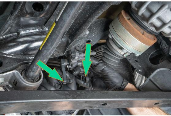
Lift up the link from the upper ball and remove.
