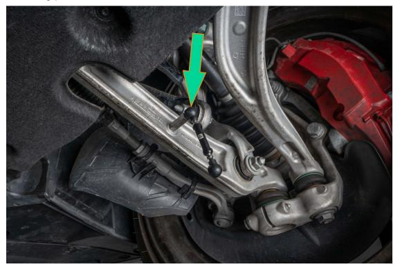
Support ride height sensor and press IE link into place, then set desired lowering point by twisting the body of the link. Once desired height is set, tighten the locking nut using a 5/16mm wrench. Ensure that the measurement settings match from side to side.
