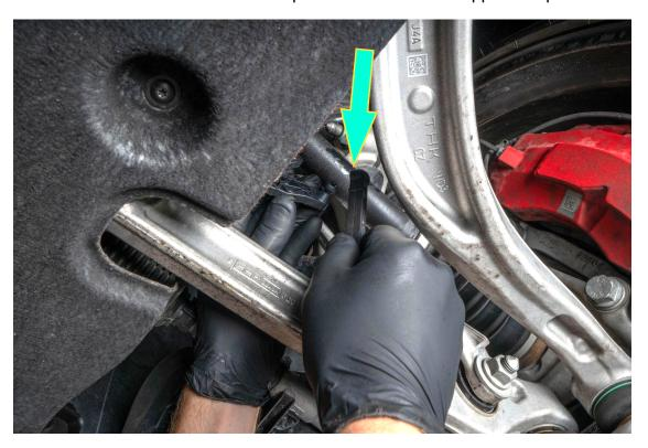
Rotate down and pry off of the pivot ball mounting point.
