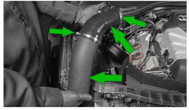
Install short silicone coupler and included hose clamps to the back of the velocity stack.
