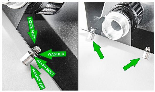
Assemble both of your intake heat shield parts as shown below with the included button head bolts and washers. Tighten firmly with a 4mm allen wrench.
