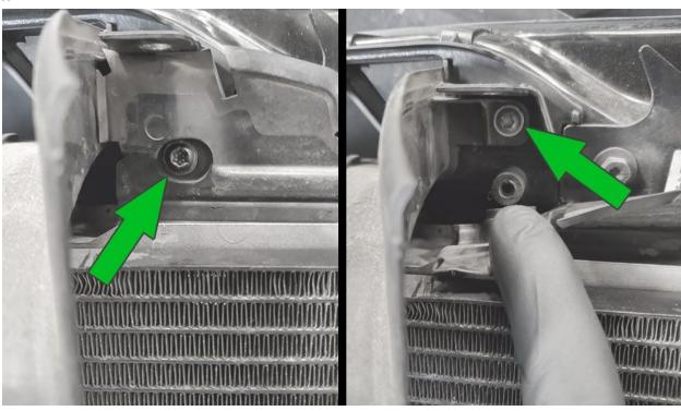
With a T25 torx, remove the second mounting screw from the radiator support on the left-hand side of the intake inlet.
