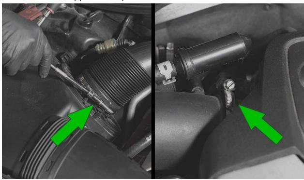
Remove the inlet pipe and both hose clamps from the vehicle.
