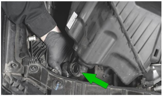
With the airbox completely disconnected, remove it from the engine bay.
