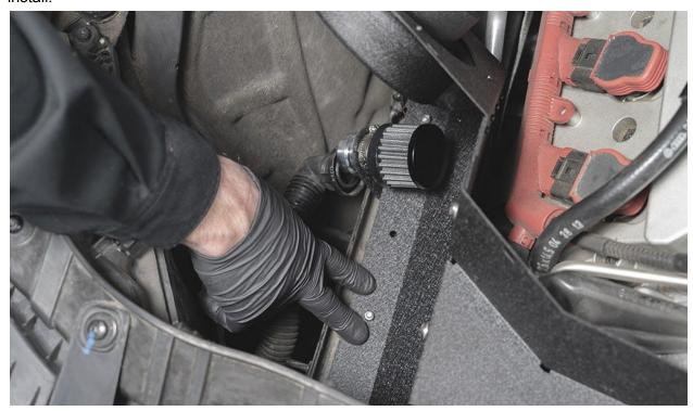
Press firmly to install the factory SAI line onto the new SAI adapter on the heat shield.
