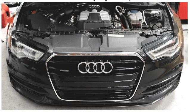
Remove two push clips from the radiator cowl. Use a small flathead to pull up the center pin of the clip, then pull to remove the entire clip.
