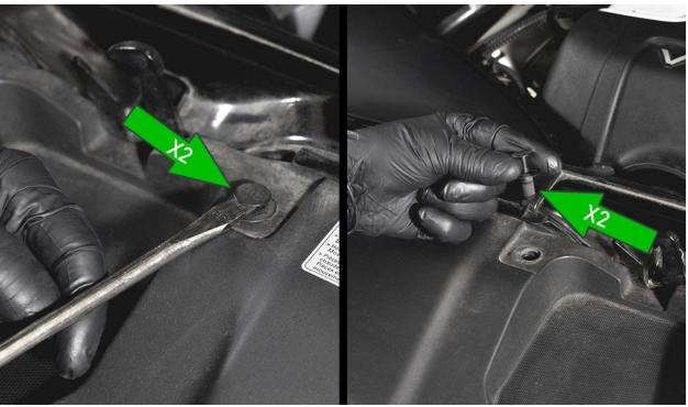
Carefully pull up on cowl clips to release it, then pull to remove from the vehicle, and set it aside.
