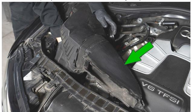
Insert the SAI adapter into the SAI bracket on the heatshield. Install the SAI filter and clamp onto the adapter, sandwiching the bracket then tighten the clamp with a screwdriver. The filter should be sitting facing the heat shield when installed.
