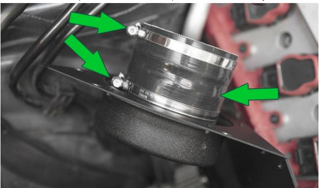
Install the hard pipe and silicone onto the throttle body and into the velocity stack silicone. Adjust inlet and silicone positions as needed, make sure nothing is pulling or bound and that it sits freely and without tension. Tighten all 4 clamps. *Do not overtighten hose clamps.*
