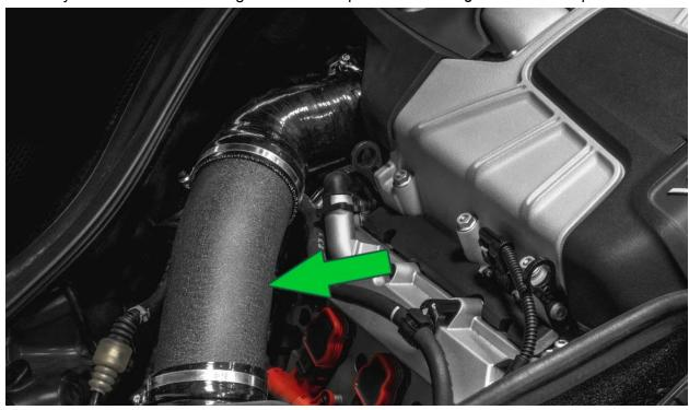
Push to install the factory vacuum line to the new IE inlet silicone. Optional: secure with a zip tie.
