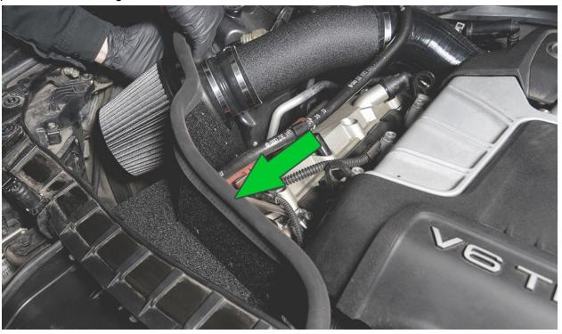
Re-install the radiator cowl and push clips. Verify all hose clamp connections are tight, and that your intake is fully installed. Start the car and inspect for any leaks or rubbing components.
