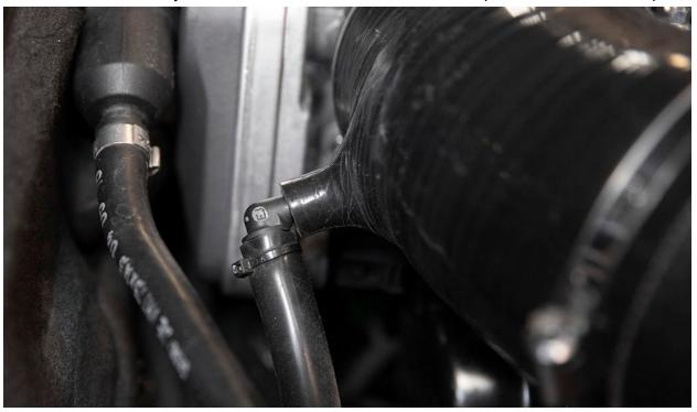
Install the air filter and clamp onto the velocity stack. For maximum horsepower output, make sure the IE logo on the filter is positioned in a legible position before tightening the hose clamp.
