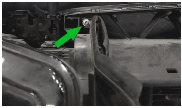
Pull up on the airbox to remove it from all the mounting grommets. Disconnect the factory SAI line from the bottom by depressing the lock ring and pulling it back. *Be careful not to break the plastic on your factory SAI line*
