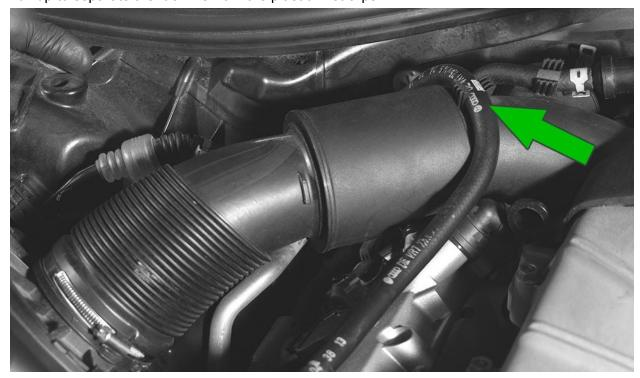
Loosen both hose inlet pipe hose clamps with a flat head screwdriver.
