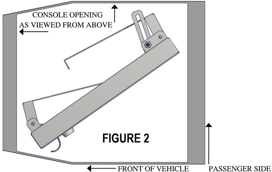
The Console Safe will need to rotate while being placed so that the lid/logo faces up. The fit is quite tight and may require a second effort at a slightly different angle. The Console Safe should now be resting on the bottom of the console with the logo facing up.
