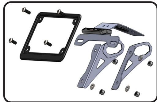
6. Install assembled fender eliminator using the stock fender bolts, *14720-SPR*, fender bracket spacer, and *8MMNUT*, 8mm flange nuts. Route license plate light and turn signal wires through *H-2158*, wire cover on fender eliminator bracket and through undertail. Torque bolts to factory specification.
