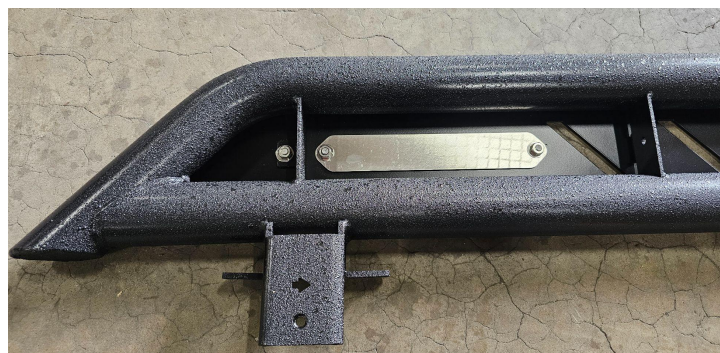
Detail B3: Assemble top plates and accent plates
