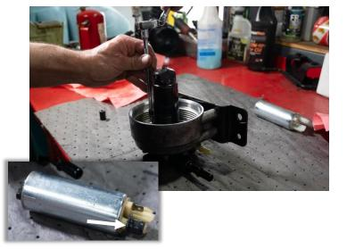
**STEP 10:** Remove the four bolts retaining the upper fuel filter assembly using a 10mm socket or wrench.
