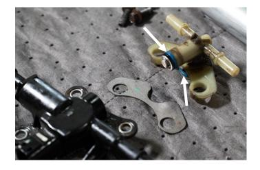
**STEP 15:** Using a 19mm socket or wrench, remove the plastic QD fitting on the side of the upper filter assembly. Remove the O-ring from the fitting.
