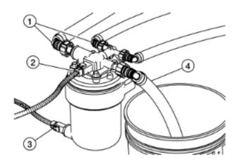
STEP 1: Connect a  $\frac{1}{2}$ " ID fuel hose to the supply outlet of the filter housing (4) of the fuel filter housing. Allow the open end of the  $\frac{1}{2}$ " ID hose to flow into a clean 5-gallon bucket.
