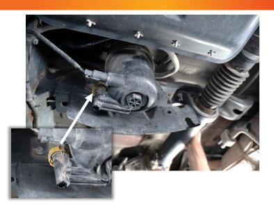
**STEP 3:** Disconnect the chassis harness connectors for the fuel pump power and the water-in-fuel (WIF) sensor. Using a 19mm socket or wrench, remove the WIF sensor from the lower fuel filter housing.
