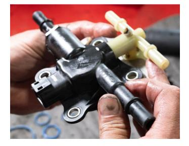
**STEP 20:** Lubricate with clean fuel or grease and install the new O-ring (item 2 in kit) onto the underside of the upper filter assembly.
