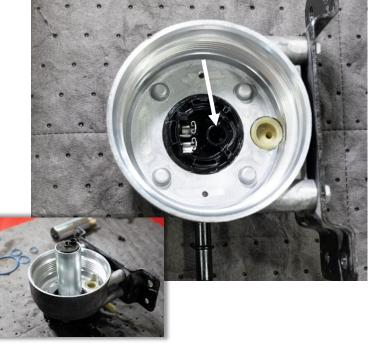
STEP 27: Install the filter and pump assembly onto the vehicle. Using a 12mm socket or wrench, install the two nuts and two bolts to retain the filter and pump assembly.
