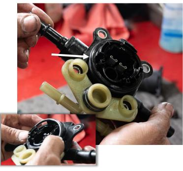
**STEP 23:** Install the pump into the underside of the upper filter assembly. The outlet of the pump will insert into the hole shown at right. Line up the electrical connectors with the terminals on the upper filter assembly. Carefully press the pump into place until fully seated.
