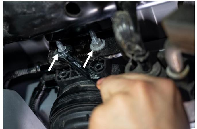
**STEP 6:** Install the Fleece Performance fuel filter base onto the mounting bracket, utilizing the two included M8-1.25 bolts. Using a 13mm socket or wrench, install the bolts through the mounting bracket and into the filter base assembly. Torque the bolts to 10 ft-lb.
