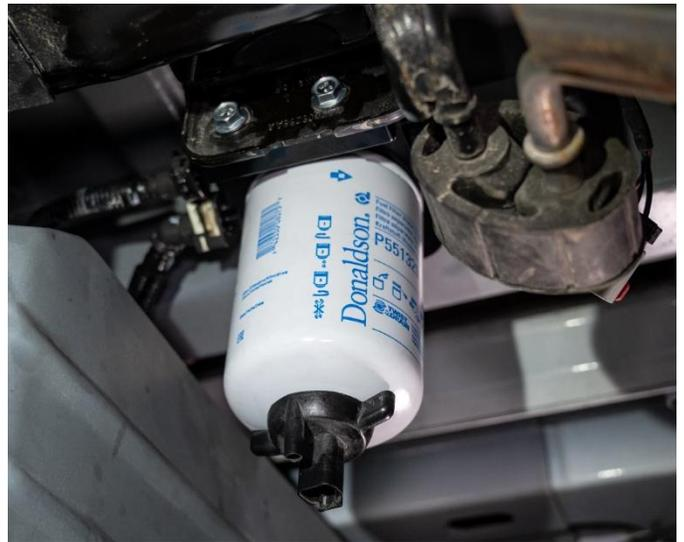
**STEP 11:** Connect the WIF sensor extension harness to the truck-side connector and the WIF sensor on the bottom of the fuel filter.
