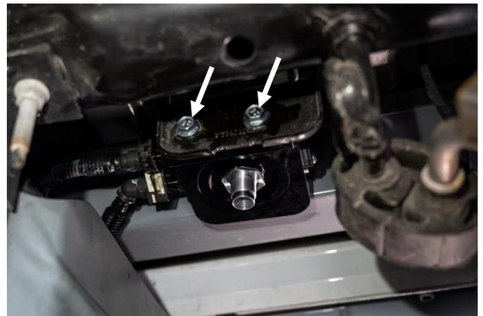
**STEP 7:** Connect the quick disconnect fuel line fittings to the adapter fittings on the Fleece Performance filter base. Once the fittings are connected, engage the locking tabs by pressing them into the fittings until seated.
