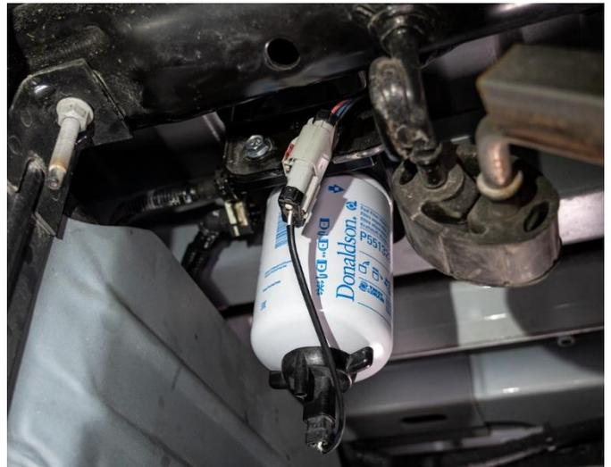
**STEP 12:** Connect the batteries. Prime the fuel system by cycling the ignition to the “on” position (without starting the vehicle) and wait for 5-6 seconds. Cycle the ignition to the “off” position. Repeat this process 2-3 times, then start the vehicle. Check for fuel leaks.
