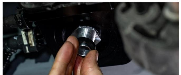
**STEP 9:** Remove the water drain adapter pre-installed on the bottom of the included Donaldson fuel filter. Turn the adapter counterclockwise to remove. Install the included water-in-fuel (WIF) sensor and water drain onto the bottom of the filter. Turn the WIF sensor clockwise until tight.
