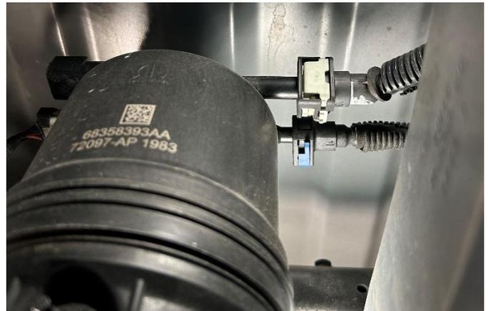
**LOCKING TAB #1** – This lock is white or gray in color. To disengage the locking tab, spread the two tabs outwards from the center of the fitting. With the tabs spread, push the ends of the tabs inwards towards the middle of the fitting (towards the right in the image shown). Pull the fitting from the filter housing to disconnect.
