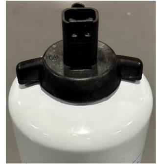
**STEP 10:** Lubricate the sealing O-ring on the fuel filter with fresh fuel. Install the filter onto the filter base. Twist the filter clockwise until tight.
