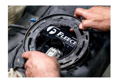
**STEP 15:** Install any necessary fittings provided with your aftermarket lift pump onto the SureFlo sending unit. See the image at right for connections on the cap of the SureFlo sending unit. Connect your factory fuel return fitting onto the unit.
