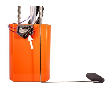
**STEP 13:** Place the included tank flange O-ring onto the tank flange. Carefully install the new SureFlo sending unit into the tank in the orientation shown at right.
