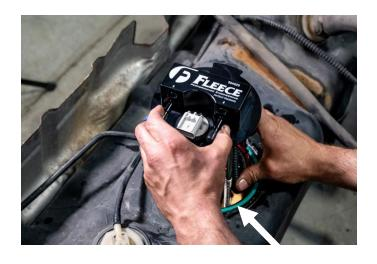
**STEP 14:** Install the locking ring back onto the tank to retain the sending unit assembly. Using a hammer and punch or chisel, turn the ring clockwise until fully seated.
