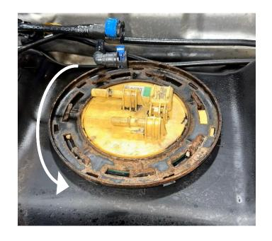
**STEP 12:** Install the included fuel level float arm onto the new Fleece Performance SureFlo sending unit by gently clipping the arm into the fuel level sensor.
