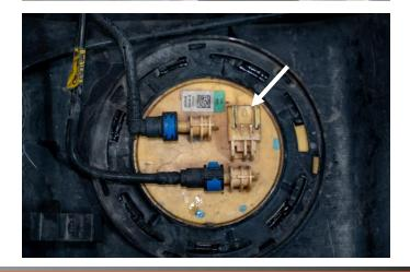
**STEP 7:** Lower the tank five to six inches and disconnect the electrical harness connector from the cap of the OE lift pump.
