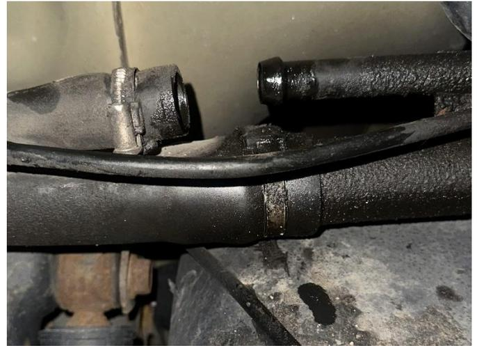
**STEP 4:** Disconnect the red fuel line quick disconnect fitting near the front of the fuel tank. To disengage the locking tab, spread the two ends of the tab and push them into the fitting. Disconnect the fuel line.
