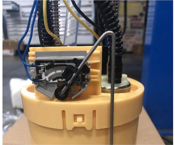
**STEP 13:** Place the included tank flange O-ring onto the tank flange. Carefully install the new PowerFlo lift pump into the tank in the orientation shown at right.
