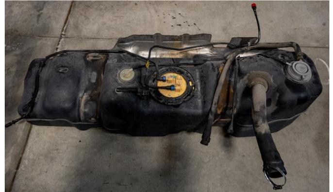
**STEP 10:** Disconnect the two quick disconnect fittings from the feed and return ports on the cap of the OE lift pump. See the identifying labels at right.
