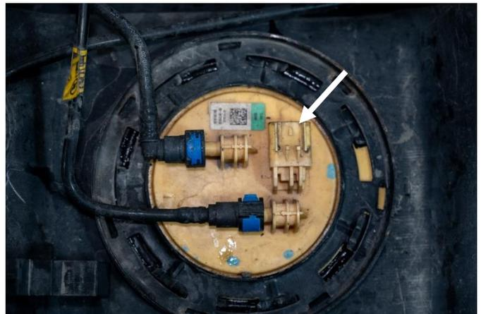
**STEP 9:** Thoroughly clean off the top side of the tank around the sending unit to avoid getting any debris inside the fuel tank when the OE unit is removed.
