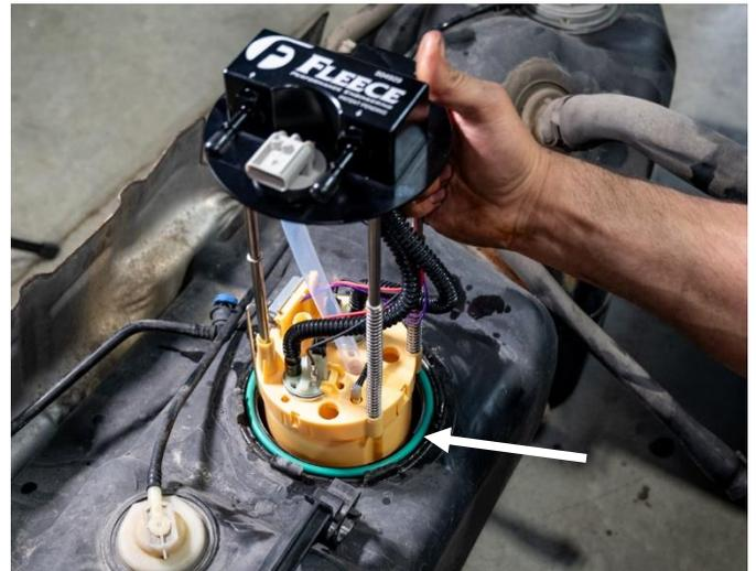
**STEP 14:** Install the locking ring back onto the tank to retain the lift pump assembly. Using a hammer and punch or chisel, turn the ring clockwise until fully seated.
