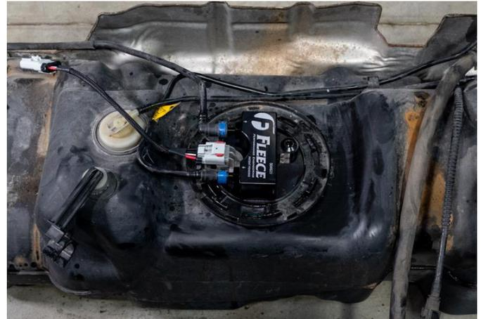
**STEP 16:** Place the fuel tank under the truck and onto a transmission jack. Lift the tank 5-6 inches short of its fully installed position and connect the adapter harness to the truck side lift pump connection.
