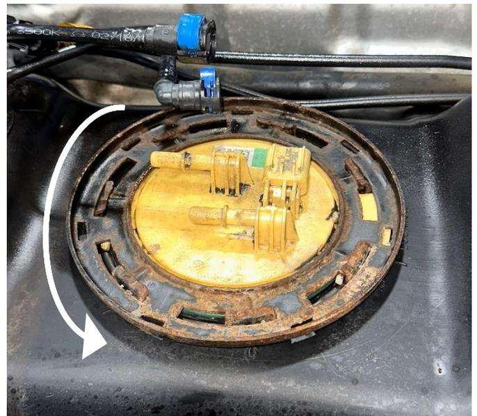
**STEP 12:** Install the included fuel level float arm onto the new Fleece Performance PowerFlo lift pump by gently clipping the arm into the fuel level sensor.
