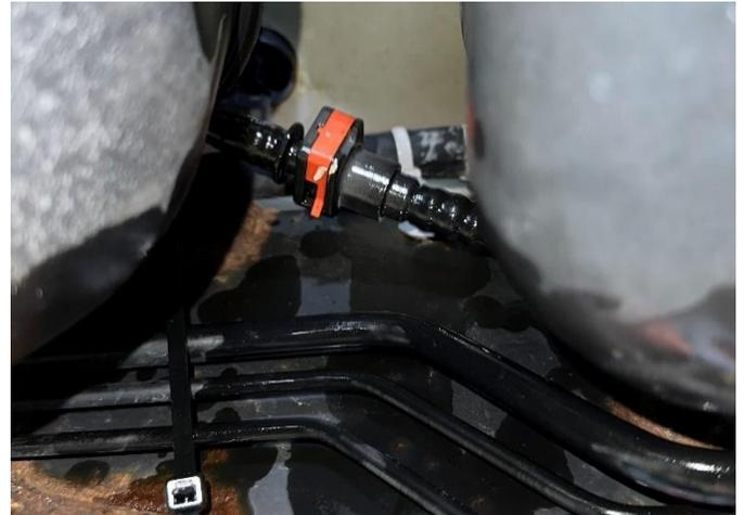
**STEP 5:** Disconnect the red quick disconnect fitting from the fuel filter assembly located on the rear, passenger side of the fuel tank. To disengage the locking tab, spread the two ends of the tab and push the ends toward the center of the fitting. Disconnect the fuel line.
