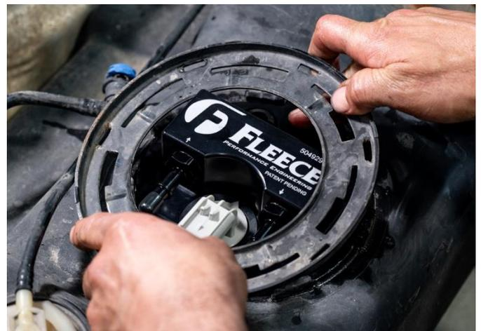
**STEP 15:** Connect the fuel feed and return fittings. Connect the included adapter harness to the connector on the cap of the PowerFlo lift pump.
