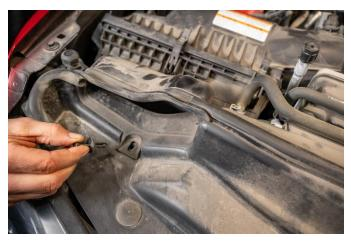
**STEP 12:** Install the intake tube. Connect the tube to the intake manifold first, then tighten the hose clamp. Fasten the retaining clips onto the upper airbox housing. Place the degas line into the clip on the top of the intake tube. Reconnect the MAF sensor connector
