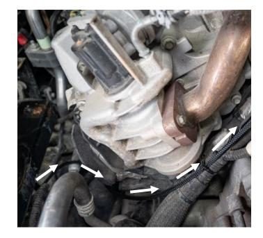
Continue routing the alternator signal harness across the front of the engine bay and along the plastic channel underneath the intake manifold.
