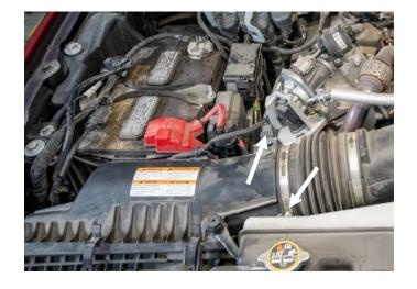
**STEP 3:** Carefully lift the coolant de-gas line to remove it from the clip on the top of the intake tube. Loosen the hose clamp connecting the intake tube to the upper intake manifold. Remove the intake tube and set aside.
