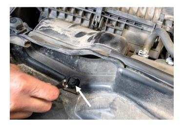
**STEP 5:** Locate the screw retaining the lower airbox assembly to the front core support. Using a 7mm socket or wrench, remove the screw. Gently pull upwards on the lower airbox assembly to remove. A fir tree harness retainer may be present on the underside of the airbox. Carefully remove the retainer from the lower airbox assembly.
