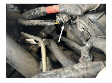
**STEP 7:** Locate the 20-pin PCM harness connector underneath the front facing side of the battery box (circled at right). Disconnect the harness connector by pressing on the release tab and pulling the connector apart.
