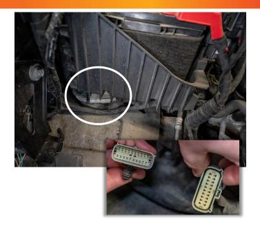
**STEP 8:** Connect the passthrough connector onto both ends of the PCM harness as shown at right. Push the red locking tab into the connector to secure the connection.
