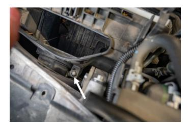
**STEP 6:** Locate the alternator. Disconnect the OE charging circuit harness connector from the rear of the alternator.
