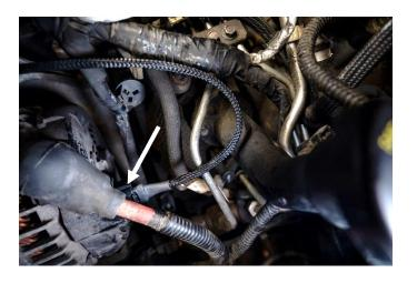
**STEP 12:** Install the lower airbox housing. If present, press the fir tree retainer into the rear of the housing to retain the MAF sensor harness. Using a 7mm socket or wrench, torque the mounting screw to 53 in-lb.
