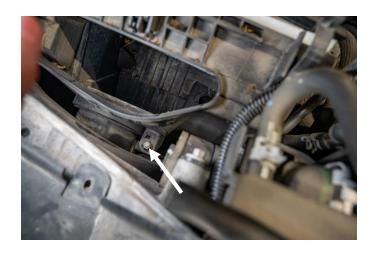
**STEP 13:** Install the airbox inlet onto the lower airbox assembly. Place the plastic pop rivet into the mounting hole as shown at right and press down to fasten.
