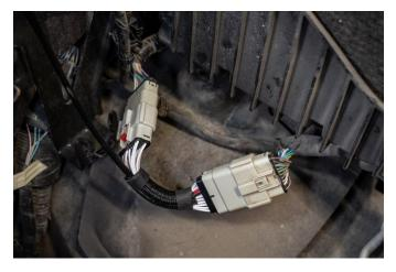
**STEP 9:** Tuck the connector underneath the battery box as shown at right. Route the alternator signal harness wire towards the driver's side of the vehicle.
