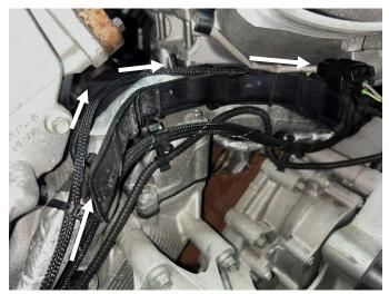
Connect the end of the alternator signal wire harness to the rear of the primary alternator.
