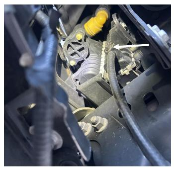
**STEP 3:** Locate the coolant hose routed from the driver's side of the radiator to the thermostat housing. Using a flathead screwdriver or pliers, remove the retaining clip on the coolant elbow as shown in the secondary image at right. Disconnect the elbow and hose from the thermostat housing.
