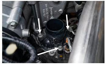
**STEP 7:** Remove the thermostat from the engine. Remove the rubber O-ring from the thermostat.
