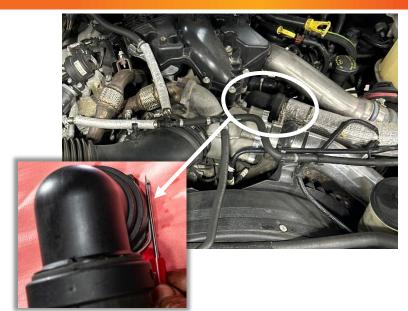
**STEP 4:** Remove the internally mounted O-ring from the coolant elbow removed from the thermostat housing as shown at right.
