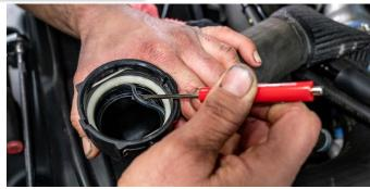
**STEP 5: Lubricate** the included round O-ring in your kit with fresh coolant and install it into the coolant elbow.
