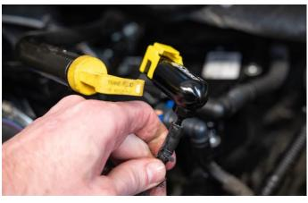
**STEP 7:** Using pliers, move hose clamp upward and position the hose clamp over the fitting.
