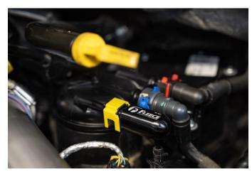
If the fitting requires maintenance, a service kit is available, Fleece Performance P/N: FPE-FMC-FF-RLK-1724-SER. The kit includes replacement O-rings and locking tabs.
