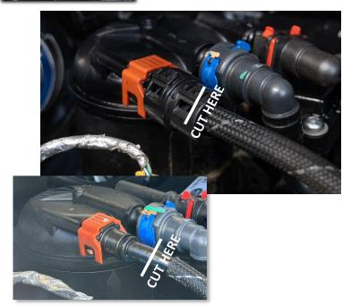
**STEP 4:** Cleanly cut the injector return line.
