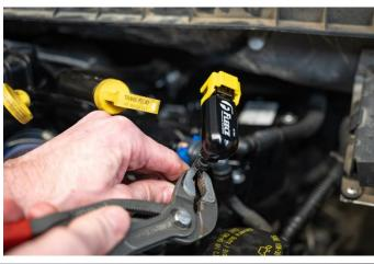
**STEP 8: Lubricate** the injector return line connector on the fuel filter assembly with clean fuel. Ensure the locking tab is lifted to the up position.
