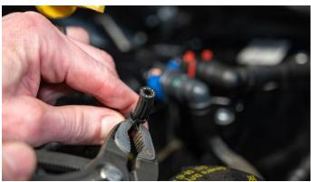
**STEP 6: Lubricate** the hose barb fitting with clean fuel to ease installation into the injector return hose. Press the barb fitting into the hose until both barbs are fully covered by the hose.
