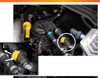
STEP 3: Disconnect the fuel feed fitting (gray plastic release buttons shown) from the filter assembly. Push the fitting towards the filter to release tension on the retainer. Squeeze both of the gray buttons and pull the fitting away from the filter to remove.
