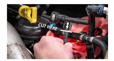
**STEP 5:** With the factory injector return connector removed, install the included hose clamp onto the injector return hose using a pair of pliers. Install the clamp approximately one inch from the end to allow room for the barb fitting to be installed.
