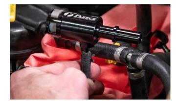
**STEP 8: Lubricate** the inlet connector on the fuel filter assembly with clean fuel. Install the new Fleece Performance fitting onto your fuel filter assembly. Push the fitting towards the filter housing until you feel the locking ring click into place. Pull the fitting away from the filter to confirm it is seated properly.
