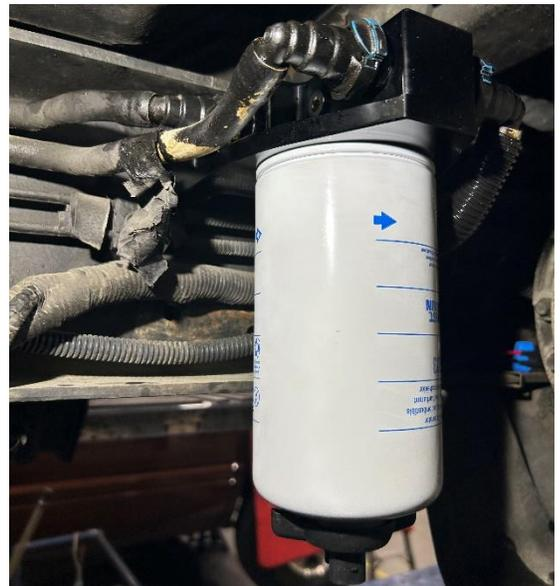
**STEP 21:** Using the included adapter, connect the water in fuel sensor to the electrical harness.
