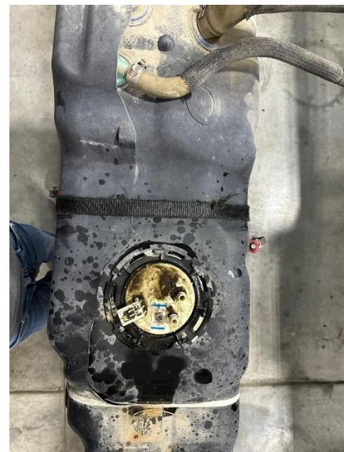
**STEP 9:** Using a hammer and a chisel or punch, remove the locking ring by tapping the ring counterclockwise.
