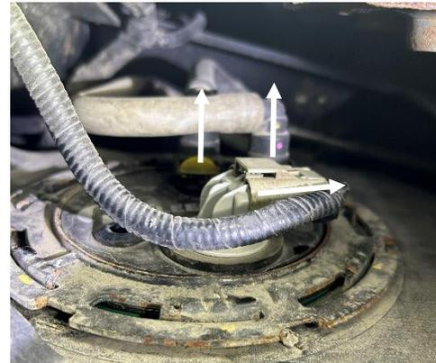
**STEP 7:** Fully lower the tank. You may have to adjust the fuel filler tube and breather to help clear the frame.
