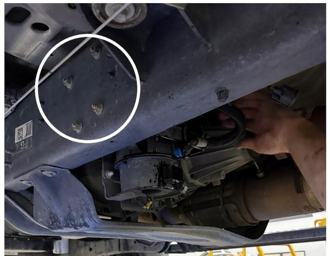
**STEP 16:** Connect the new Powerflo lift pump harness to the OE pump harness that was disconnected from the OE pump assembly. Use zip ties to secure the harness in place.
