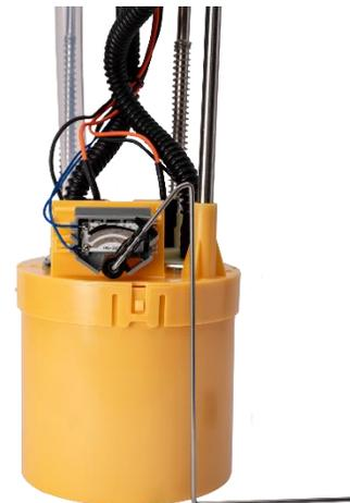
**STEP 12:** Install the new lift pump into the tank in the same orientation as the OE sending unit. Align the pump in its proper orientation before inserting into the tank. Once installed into the tank, **DO NOT** rotate the pump in such a manner that may cause the float arms to hit the sides of the tank. This will cause damage to the float arm. Reinstall the locking ring.
