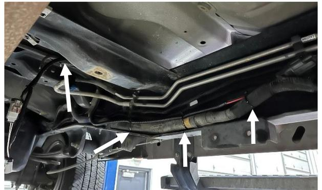
**STEP 18:** Connect the OE sending unit harness to the new PowerFlo harness as shown at right.
