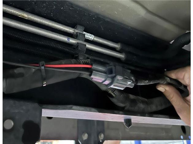
**STEP 17:** Route the new harness along the existing chassis harness on the inside of the frame rail using zip ties in the locations shown at right.
