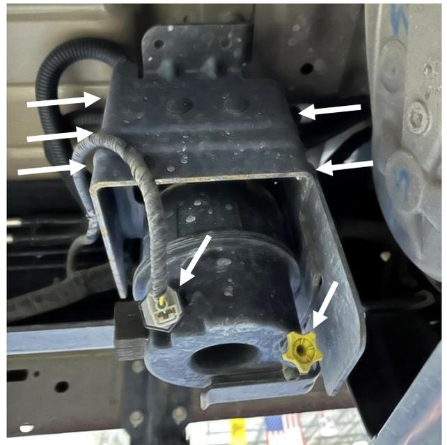
**STEP 14:** Disconnect the two quick disconnect fuel lines on the front facing side of the filter and pump assembly.
