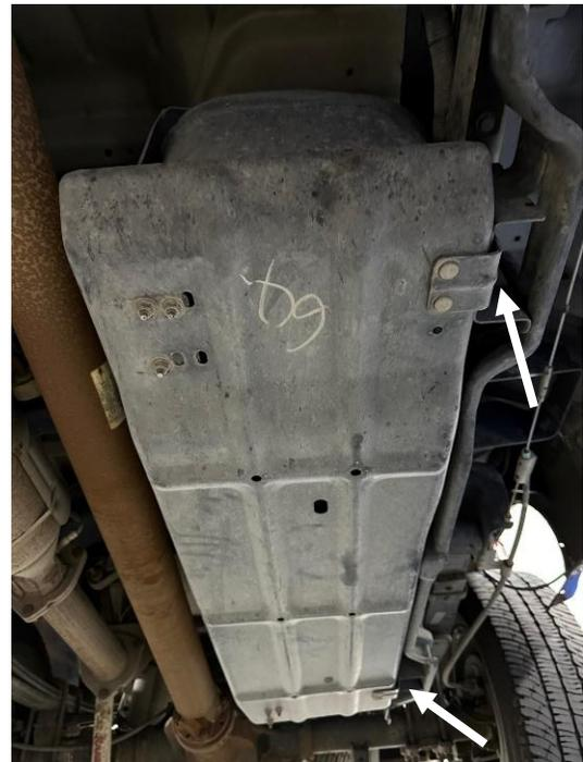
**STEP 5:** Place a transmission jack or floor jack under the fuel tank to lightly support it. Remove the bolts on the tank straps using a 13mm socket or wrench.
