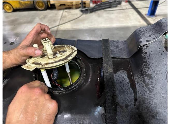
**STEP 11:** Remove the existing o-ring from the tank and replace it with the o-ring included in the kit.
