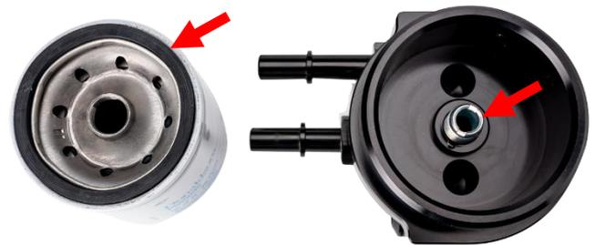
**STEP 5:** Install the new Fleece Performance filter assembly into the filter mounting canister on the engine. Make note of the alignment dowel on the new filter assembly and the locking tab position in the mounting canister. Align the locking tab and rotate the assembly clockwise into the housing.
