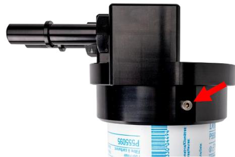
**STEP 6:** Reconnect the fuel line quick disconnect fittings and engage the locking tab on the fuel output hose by pressing the locking tab downward into the connector body. Confirm the connection is secure by gently pulling on each the line to ensure it is secure.
