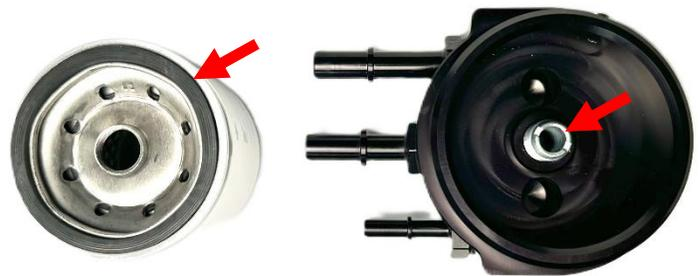
**STEP 5:** Install the new Fleece Performance filter assembly into the filter mounting canister. Make note of the alignment dowel on the new filter assembly and the position in the mounting canister. Align the locking tab and rotate the assembly clockwise into the housing.
