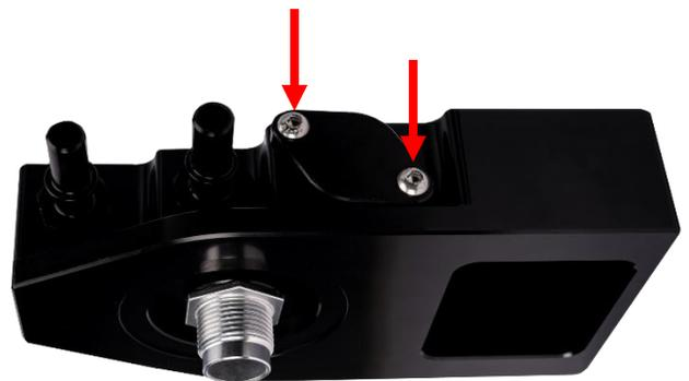
**STEP 3:** Install the fuel heater into the port where the block off plate was removed. Reinstall the screws using a 4mm allen wrench.
