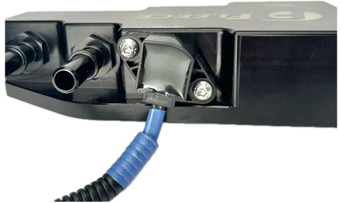
**STEP 4:** Route the fuel heater connector through the rear of the engine bay and down towards the driver's side frame rail. Retain the fuel heater relay to the firewall using either a zip tie or bolt if available.
