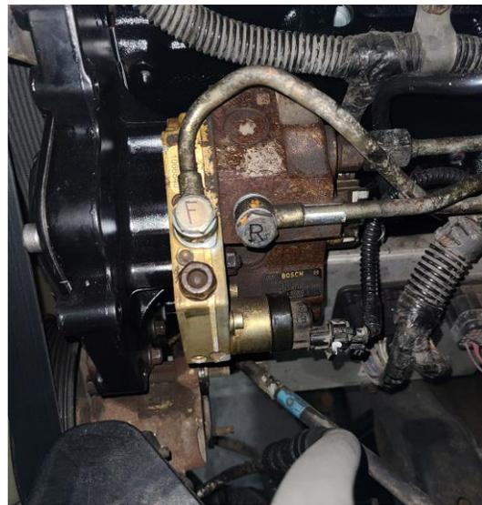
A fully installed 6.7L CP3 is shown at right.
