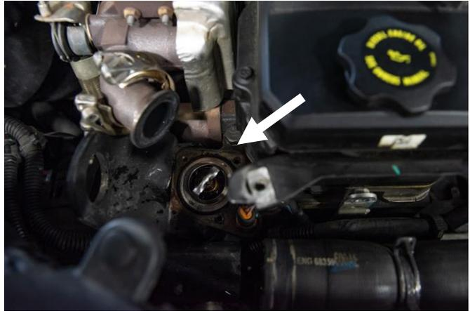
STEP 19: Install the new Fleece coolant bypass elbow into the same location as the factory coolant elbow. Install the three new M6 bolts included in the kit that retain the coolant elbow to the cylinder head. Reinstall the coolant hose and clamp.
