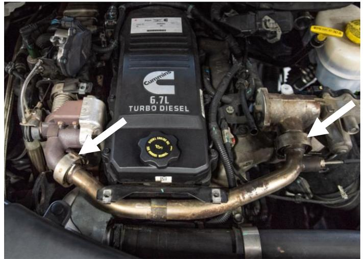
STEP 13: Remove the 8 mm bolt that retains the cross over tube at the front of the engine.
