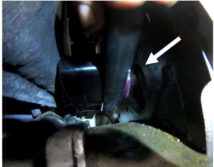
STEP 7: Slide the thermostat housing between the firewall and the back of the engine block. Align the thermostat housing with the original freeze plug hole location and press the housing against the engine to seat the housing. The coolant bypass hose should be oriented towards the passenger side of the vehicle.
