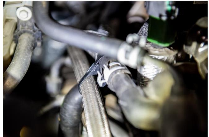
STEP 23: Reinstall the EGR cross over tube. Ensure the new gaskets included with the kit are utilized. Install the V-band clamps and the bolt that retains the cross over tube to the front of the engine.
