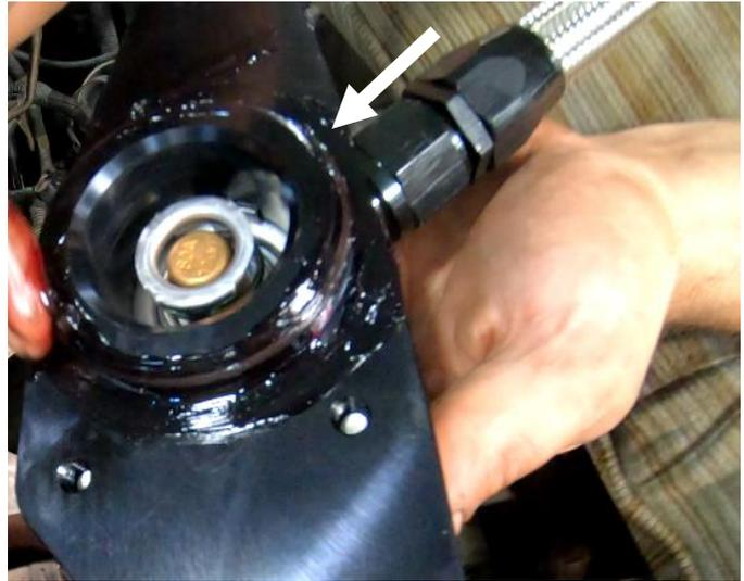
STEP 6: With assembly grease or light oil, thoroughly lubricate the sealing O-ring on the coolant bypass thermostat housing and press it into place on the back of the engine block.
