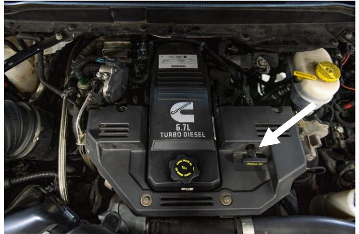
STEP 10: Remove the 4, 8 mm bolts that retain the engine shroud and remove the engine shroud.
