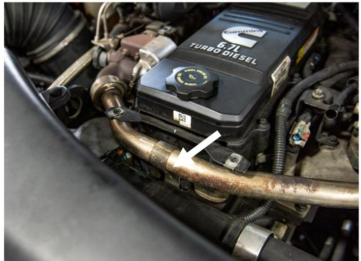
STEP 14: Remove the cross over tube and EGR cross over tube gaskets from each end of the tube. Discard the gaskets, new gaskets are provided in the kit.
