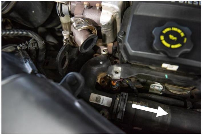
STEP 17: Remove the three, 8mm bolts that retain the cooler elbow to the cylinder head. Remove the cooler elbow. The three bolts will be reused for installation of the Fleece coolant bypass elbow.
