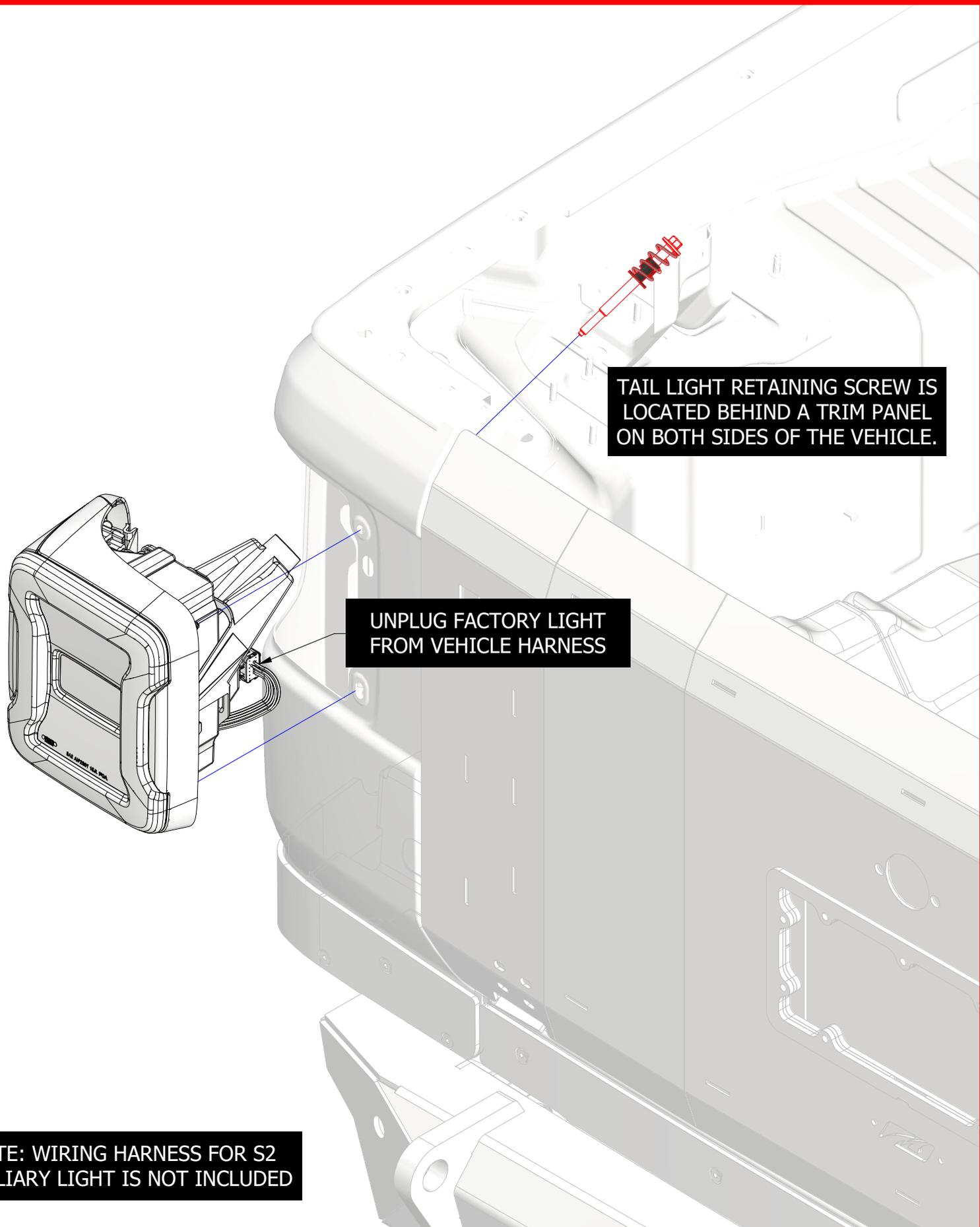
**TAIL LIGHT RETAINING SCREW IS LOCATED BEHIND A TRIM PANEL ON BOTH SIDES OF THE VEHICLE.**
