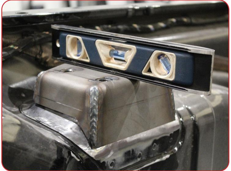
**55** Mark the area at the bottom of MB3032-08 where it meets the tub. Remove the plate and grind the tub down to the bare metal 1/2" above and below the line to prepare for welding.
