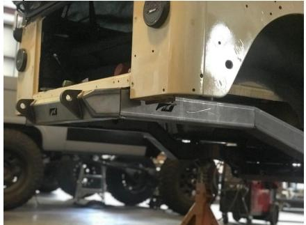
You can clearly see how the frame has moved further up and no longer dips down in the back. This means when we move the rear axle back we will have the necessary room, while allowing us to keep the Jeeps height as low as possible.
