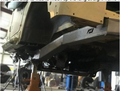
On the inside of the long straight frame rails there is a body mount tab with hole. This lines up with the factory body mount in the middle of the cross member.
