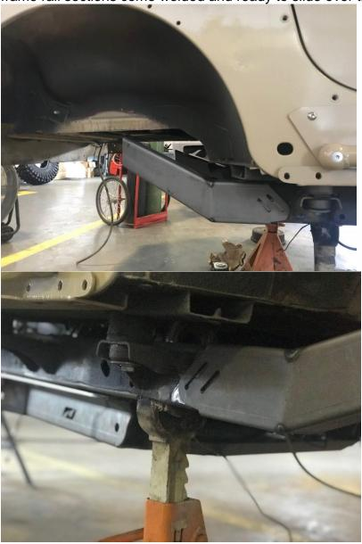
The next step to was to mock up the long straight frame rail sections and rear bumper.
