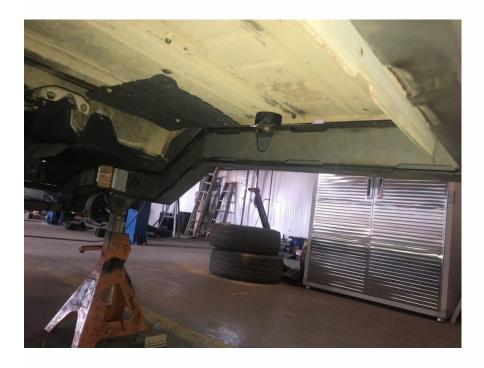
This LJ has a 1.5" body lift so we only had to cut the tub a small amount. You can see where we notched the body just below the tail gate. This kit will work without a body lift but you will need to cut more in this area.
