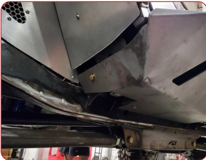
**20** Fasten the front of MB1136-A to MB1136-06 with two 3/8"-16 x 1" hex bolts into the barrel screws installed on MB1136-06
