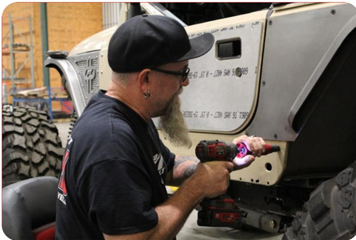
**4** Install two 3/8" rivnuts on each side in the appropriate holes.
