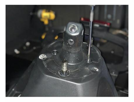
With the screws removed you can separate the camera mount from the wheel studs.
