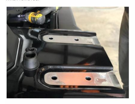
Next un-bolt the factory tire carrier from the tailgate. Disconnect the camera mount wiring.
