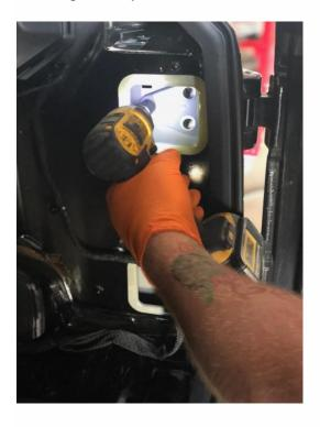
Remove the tailgate and place on your work surface. Remove the 4 tail gate hinge bolts using a #55 torx bit.
