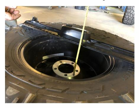
Bolt the tire carrier mount to the main carrier and adjust the mount to be slightly less than the measurement you made with the tire and the flat edge. The reason you want it to be slightly less is so when the tire is bolted to the carrier it applies slight pressure against the carrier. Be sure to torque all the fasteners.
