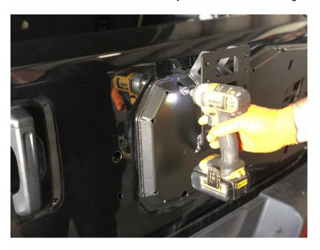
Next the tire carrier mounts can be assembled. Attach using the 6 provided grade 8 bolts. There are multiple positions based on the size of your tire.
