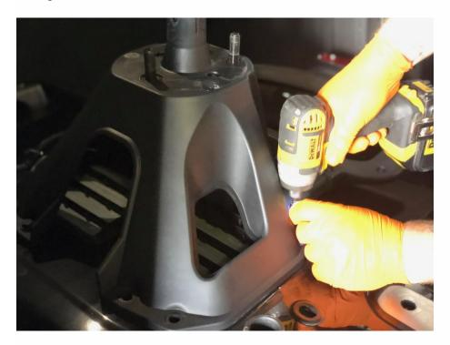
Take this time to clean up the surface of your tail gate. These vents will also be used as the point to pass your tag light wiring through. Be sure to remove the rubber stops also.
