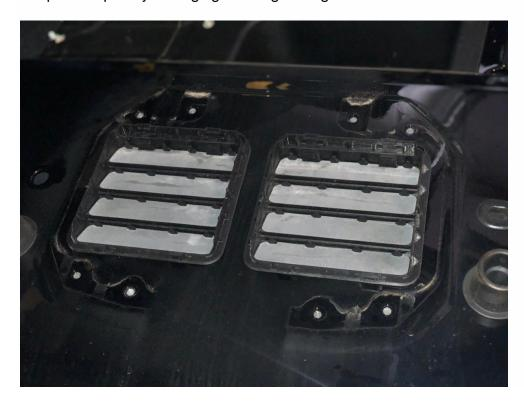
With the tire carrier removed use a torx bit to remove the two screws shown on the camera mount.
