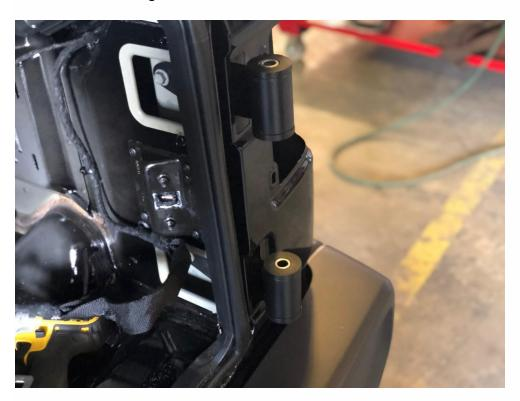
Now place the tire carrier and tail gate assembly onto the hinges and install the greaseable bolts.
