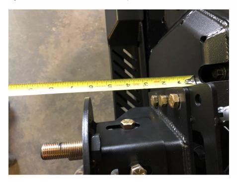
Next you can attach the spare tire and final check your alignment. Depending on the weight of your setup you may need to remove one of the 3 shims.
