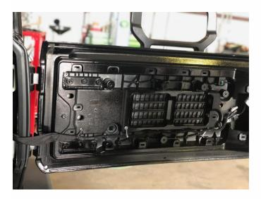
Remove the small plastic panel and use a #45 torx bit to remove the brake light retaining screw. The tail light will need to be removed in order to install the wiring for the MB2115 tag relocation kit and LD-PL6 tag light kit.
