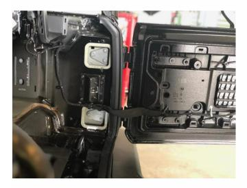
Disconnect the wiring from the tailgate to the tub. Remove the factory tail gate catch as this will no longer be used. We have built in a stop into the tire carrier.
