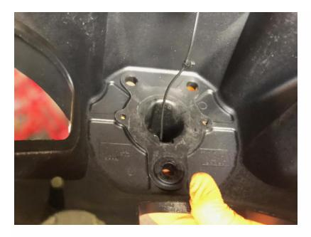
With the camera mount disassembled you can use a torx bit to remove the 3 screws holding the camera to the mount. The new camera/tag mount includes 3 screws that are slightly bigger so the factory camera mount holes will have to be drilled to 1/8 inch.
