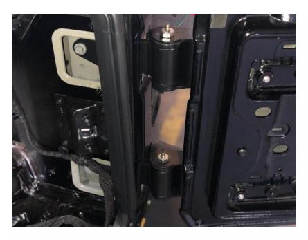
Carefully check the tailgate as you close it for clearance. You may need to make some adjustments before you torque the bolts down. Also, it is typical for the tail gate to sit higher on the driver's side during assembly until the full weight of the tire is installed.
