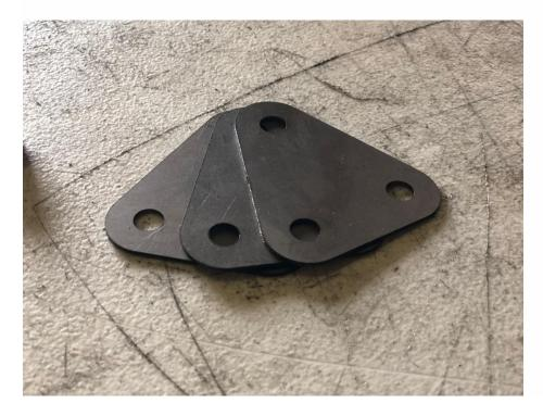
These shims will be placed on the bottom tail gate hinge bracket and bolted between the bracket and the Jeep. A simple trick is to use a dab of axle grease between the shims and the brackets to hold it in place.
