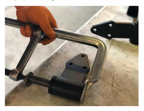
We provide 3 triangular shaped shims to be used on the bottom tailgate hinge. The number of shims used will be dependent on the size and weight of your spare tire.
