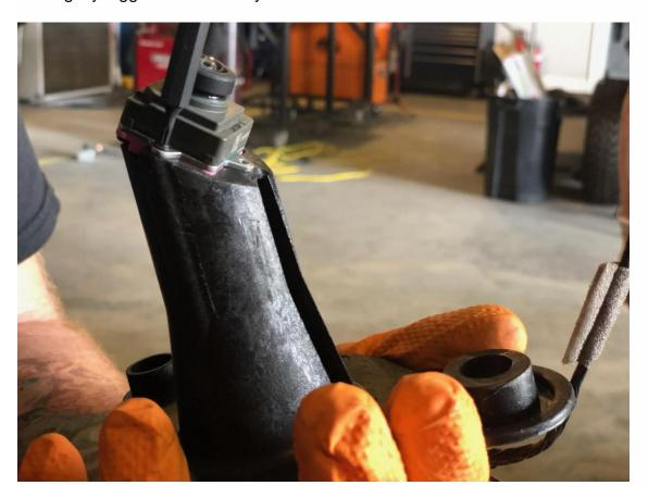
You can disassemble the third brake light assembly to access the end of the wiring or simply cut the wire as we are going to splice it back into our new brake light kit.
