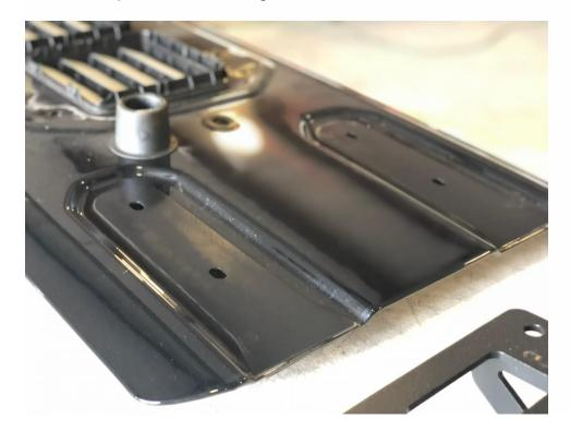
Now place the Motobilt Jeep JL Spare Tire Carrier onto the tailgate. Using the factory bolts lightly install each into the tailgate. Do not tighten them yet as you will need to be able to adjust for alignment.
