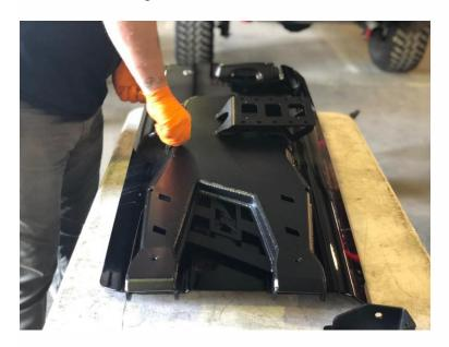
Using the provided bushings install them into the new tail gate hinge brackets along with the metal sleeves.
